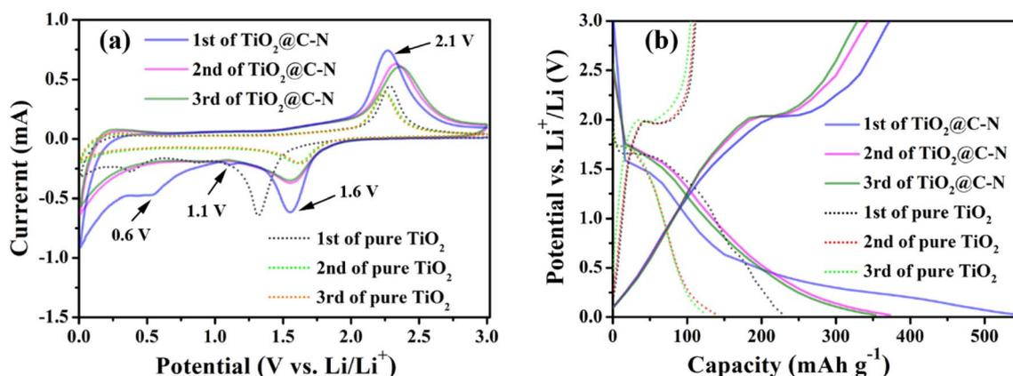
Fig. 6 (a) CV curves of  $\text{TiO}_2@\text{C-N}$  and the pure  $\text{TiO}_2$  precursor; (b) galvanostatic discharge/charge curves of the initial three cycles at  $0.1 \text{ A g}^{-1}$  of  $\text{TiO}_2@\text{C-N}$  and the pure  $\text{TiO}_2$  precursor.
