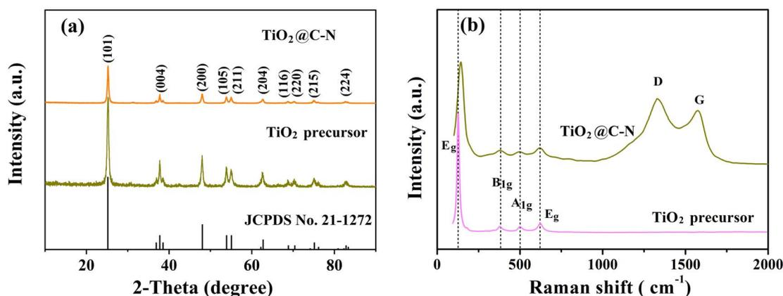
Fig. 2 (a) XRD patterns of the TiO<sub>2</sub> precursor and TiO<sub>2</sub>@C-N; (b) Raman spectra of the TiO<sub>2</sub> precursor and TiO<sub>2</sub>@C-N.
