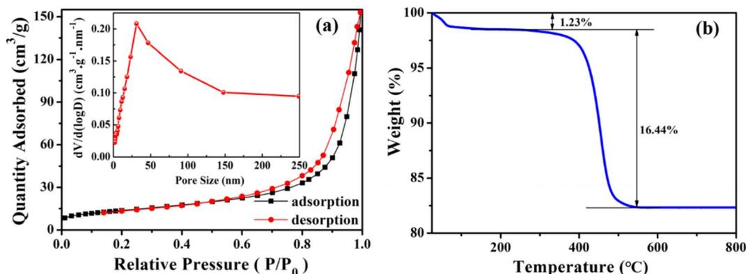
Fig. 4 (a)  $\text{N}_2$  adsorption-desorption isotherms of  $\text{TiO}_2@C-N$ ; inset shows the distribution of pore sizes. (b) TGA plot of  $\text{TiO}_2@C-N$ .
