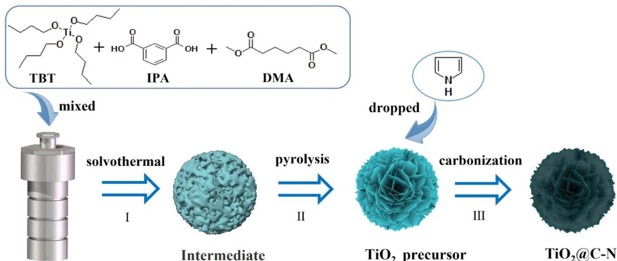
Fig. 1 Schematic of the synthesis process for the TiO<sub>2</sub> precursor and TiO<sub>2</sub>@C-N.
