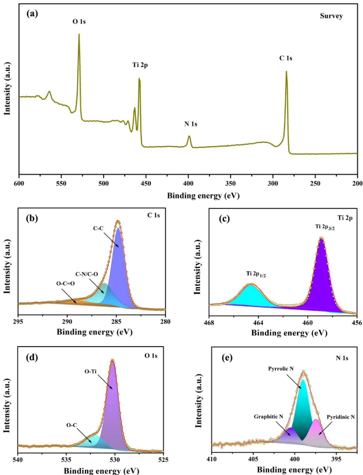
Fig. 5 XPS spectra of TiO<sub>2</sub>@C–N. (a) Survey scan, (b) C 1s, (c) Ti 2p, (d) O 1s, and (e) N 1s.
