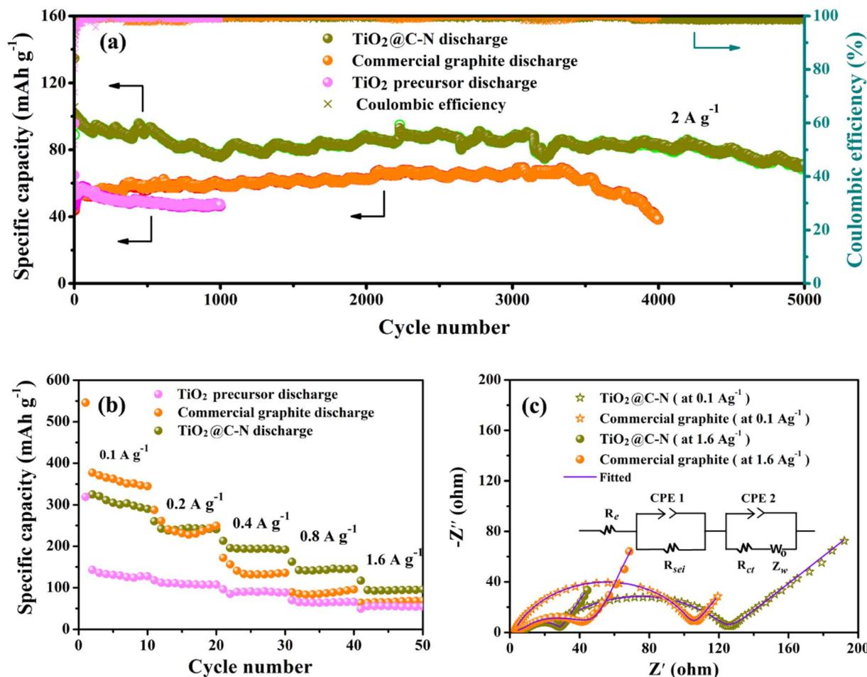
Fig. 7 (a) Long-term cycling performance and coulombic efficiency at 2 A g<sup>-1</sup> of the TiO<sub>2</sub> precursor, TiO<sub>2</sub>@C-N and commercial graphite; (b) rate capabilities of the TiO<sub>2</sub> precursor, TiO<sub>2</sub>@C-N and commercial graphite; (c) experimental and fitted Nyquist plots of commercial graphite and TiO<sub>2</sub>@C-N; inset shows the equivalent circuit model.
