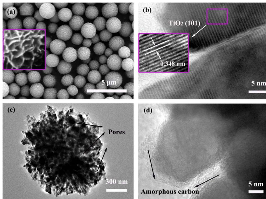
Fig. 3 (a) SEM images of the  $\text{TiO}_2$  precursor; inset shows enlarged image. (b) TEM image of the  $\text{TiO}_2$  precursor; inset shows close-up of the marked area. (c and d) TEM images of  $\text{TiO}_2@C-N$ .
