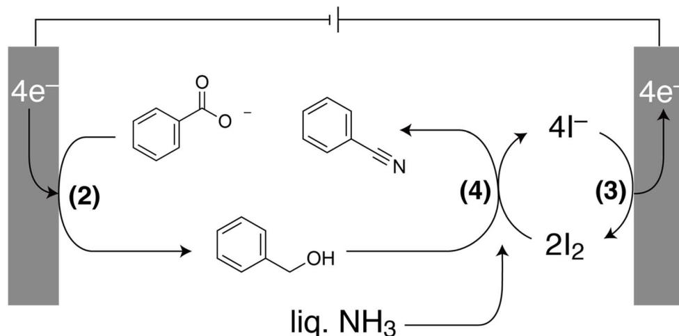
Fig. 3 Schematic of the paired electrocatalysis of benzoic acid in liquid ammonia. Benzoic acid is reduced to benzyl alcohol at the cathode (eqn (2)) and  $I^-$  is oxidized to  $I_2$  at the anode (eqn (3)). Benzyl alcohol and  $I_2$  react with ammonia to produce benzonitrile (eqn (4)).
