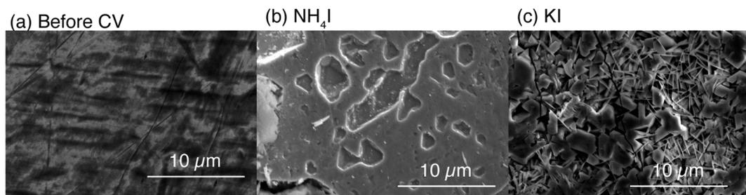
Fig. 6 Surface SEM images of Pb electrodes (a) before CV, and after CV in (b)  $\text{NH}_4\text{I}$  or (c) KI electrolytes. The surface after CV in the  $\text{NH}_4\text{I}$  electrolyte is still smooth, although the roughness is slightly higher than that of the initial surface due to anodic dissolution. In contrast, a porous Pb surface was formed in the KI electrolyte.
