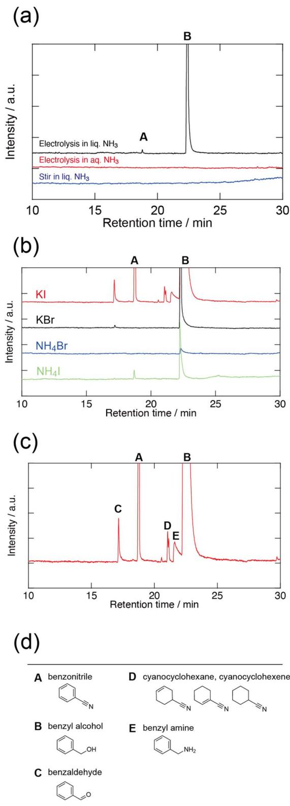
**Fig. 2** (a) GC–MS chromatograms of the products after the electrolysis of 0.1 M benzoic acid + 0.2 M KI in liquid ammonia (black line) and in aqueous ammonia solution (red line). The blue line was obtained using 0.1 M benzoic acid + 0.1 M KI + 0.1 M I<sub>2</sub> in liquid ammonia stirred for 3 h without electrolysis. Benzonitrile and benzyl alcohol were detected only in the electrolysis in liquid ammonia. (b) GC–MS chromatograms of the products after the electrolysis of 0.1 M benzoic acid
