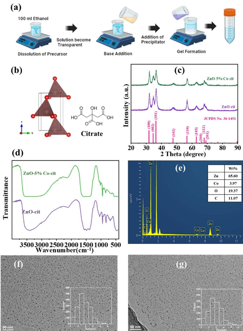
**Fig. 1** Synthesis and spectroscopic characterizations: (a) schematic illustrating the synthetic procedure of ZnO and ZnO-5%Co-cit; (b) crystal structure of ZnO; (c) XRD patterns (d) IR spectra of ZnO and ZnO-5%Co-cit; (e) EDS mapping images of ZnO-5%Co-cit; TEM images of (f) ZnO-cit and (g) ZnO-5%Co-cit.
