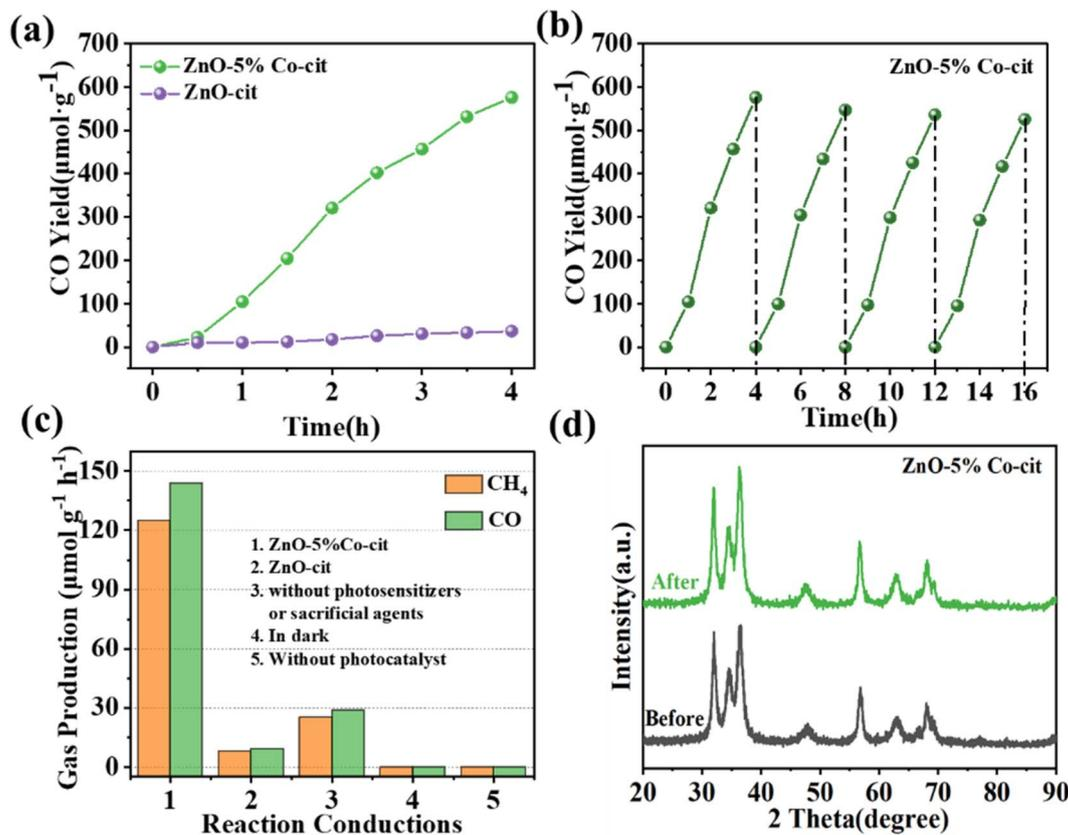
Fig. 2 Photocatalytic performance: (a) photocatalytic CO evolution (light source:300 W Xe lamp,  $\lambda > 420$  nm), (b) Cycling test of ZnO-5%Co-cit for the photocatalytic CO evolution, (c) CH<sub>4</sub> and CO evolution rates under different reaction conductions, (d) XRD patterns of ZnO-5%Co-cit before and after photocatalytic tests.
