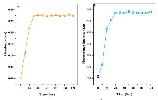
Fig. 3 (a) Response time-absorbance profile of AMMN (5  $\mu$ M) after the addition of Al $^{3+}$  ions (1.0 equiv.) in a DMSO/HEPES (1:9 v/v, pH = 7.4) solution; (b) response time-fluorescence profile of AMMN (5  $\mu$ M) after the addition of Al $^{3+}$  ions (1.0 equiv.) in a buffer solution (1:9 v/v, pH 7.4).
