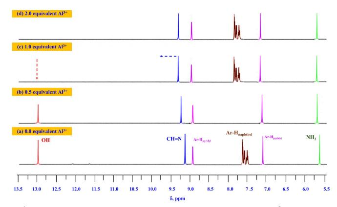
Fig. 11  $^{1}$ H NMR spectra of AMMN (5  $\mu$ M) after addition of (a) 0 equiv.; (b) 0.5 equiv.; (c) 1 equiv. and (d) 2 equiv. of Al<sup>3+</sup> ions.
