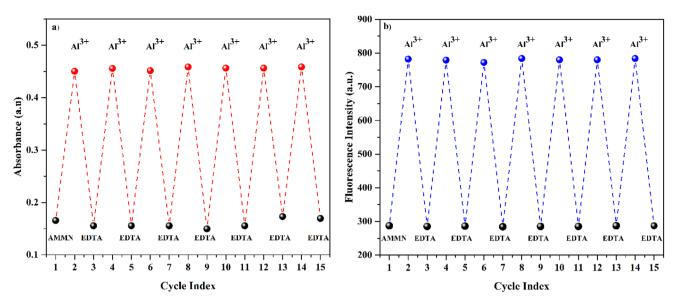
Fig. 8 Reversible changes in (a) absorbance and (b) fluorescence intensity of AMMN after the seguential addition of Al<sup>3+</sup> and Na<sub>2</sub>EDTA.
