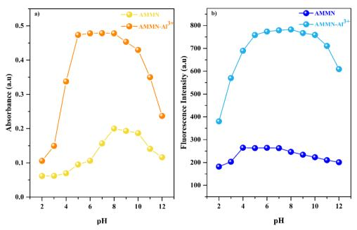
Fig. 2 Impact of pH on AMMN (5  $\mu$ M) (a) absorption intensity in absence and presence of Al<sup>3+</sup> ions; (b) fluorescence intensity in absence and presence of Al<sup>3+</sup> ions.
