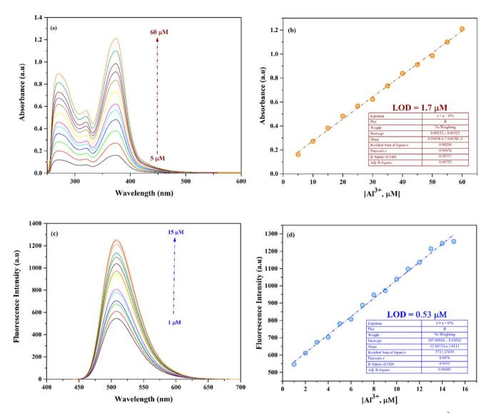
Fig. 5 The spectra and linear relationships between of (a and b) absorbance of AMMN (5  $\mu$ M) at 375 nm after treatment of Al<sup>3+</sup> ions with increasing concentrations from 5–60 mM; (c) and (d) Fluorescence intensity emission of AMMN (1  $\mu$ M) at 503 nm after treatment with increasing Al<sup>3+</sup> concentrations from 1 to 15  $\mu$ M at room temperature.
