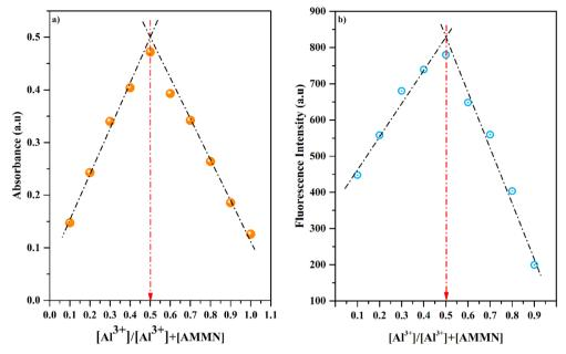
Fig. 4 Job's plot analysis: (a) Absorbance at  $\lambda_{max} = 375$  nm as a function of the mole fraction of the Al<sup>3+</sup> ion ([Al<sup>3+</sup>] = [AMMN] = 20  $\mu$ M); (b) Fluorescence intensity at  $\lambda_{em} = 503$  nm as a function of the mole fraction of the Al<sup>3+</sup> ion ([Al<sup>3+</sup>] = [AMMN] = 5  $\mu$ M).
