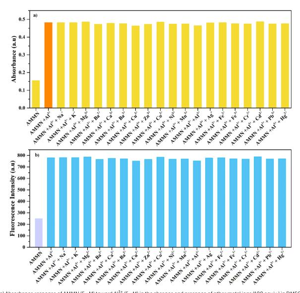
Fig. 7 (a) Absorbance response of AMMN (5  $\mu$ M) toward Al<sup>3+</sup> (5  $\mu$ M) in the absence and presence of other metal ions (100 equiv.) in DMSO/HEPES (1:9 v/v, pH 7.4); (b) Fluorescence response of AMMN (5  $\mu$ M) toward Al<sup>3+</sup> (5  $\mu$ M) in the absence and presence of other metal ions (100 equiv.) in DMSO/HEPES (1:9 v/v, pH 7.4,  $\lambda_{em}$  503 nm).
