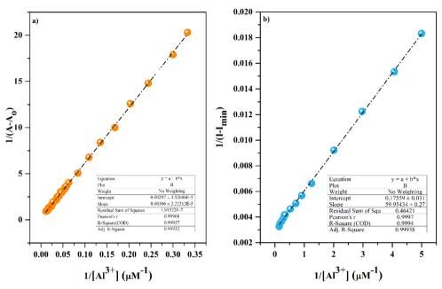
Fig. 6 Benesi-Hildebrand plot analysis of Al<sup>3+</sup> with AMMN from (a) UV-vis spectroscopy; (b) Fluorescence spectroscopy.
