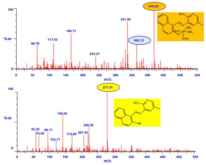
Fig. 10 Positive-ion ESI-mass spectrum of AMMN (50 μM) upon addition of Al<sup>3+</sup> (1.0 equiv.).
