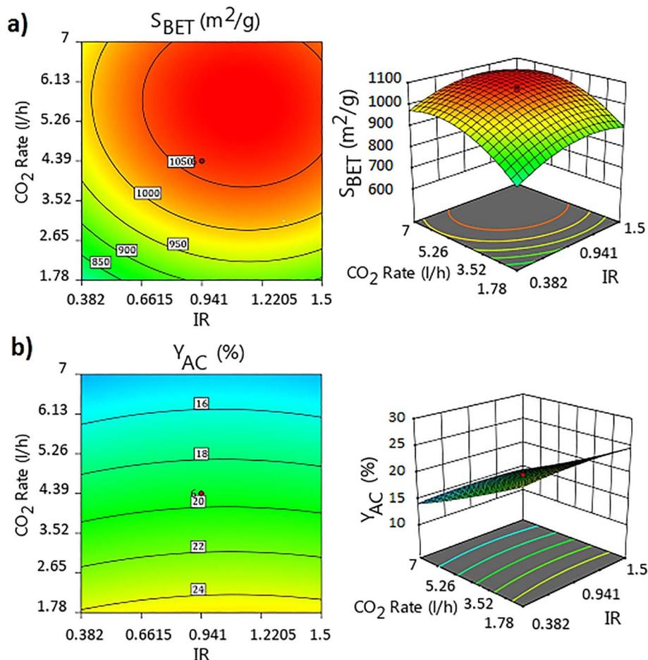
Fig. 10 3D response surfaces and contour plots for effects CO<sub>2</sub> flow rate & IR on (a) S<sub>BET</sub>, (b) Y<sub>AC</sub> at central point of T<sub>act</sub> = 750 °C.
