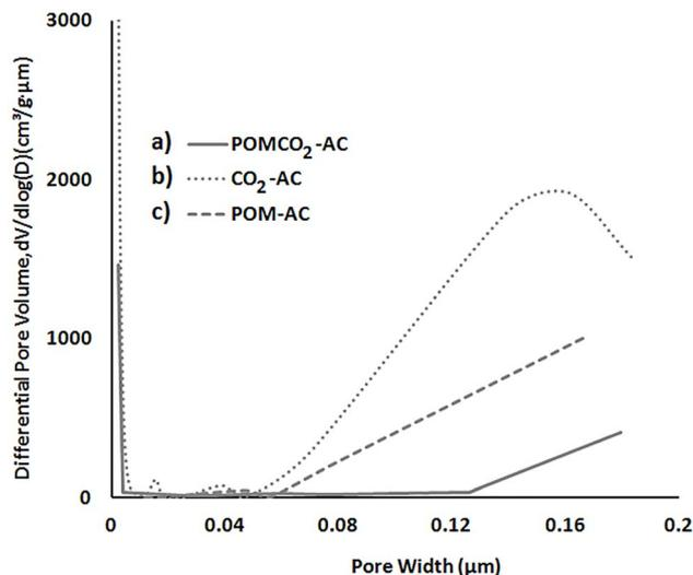
Fig. 4 BJH pore size distribution for the (a) POMCO<sub>2</sub>-AC, (b) CO<sub>2</sub>-AC, (c) POM-AC.
