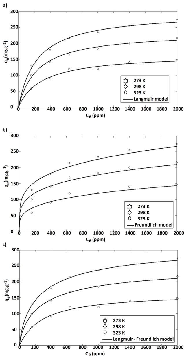
Fig. 11 A comparison of the experimental and predicted adsorption isotherms of DCM on POMCO<sub>2</sub>-AC surface at different temperatures using (a) Langmuir, (b) Freundlich, and (c) Langmuir–Freundlich equations.
