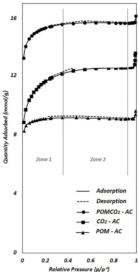
Fig. 3 N<sub>2</sub> adsorption (filled symbols) and desorption (open symbols) isotherms at 77 K for the POMCO<sub>2</sub>-AC (●), CO<sub>2</sub>-AC (■), POM-AC (▲).
