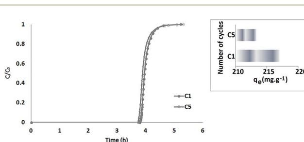
Fig. 14 Breakthrough curve for POMCO<sub>2</sub>-AC under stability test.
