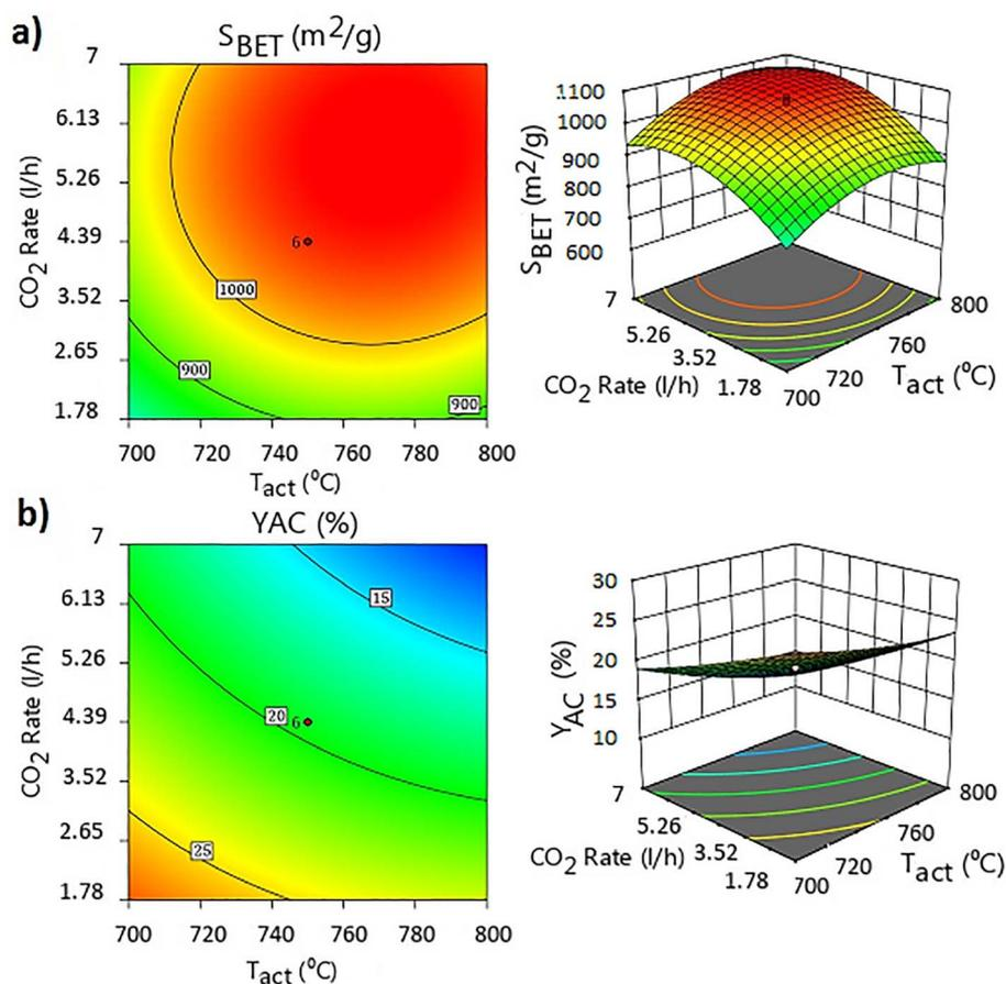
Fig. 9 3D response surfaces and contour plots for effects CO<sub>2</sub> gas flow rate & T<sub>act</sub> on (a) S<sub>BET</sub>, (b) Y<sub>AC</sub> at central point of IR = 0.941 g g<sup>-1</sup>.
