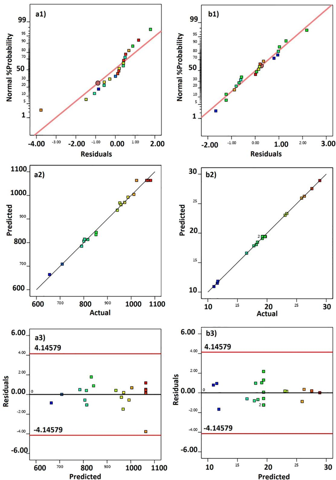
Fig. 7 Assessment of the CCD predictive correlation for (a)  $S_{\text{BET}}$  and (b) Yield (%). 1, 2, and 3 indicate Residual normal probability plot, predicted versus actual values plot, and residual versus predicted response plot, respectively.
