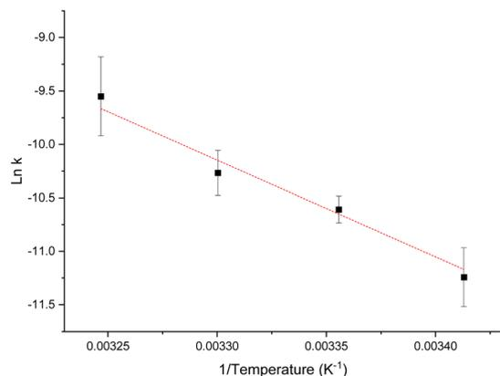
Fig. 4 Arrhenius plot for the determination of the activation energy for the esterification of one alcohol group of Ox063 by pyruvic acid, the slope as determined by the best fit was  $-9053.3$  K. (see Fig. S2 and Table S1 for data points†).
