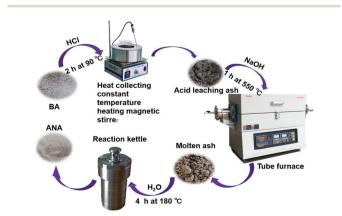
Fig. 1 Flowchart for the synthesis of analcime from BA.
