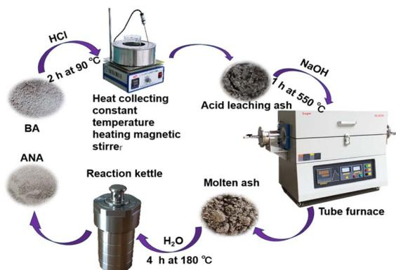
Fig. 1 Flowchart for the synthesis of analcime from BA.
