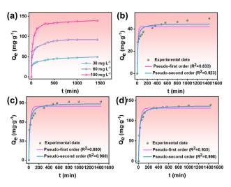
Fig. 6 Effect of concentration on the adsorption (a), pseudo-first-order kinetic model and pseudo-second-order kinetic model of 30 mg  $\rm L^{-1}$  (b) 60 mg  $\rm L^{-1}$  (c) and 100 mg  $\rm L^{-1}$  (d) of TC.
