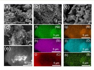
Fig. 3 SEM images of BA (a), acid-leached ash (b), molten ash (c) and ANA (d and e) and EDS elemental mapping of ANA (f-k).
