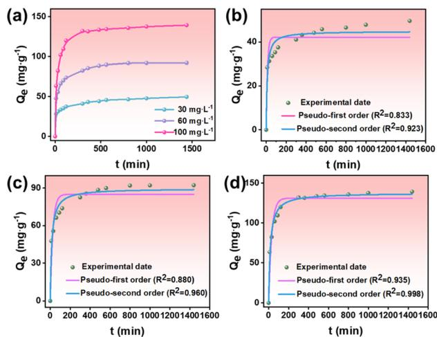
Fig. 6 Effect of concentration on the adsorption (a), pseudo-first-order kinetic model and pseudo-second-order kinetic model of 30 mg L<sup>-1</sup> (b) 60 mg L<sup>-1</sup> (c) and 100 mg L<sup>-1</sup> (d) of TC.
