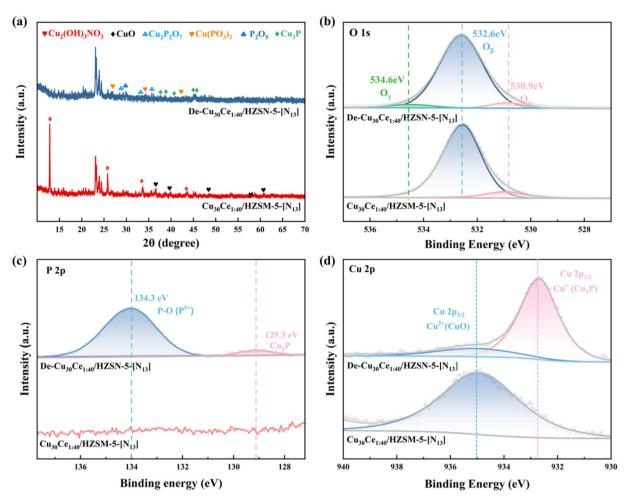
Fig. 9 (a) XRD patterns and XPS results of (b) O 1s spectra, (c) P 2p spectra, and (d) Cu 2p spectra of fresh and used  $Cu_{30}Ce_{1:40}/HZSM-5-[N_{13}]$  adsorbents
