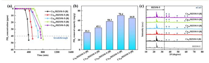
Fig. 2 Effect of different Cu loading amounts on PH<sub>3</sub> removal performance; (a) PH<sub>3</sub> breakthrough curve; (b) adsorption capacity; (c) XRD patterns (adsorption conditions: PH<sub>3</sub> (100 ppm)/N<sub>2</sub>, temperature (30 °C), gas inlet flow rate (24 000 mL min<sup>-1</sup>)).
