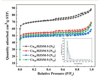
Fig. 5  $N_2$  adsorption/desorption isotherms of different types of adsorbents.
