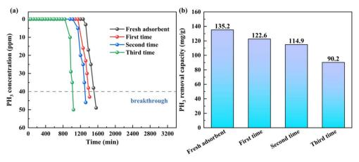
Fig. 10 Effect of regeneration times on PH<sub>3</sub> removal performance: (a) PH<sub>3</sub> breakthrough curve and (b) PH<sub>3</sub> breakthrough adsorption capacity.
