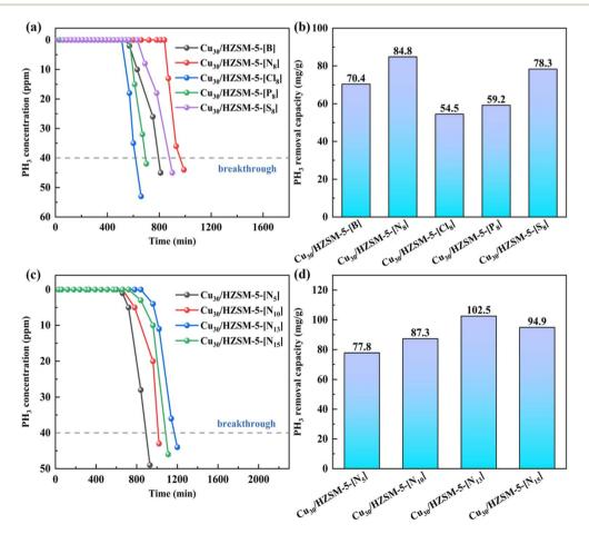
Fig. 3 PH3 breakthrough curves and adsorption capacities of adsorbents with different acid types (a and b) and different hydrogen nitrate impregnation concentrations (c and d) (adsorption conditions: PH<sub>3</sub> (100 ppm)/N<sub>2</sub>, temperature (30 °C), gas inlet flow rate (24 000 mL min<sup>-1</sup>)).
