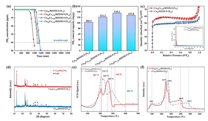
Fig. 6 Effect of different Ce doping concentrations on PH<sub>3</sub> removal: (a) breakthrough curves for PH<sub>3</sub>, (b) PH<sub>3</sub> capacity, (c) BET patterns, (d) XRD patterns, (e) H<sub>2</sub>-TPR profiles, and (f) NH<sub>3</sub>-TPD curves of the materials before and after Ce incorporation (adsorption conditions: PH<sub>3</sub> (100 ppm)/N<sub>2</sub>, temperature (30 °C), gas inlet flow rate (24 000 mL min<sup>-1</sup>)).
