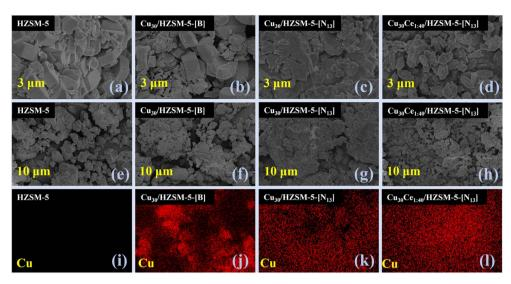
Fig. 7 (a-h) SEM micrographs; (i-l) EDS mapping images of HZSM-5,  $Cu_{30}/HZSM-5-[B]$ ,  $Cu_{30}/HZSM-5-[N_{13}]$ , and  $Cu_{30}Ce_{1:40}/HZSM-5-[N_{13}]$  showing the elemental distribution of Cu.
