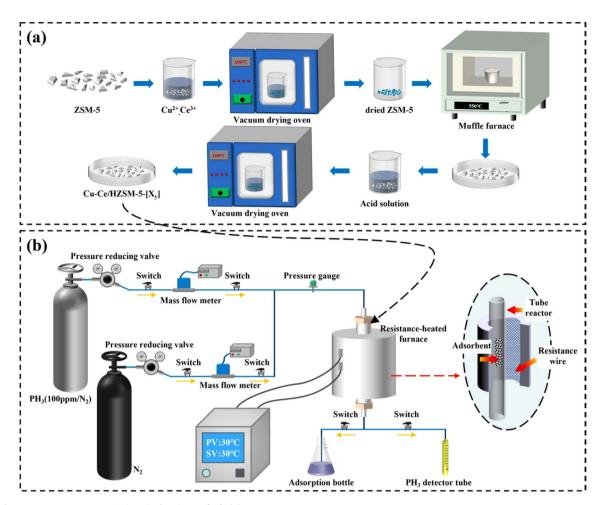
(a) Preparation process of Cu-Ce/HZSM-5-[X<sub>v</sub>]; (b) adsorption-oxidation performance test device
