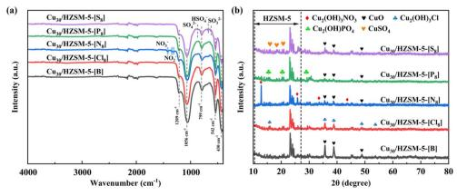
Fig. 4 (a) FT-IR spectroscopy, and (b) XRD profiles for different adsorbent materials.
