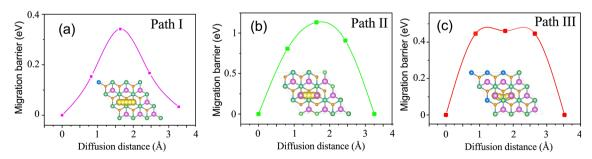
The calculated barrier energy and corresponding pathways for Na-ion migration of (a) Na/TaS2/GeC, (b) TaS2/Na/GeC and (c) TaS2/GeC/ Na.
