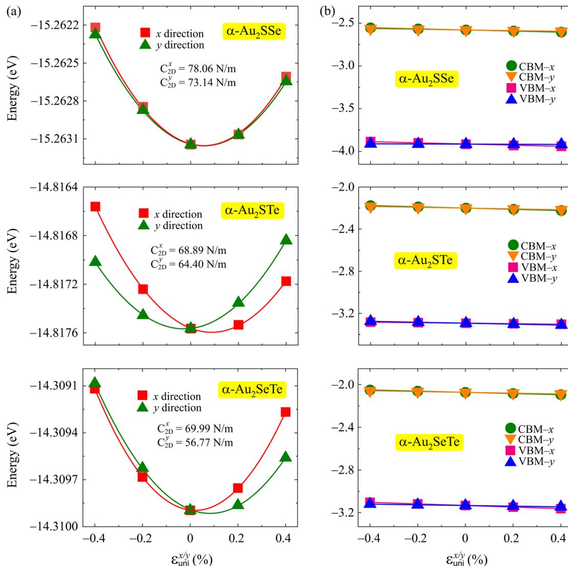
Fig. 6 (a) The shifting of the total energies and (b) CBM/VBM positions with the uniaxial strain of  $\alpha$ -Au<sub>2</sub>XY systems along the two in-plane axes. The solid lines are fitting curves.
