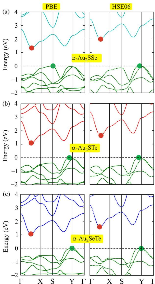
Fig. 4 Electronic band structures from PBE and HSE06 approaches of (a)  $\alpha$ -Au<sub>2</sub>SSe, (b)  $\alpha$ -Au<sub>2</sub>STe, and (c)  $\alpha$ -Au<sub>2</sub>SeTe systems.
