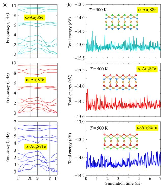
Fig. 2 Phonon spectra (a) and simulation time-dependence of the total energy from AIMD calculation at 500 K of Janus  $\alpha$ -Au<sub>2</sub>XY monolayers. Insets in (b) correspond to the  $\alpha$ -Au<sub>2</sub>XY lattices after the AIMD simulation.
