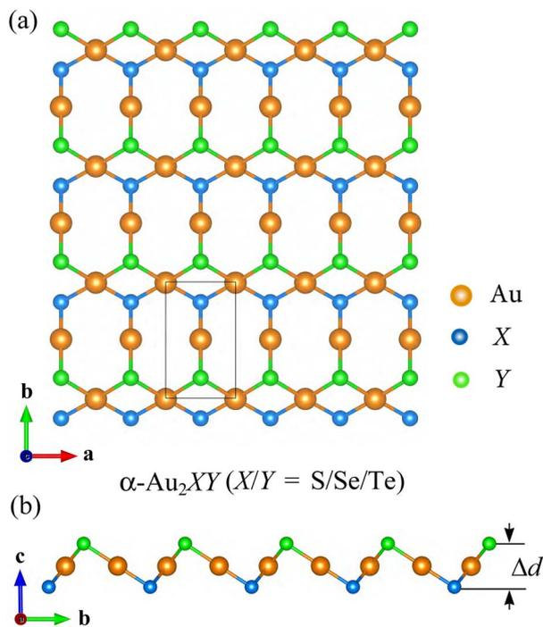
Fig. 1 Crystal structure of  $\alpha$ -Au<sub>2</sub>XY systems with top (a) and side (b) views.
