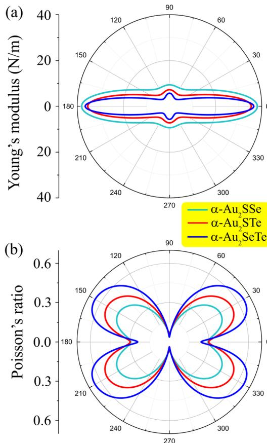
Fig. 3 (a) Young's modulus and (b) Poisson's ratio diagrams as a function of the in-plane angle  $\theta$  of  $\alpha$ -Au<sub>2</sub>XY monolayers.
