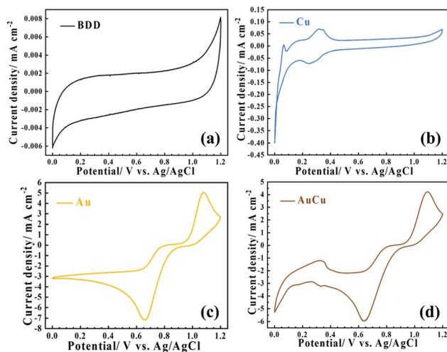
Fig. 2 (a) Baseline CV of a pristine BDD electrode in 0.5 M  $\text{H}_2\text{SO}_4$ . (b) Cu deposition behavior in 20 mM  $\text{CuSO}_4$  + 0.5 M  $\text{H}_2\text{SO}_4$ . (c) Au deposition profile in 20 mM  $\text{KAuCl}_4$  + 0.5 M  $\text{H}_2\text{SO}_4$ . (d) Co-deposition characteristics of Au-Cu alloy in 10 mM  $\text{CuSO}_4$  + 10 mM  $\text{KAuCl}_4$  + 0.5 M  $\text{H}_2\text{SO}_4$ .
