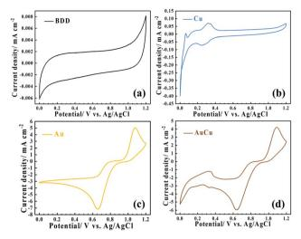
Fig. 2 (a) Baseline CV of a pristine BDD electrode in  $0.5 \text{ M H}_2\text{SO}_4$ . (b) Cu deposition behavior in 20 mM CuSO<sub>4</sub> +  $0.5 \text{ M H}_2\text{SO}_4$ . (c) Au deposition profile in 20 mM KAuCl<sub>4</sub> +  $0.5 \text{ M H}_2\text{SO}_4$ . (d) Co-deposition characteristics of Au–Cu alloy in 10 mM CuSO<sub>4</sub> + 10 mM KAuCl<sub>4</sub> +  $0.5 \text{ M H}_2\text{SO}_4$ .
