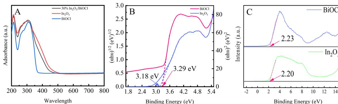
Fig. 12 (A) UV-vis DRS spectra of ( $\text{BiOCl}$ ,  $\text{In}_2\text{O}_3$ , and 30%  $\text{In}_2\text{O}_3/\text{BiOCl}$ ); (B)  $(\alpha h\nu)^{n/2}$  vs. photon energy ( $h\nu$ ) diagrams of ( $\text{BiOCl}$ ,  $\text{In}_2\text{O}_3$ ); (C) VB-XPS diagrams of ( $\text{BiOCl}$ ,  $\text{In}_2\text{O}_3$ ).
