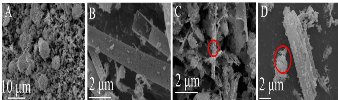
Fig. 2 SEM images of the photocatalyst. (A) BiOCl; (B) In<sub>2</sub>O<sub>3</sub>; (C and D) 30% In<sub>2</sub>O<sub>3</sub>/BiOCl.
