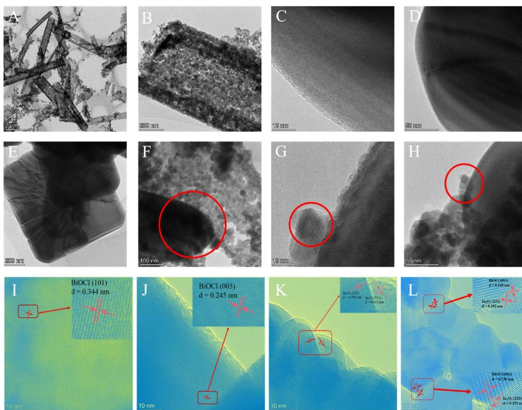
Fig. 3 TEM (A–H) and HRTEM (I–L) images of the photocatalyst. (A, B, and K) In<sub>2</sub>O<sub>3</sub>; (C–E, I and J) BiOCl; (F–H and L) 30% In<sub>2</sub>O<sub>3</sub>/BiOCl.
