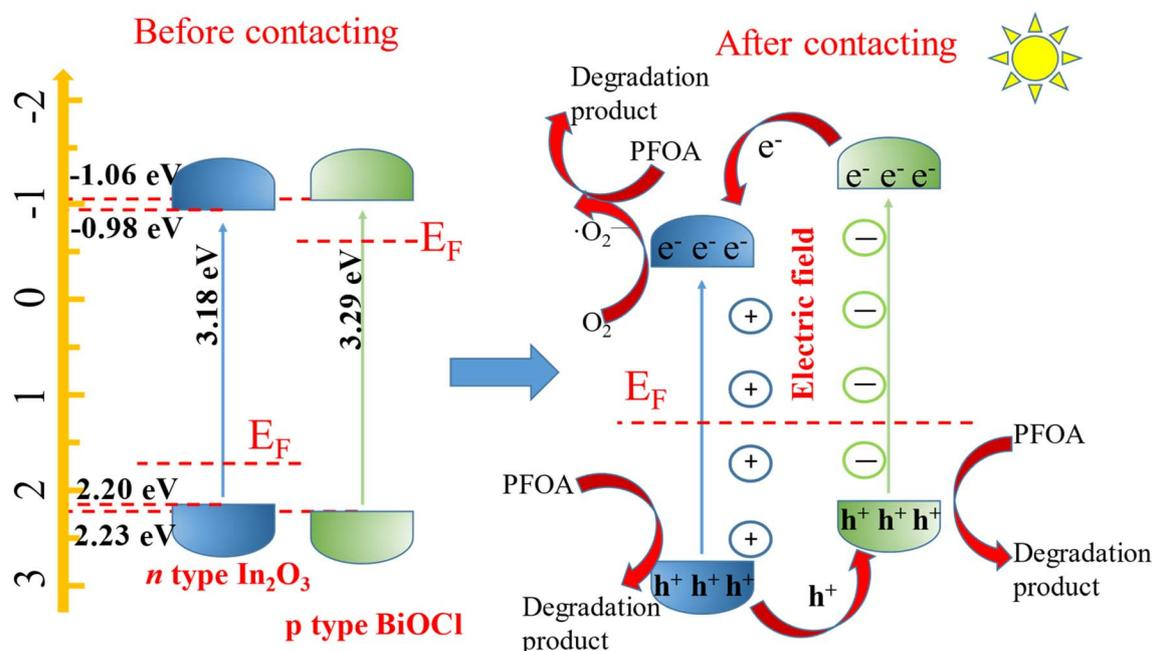
Fig. 13 Banded structure of the In<sub>2</sub>O<sub>3</sub>/BiOCl heterojunction.
