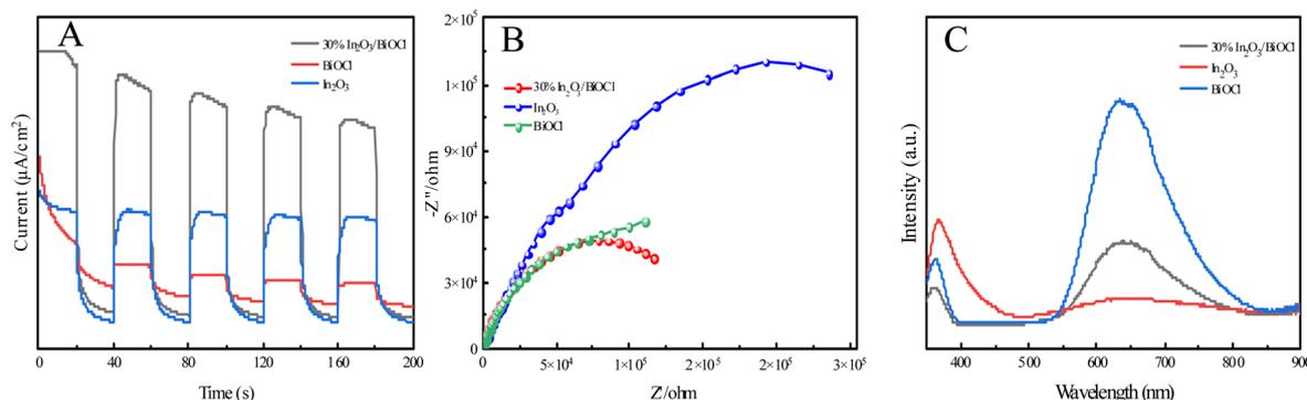
Fig. 14 (A)  $I-t$  spectra of (BiOCl,  $\text{In}_2\text{O}_3$ , and 30%  $\text{In}_2\text{O}_3/\text{BiOCl}$ ); (B) EIS diagrams of (BiOCl,  $\text{In}_2\text{O}_3$ , 30%  $\text{In}_2\text{O}_3/\text{BiOCl}$ ); (C) PL spectra of (BiOCl,  $\text{In}_2\text{O}_3$ , 30%  $\text{In}_2\text{O}_3/\text{BiOCl}$ ).
