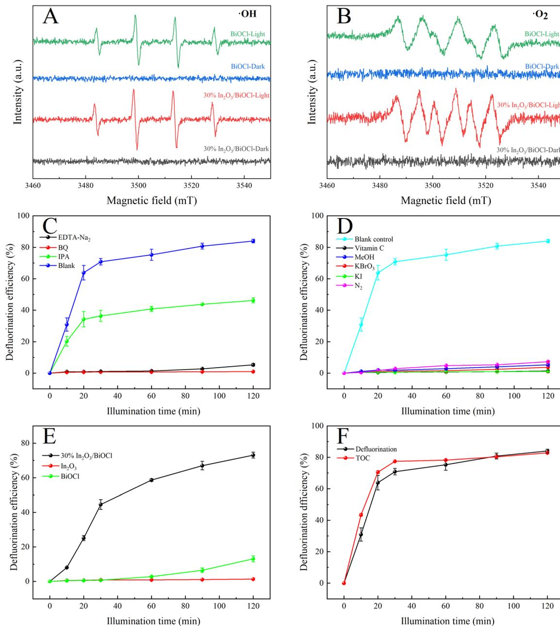
**Fig. 11** (A and B) ESR spectra of  $\cdot\text{OH}$  and  $\cdot\text{O}_2^-$  of BiOCl and 30% In<sub>2</sub>O<sub>3</sub>/BiOCl. (C) Free radical capture experiment. (D) Control experiment of  $\cdot\text{O}_2^-$  inhibition and  $\text{h}^+$  generation. (E) Degradation efficiency of different photocatalysts on PFOA under a 360 nm filter. (F) TOC removal rate of PFOA.
