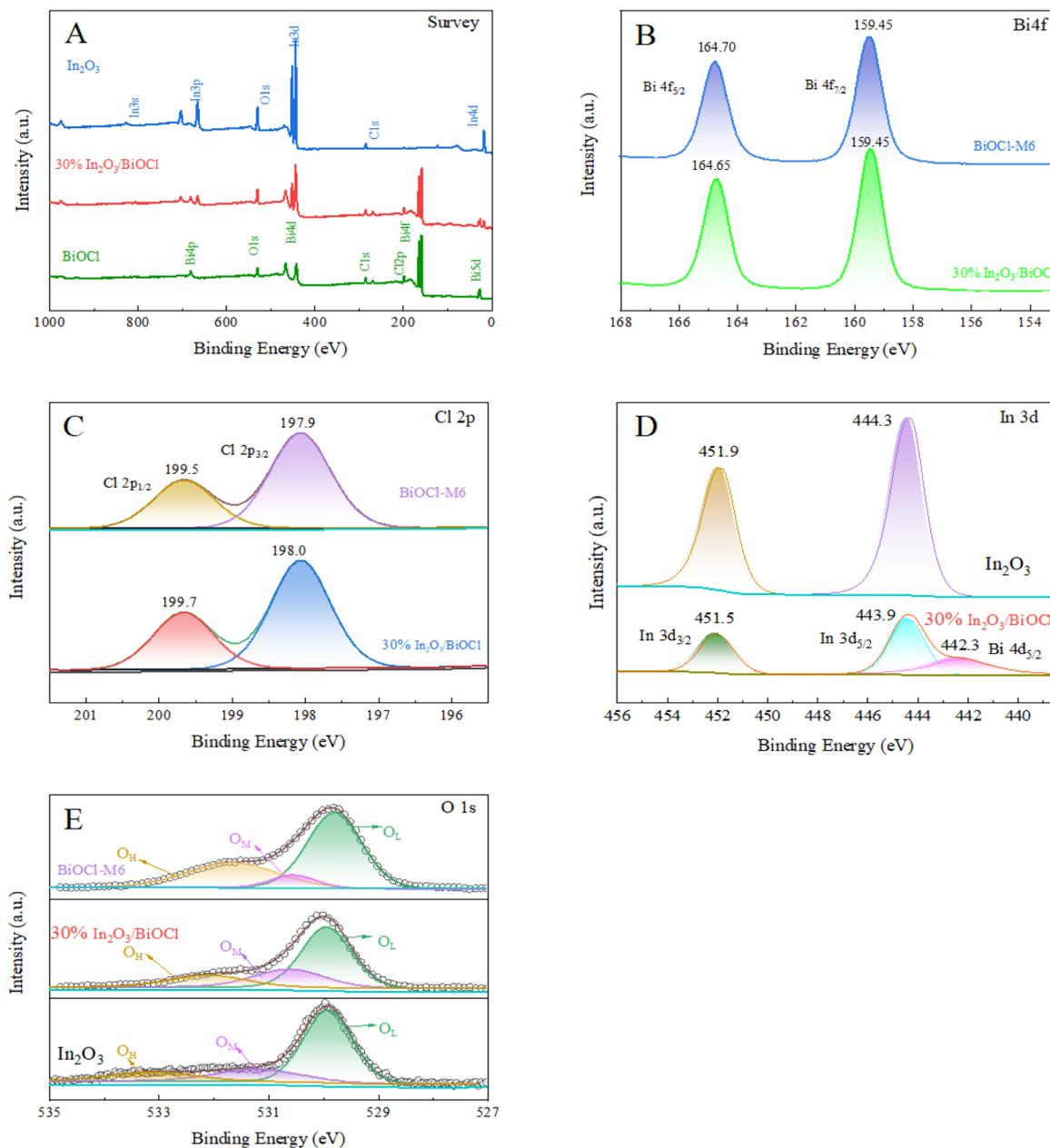
Fig. 5 XPS spectra of the photocatalysts. (A) XPS spectra of BiOCl, In<sub>2</sub>O<sub>3</sub>, and 30% In<sub>2</sub>O<sub>3</sub>/BiOCl; (B) Bi 4f spectra of BiOCl and 30% In<sub>2</sub>O<sub>3</sub>/BiOCl; (C) Cl 2p spectra of BiOCl and 30% In<sub>2</sub>O<sub>3</sub>/BiOCl; (D) In 3d spectra of In<sub>2</sub>O<sub>3</sub> and 30% In<sub>2</sub>O<sub>3</sub>/BiOCl; and (E) O 1s spectra of BiOCl, In<sub>2</sub>O<sub>3</sub>, and 30% In<sub>2</sub>O<sub>3</sub>/BiOCl.
