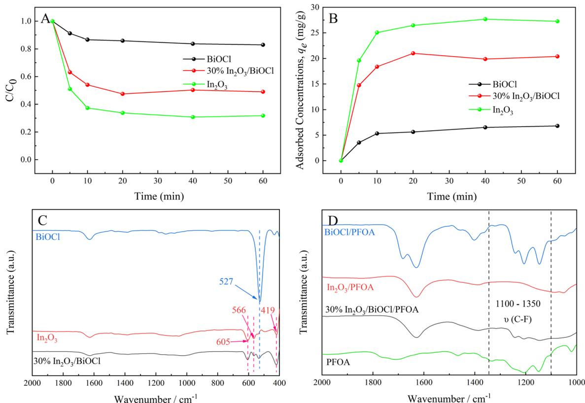
Fig. 6 Adsorption curve and FT-IR spectra. (A) Adsorption curve of different photocatalysts. (B) Adsorption volume change curve. (C) FT-IR spectra of BiOCl, In<sub>2</sub>O<sub>3</sub>, and 30% In<sub>2</sub>O<sub>3</sub>/BiOCl. (D) FT-IR spectra of BiOCl/PFOA, In<sub>2</sub>O<sub>3</sub>/PFOA, and 30% In<sub>2</sub>O<sub>3</sub>/BiOCl/PFOA.
