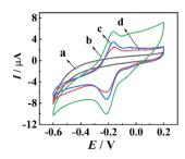
Fig. 5 Cyclic voltammogram of the electrode during the modification process, (a) bare gold electrode, (b) (GO/thionine/AuNPs)/Au. (c) L-Phe/(GO/thionine/AuNPs)/Au. (d) p-Phe/(GO/thionine/AuNPs)/Au.
