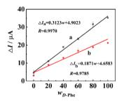
Fig. 12 Current changes in the reaction of (GO/Thi/AuNPs)/Au with a series of solutions in which  $\rm p-$  and  $\rm L-$ Phe are mixed in different ratios. The concentrations of Phe were: (a) 8 mmol  $\rm L^{-1}$  and (b) 2 mmol  $\rm L^{-1}$ .
