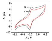
Fig. 6 CV of gold electrodes modified with different modifying materials. (a) Thi/AuNPs/Au, (b) (GO/Thi/AuNPs)/Au
