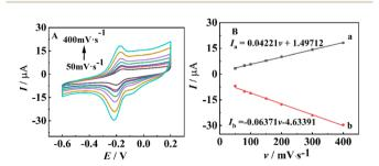
Fig. 7 Cyclic voltammograms obtained from the GO/thionine/AuNPs hybrids modified electrode with L-Phe at different scan rates in a a testing base solution containing 0.1 mol per L NaAc-HAc (A). Linear relationship between the oxidation (a)/reduction (b) peak current values and the scan rates (B).
