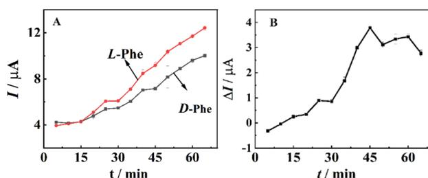
Fig. 10 The relationship of reaction time between modified electrode and D/L-Phe (A). Dependence of  $\Delta I$  on incubation time (B).
