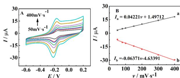
Fig. 7 Cyclic voltammograms obtained from the GO/thionine/AuNPs hybrids modified electrode with *L*-Phe at different scan rates in a testing base solution containing 0.1 mol per L NaAc-HAc (A). Linear relationship between the oxidation (a)/reduction (b) peak current values and the scan rates (B).
