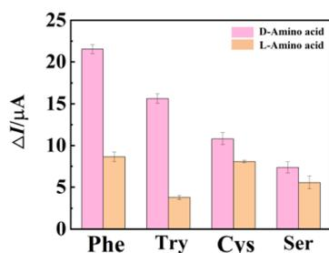
Fig. 13 Chiral sensor recognition of four amino acids.
