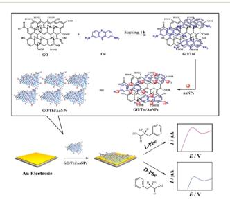
Scheme 2 Schematic illustration of preparation process of the immunosensor.
