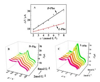
Fig. 11 Relationship diagram between peak current difference and D/L-Phe concentration (A). CV intensity of the biosensor in gradually enhanced D-Phe (B) and L-Phe (C) concentration (2 to 8 mmol  $L^{-1}$ ).
