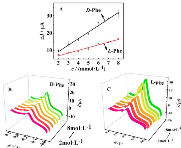
Fig. 11 Relationship diagram between peak current difference and D/L-Phe concentration (A). CV intensity of the biosensor in gradually enhanced D-Phe (B) and L-Phe (C) concentration (2 to 8  $\text{mmol}\cdot\text{L}^{-1}$ ).
