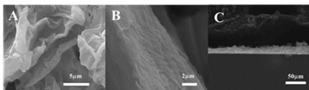
Fig. 2 SEM images of (A) GO at low magnification of 5  $\mu\text{m}$ , (B) GO/thionine nanocomposites at low magnification of 2  $\mu\text{m}$ , and (C) film thickness of the GO/thionine/AuNPs at low magnification (50  $\mu\text{m}$ ).
