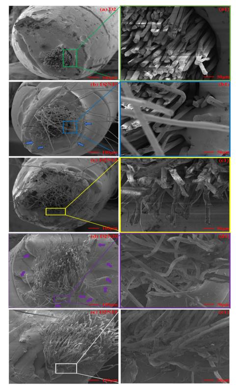
Fig. 8 Fractural morphologies affected by different alkali treatment times: (a) D2, (b) D2N10, (c) D2N15, (d) D2N20, and (e) D2N25. (a1), (b1), (c1), (d1) and (e1) is the enlargement of (a), (b), (c), (d) and (e), respectively.
