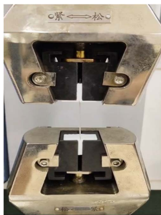
Fig. 4 Tensile tests of PCL/MS filaments while under load.
