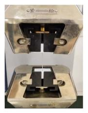
Fig. 4 Tensile tests of PCL/MS filaments while under load.
