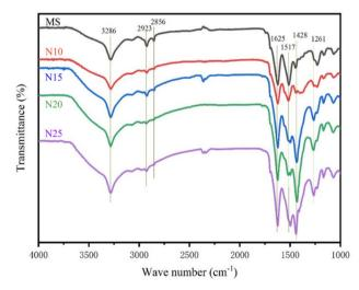
Fig. 5 FTIR of untreated and NaOH-treated MS filaments.
