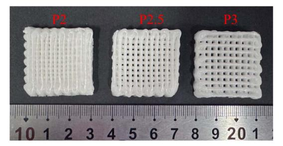
Fig. 10 Porous scaffolds of CL/MS composites
