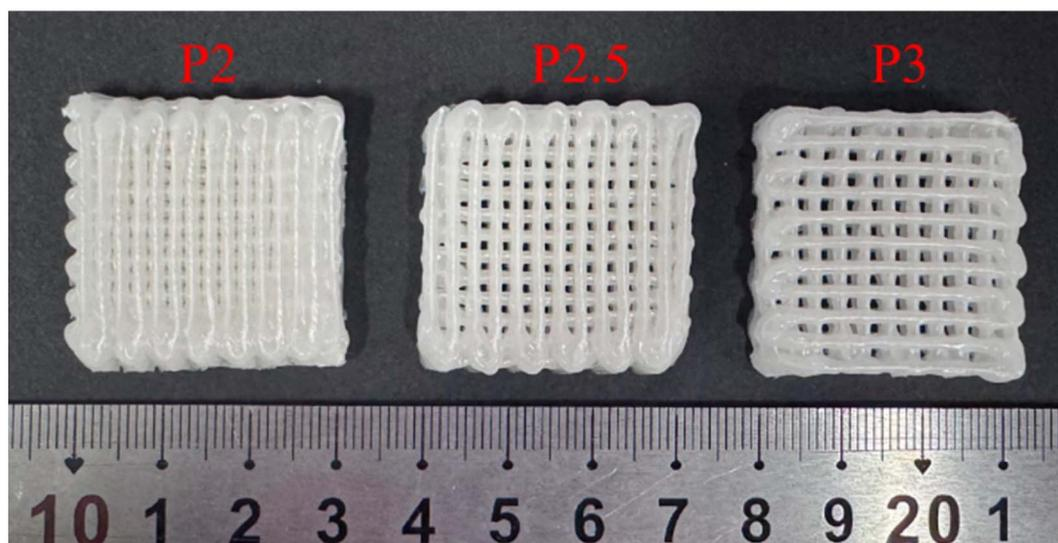
Fig. 10 Porous scaffolds of CL/MS composites.
