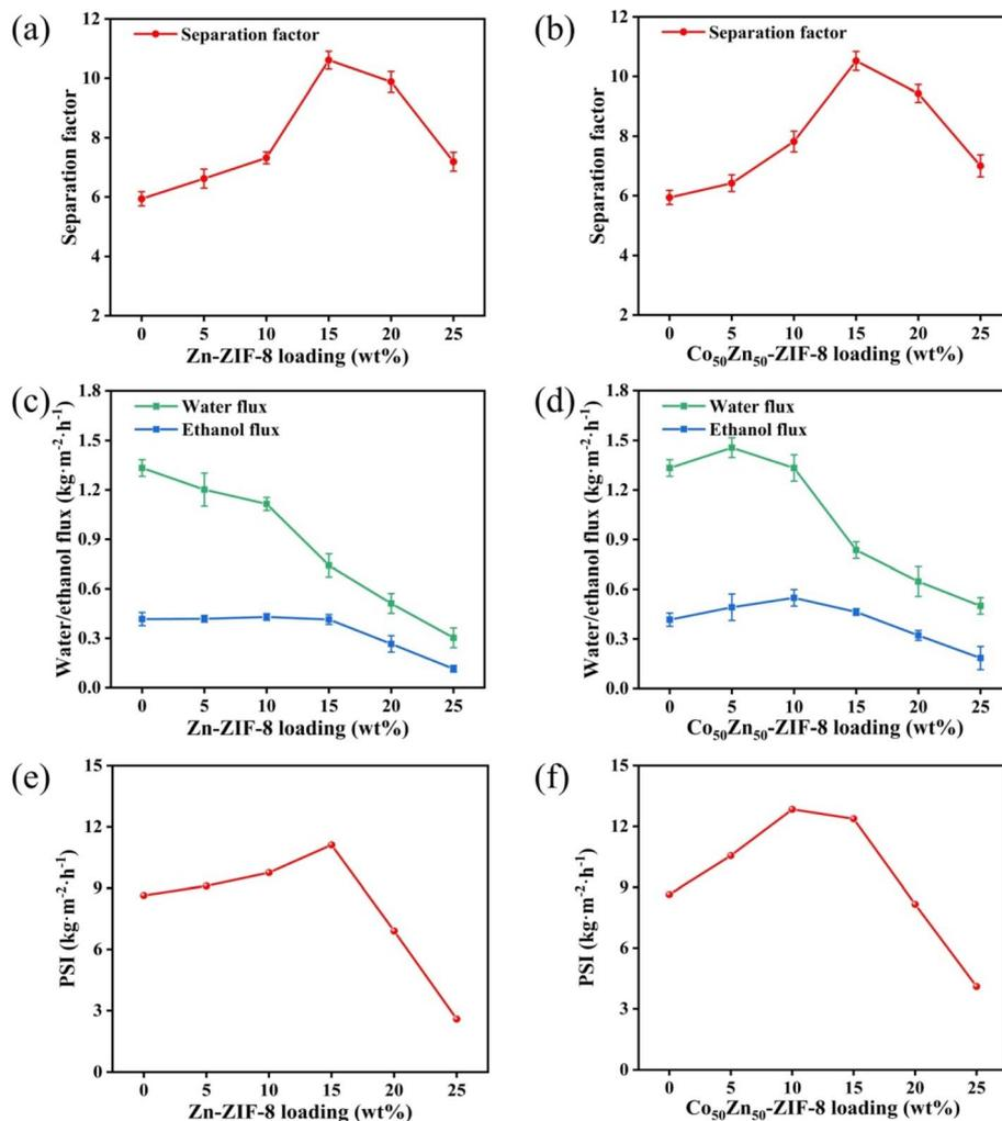
Fig. 11 Effect of different Zn-ZIF-8 and Co<sub>50</sub>Zn<sub>50</sub>-ZIF-8 loading on (a and b) pervaporation performance, (c and d) ethanol flux and water flux, and (e and f) pervaporation separation index of MMMs (operating conditions: 5.0 wt% ethanol aqueous solution, 60 °C).
