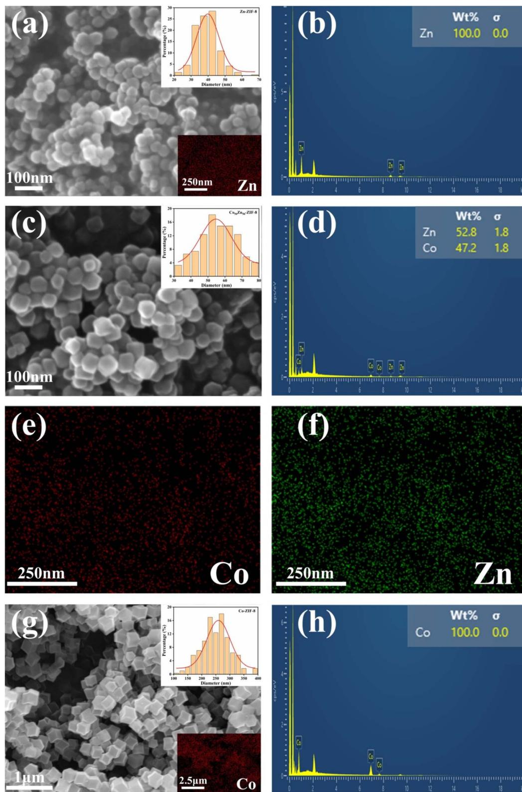
Fig. 5 SEM images with particle size distribution histogram (inset) and elemental mapping (inset lower right) of (a) Zn-ZIF-8, (c) Co<sub>50</sub>Zn<sub>50</sub>-ZIF-8 (elemental mapping provided in (e) and (f)) and (g) Co-ZIF-8. EDS spectra for (b) Zn-ZIF-8, (d) Co<sub>50</sub>Zn<sub>50</sub>-ZIF-8 and (h) Co-ZIF-8. (e and f) Elemental mappings of Co<sub>50</sub>Zn<sub>50</sub>-ZIF-8.
