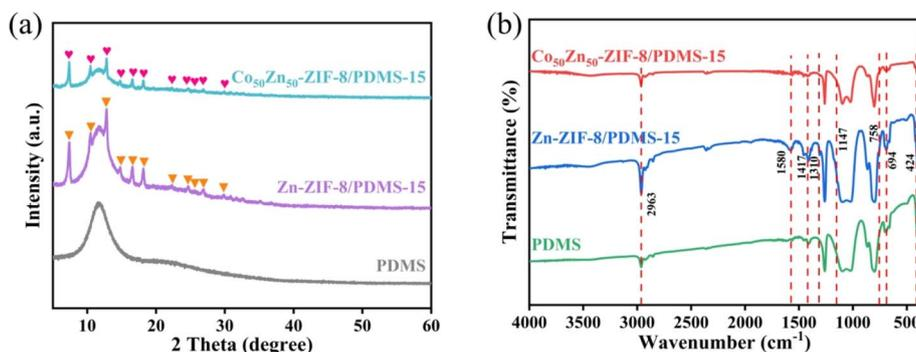
Fig. 7 (a) XRD patterns and (b) FT-IR spectra of pristine PDMS membrane, Zn-ZIF-8/PDMS-15 wt% and Co<sub>50</sub>Zn<sub>50</sub>-ZIF-8/PDMS-15 wt% MMMs.
