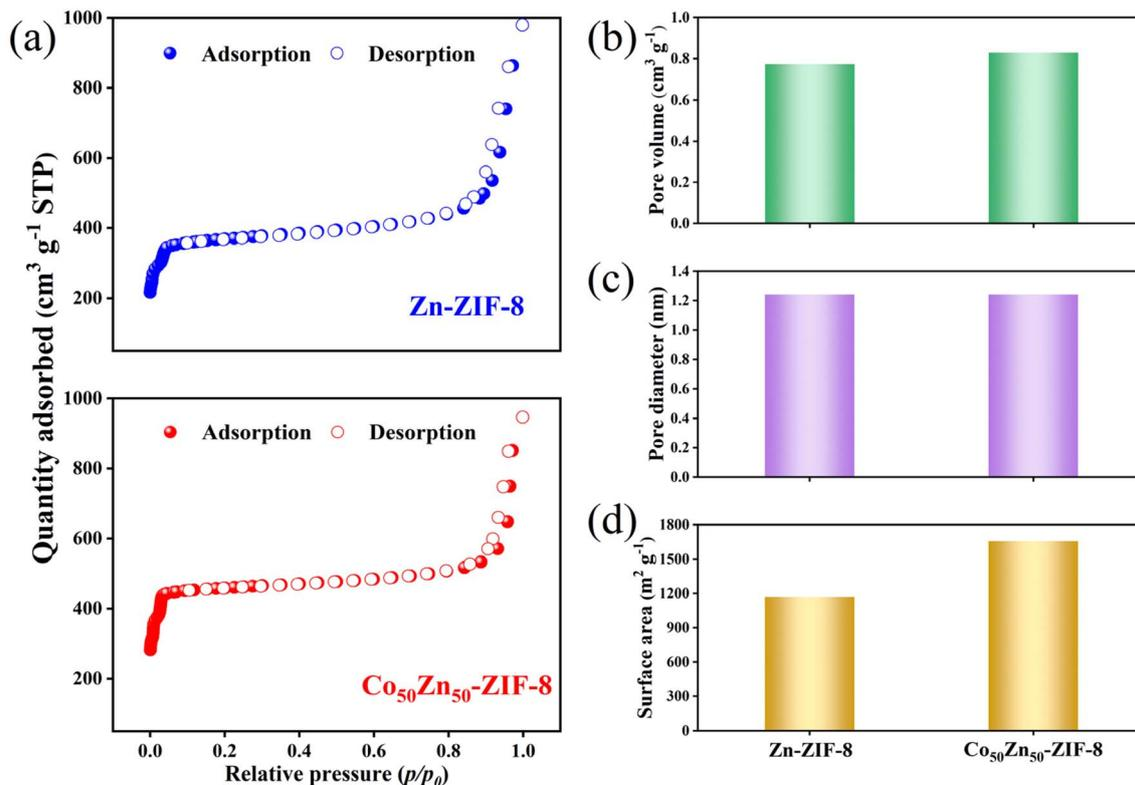
Fig. 6 (a) Nitrogen adsorption–desorption isotherms, (b) pore volume, (c) pore diameter and (d) surface area of Zn-ZIF-8 and Co<sub>50</sub>Zn<sub>50</sub>-ZIF-8 particles.
