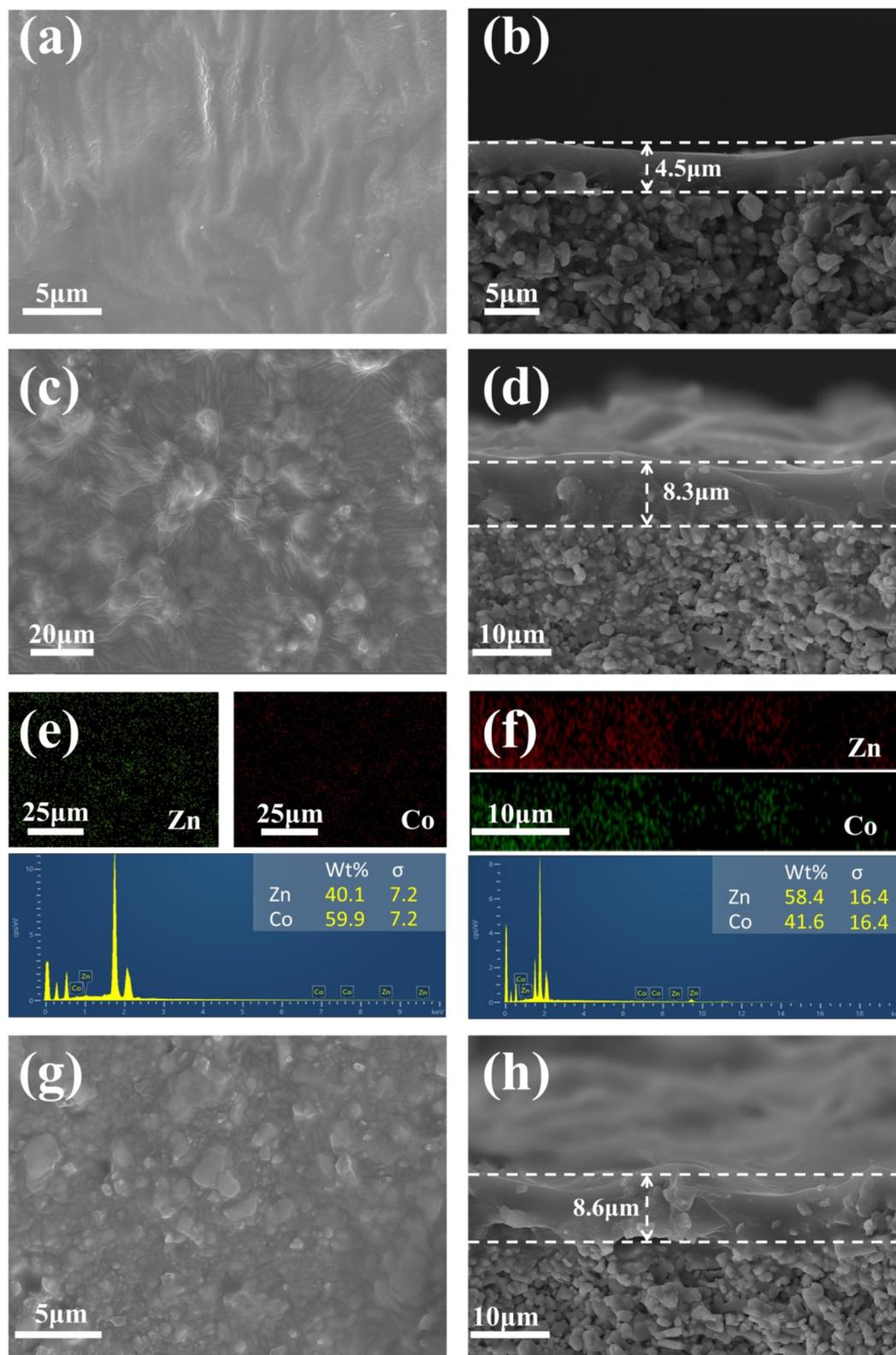
Fig. 8 SEM morphologies for surfaces and cross-sections of (a and b) pristine PDMS membrane, (c and d) Co<sub>50</sub>Zn<sub>50</sub>-ZIF-8/PDMS-15 wt% MMM and (g and h) Zn-ZIF-8/PDMS-15 wt% MMM, and elemental mapping and EDS spectra for (e) surfaces and (f) cross-sections of Co<sub>50</sub>Zn<sub>50</sub>-ZIF-8/PDMS-15 wt% MMM.
