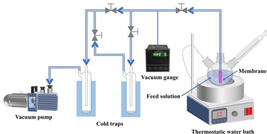
Fig. 2 Schematic of the pervaporation performance test device.
