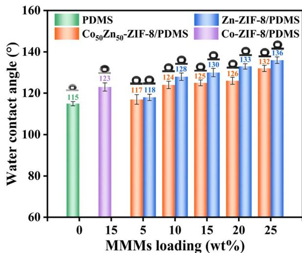
Fig. 9 Water contact angles of Zn-ZIF-8/PDMS and Co<sub>50</sub>Zn<sub>50</sub>-ZIF-8/PDMS MMMs with different particle loading levels, pristine PDMS membrane and Co-ZIF-8/PDMS-15 wt% MMM.
