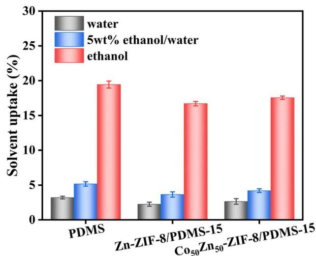
Fig. 10 Swelling degree of pristine PDMS membrane, Zn-ZIF-8/PDMS-15 wt% and Co<sub>50</sub>Zn<sub>50</sub>-ZIF-8/PDMS-15 wt% MMMs in various solutions.
