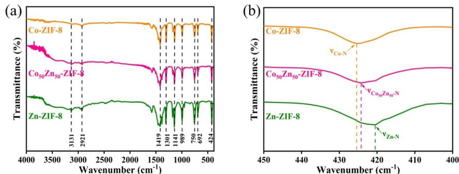
Fig. 4 FT-IR spectra of Zn-ZIF-8, Co<sub>50</sub>Zn<sub>50</sub>-ZIF-8 and Co-ZIF-8 particles.
