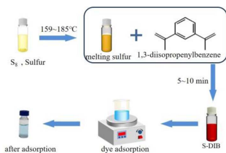
Fig. 1 Synthesis scheme and adsorption/photodegradation application of S-DIB for MB removal.
