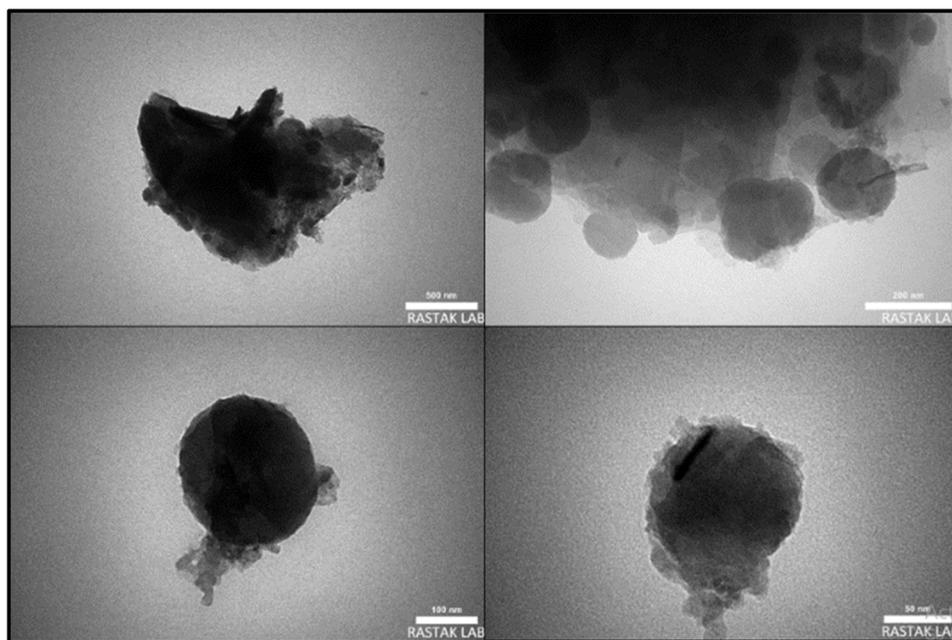
Fig. 8 TEM images of kaolin-[TMS]-NH<sub>2</sub><sup>+</sup>C(NO<sub>2</sub>)<sub>3</sub><sup>-</sup>.
