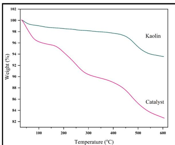
Fig. 5 TGA curves of kaolin and kaolin-[TMS]- $\text{NH}_2^+\text{C}(\text{NO}_2)_3^-$ .
