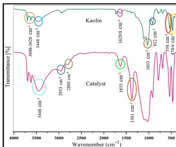
Fig. 3 FT-IR spectra of kaolin and kaolin-[TMS]- $\text{NH}_2^+\text{C}(\text{NO}_2)_3^-$ .
