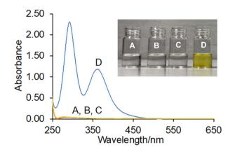
Fig. 7 UV-vis absorbance spectra (solvent subtracted) of 0.12 g L $^{-1}$  of poly(QN-co-AM) 2 in 1:1 (v/v) THF/water: (A)  $10^{-9}$  M H $^+$  (B)  $10^{-2}$  M H $^+$  (C)  $10^{-9}$  M H $^+$ , 1 mM I $^-$  (D)  $10^{-2}$  M H $^+$ , 1 mM I $^-$  after 10 min. The copolymer operates as a H $^+$ , I $^-$ -driven AND logic gate.
