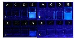
Fig. 5 Acrylamide copolymers 1–4 irradiated with 365 nm UV light in water in the presence of 0.1  $\mu$ M Na<sub>2</sub>EDTA. Condition (A)  $10^{-11}$  M H $^+$ , (B)  $10^{-2}$  M H $^+$ , (C)  $10^{-11}$  M H $^+$  & 100 mM Cl $^-$  and (D)  $10^{-2}$  M H $^+$  & 100 mM Cl $^-$ .
