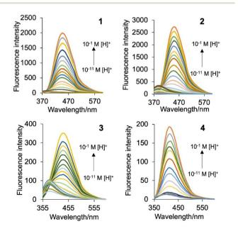
Fig. 3 The emission spectra of copolymers 1-4 in water excited at 352 nm, 345 nm, 316 nm and 315 nm, respectively, with increasing  $H^+$ .
