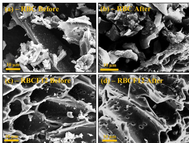
Fig. 2 SEM images of RBC (a) before and (b) after Fenton process; and RBCF12 (c) before and (d) after e-Fenton process.
