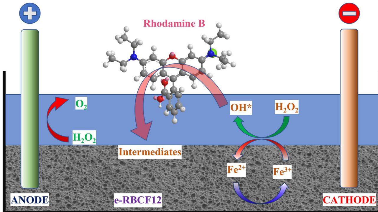
Fig. 6 RhB degradation mechanism of catalyst in electro Fenton process.
