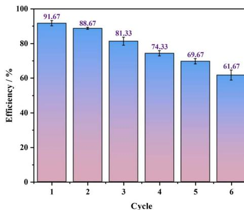
Fig. 4 Recyclability of e-RBCF12 catalyst in the electro-Fenton process for RhB removal efficiency ( $C_0 = 100 \text{ mg L}^{-1}$ ,  $\text{pH} = 3$ , dose =  $0.5 \text{ g L}^{-1}$ ,  $\text{H}_2\text{O}_2 = 20 \text{ mM}$ , electric current = 150 mA, electrode distance = 2 cm, time = 120 min).
