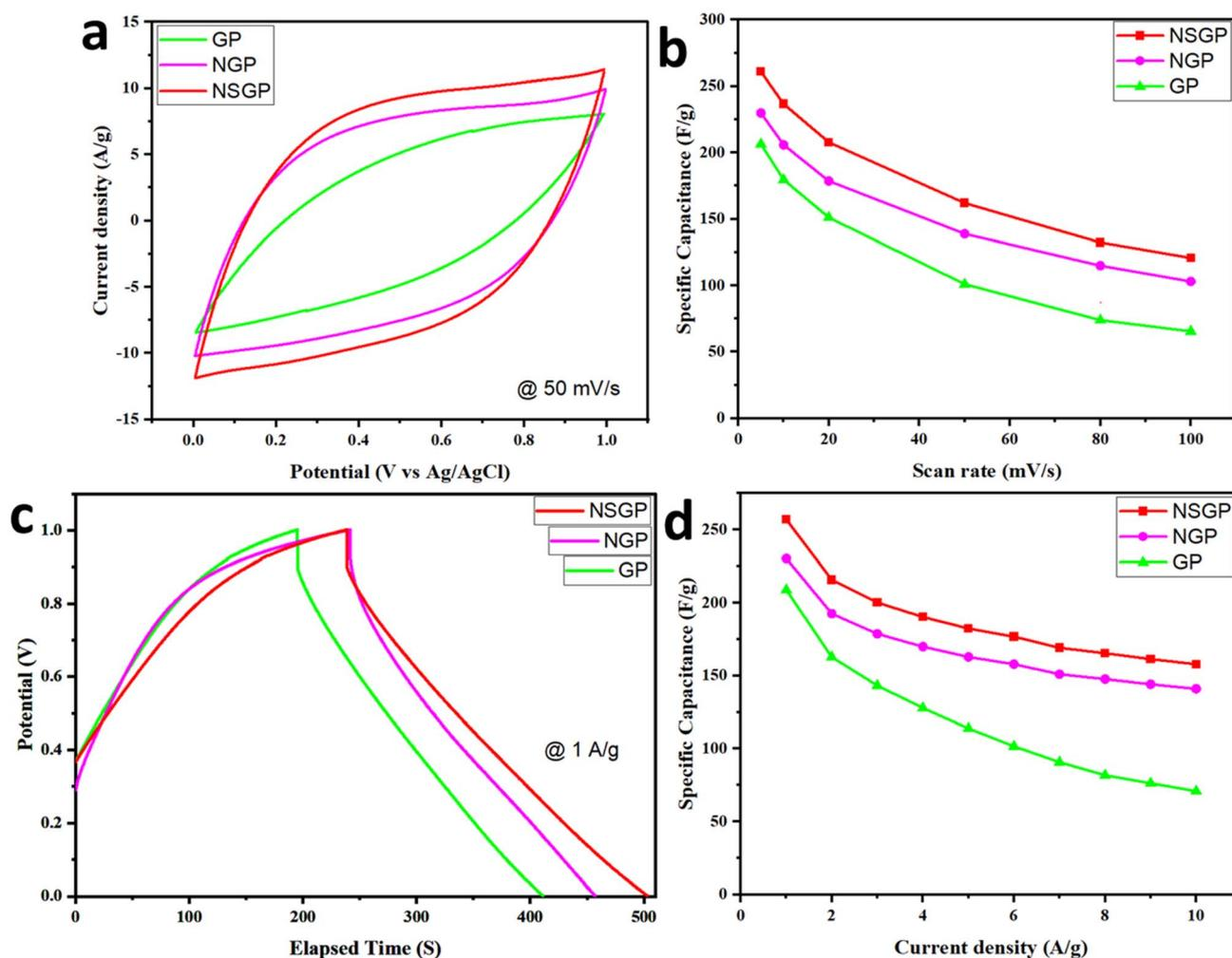
Fig. 6 (a) CV curves of GP, NGP, and NSGP at  $50 \text{ mV s}^{-1}$  and (b) CV-specific capacitances of GP, NGP, and NSGP, (c) GCD curves of GP, NGP, and NSGP at  $1 \text{ A g}^{-1}$ , and (d) specific capacitances of GP, NGP, and NSGP in a three-electrode configuration.
