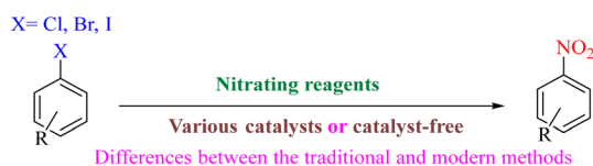
Scheme 67 General methods for the ipso-nitration of halogens [X] as leaving groups.
