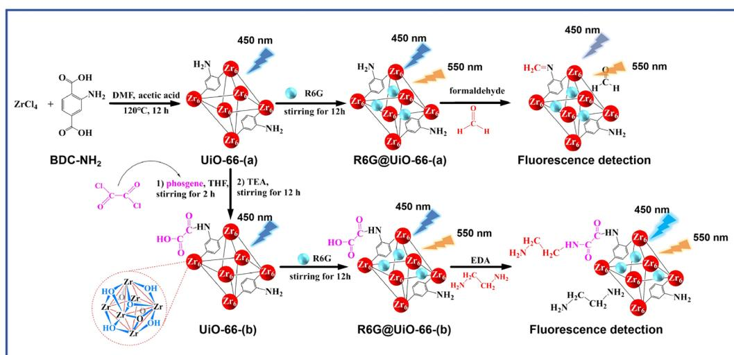
Scheme 1 The schematic diagrams of the preparation route of R6G@UiO-66-(a) and R6G@UiO-66-(b) and their application for aldehydes and amines compounds detection, respectively.
