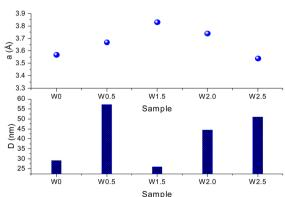
Fig. 3 The XRD of CdO-ZnO-W-P<sub>2</sub>O<sub>5</sub> (CZWP) showing different doping wt% of W in the structure (up), and the lattice parameter dimensions with the crystallite size depiction (down).
