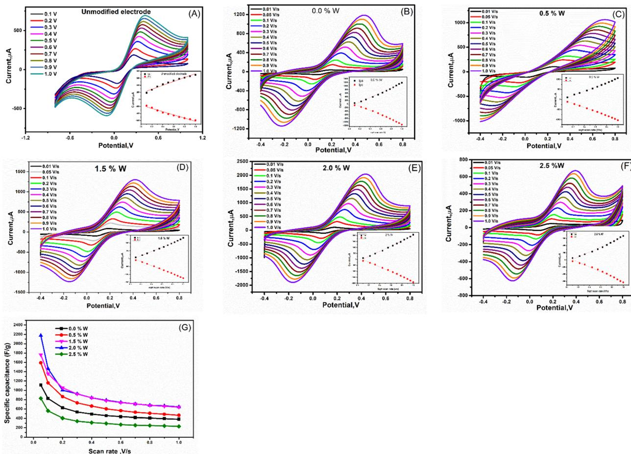
Fig. 14 (A–F) CVs for synthesized CdO-ZnO-W-P<sub>2</sub>O<sub>5</sub> (CZWP) with different % of tungsten (W) modified SPEs at different scan rates and the inset figures are  $I_{pa}$  and  $I_{pc}$  curves of all modified SPEs at different scan rates. (G) Specific capacitance of CZWP with 0.0% W, 0.5% W, 1.5% W, 2.0% W and 2.5% W modified SPE at different scan rates.
