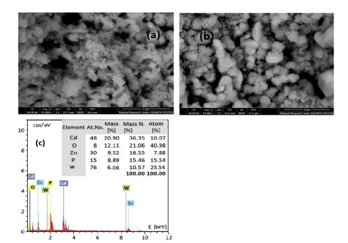
Fig. 6 SEM morphology of: (a) undoped CdZn-phosphate nanoporous, (b) CdZn-phosphate doped 2.5 mol% W, and (c) the particle distribution.
