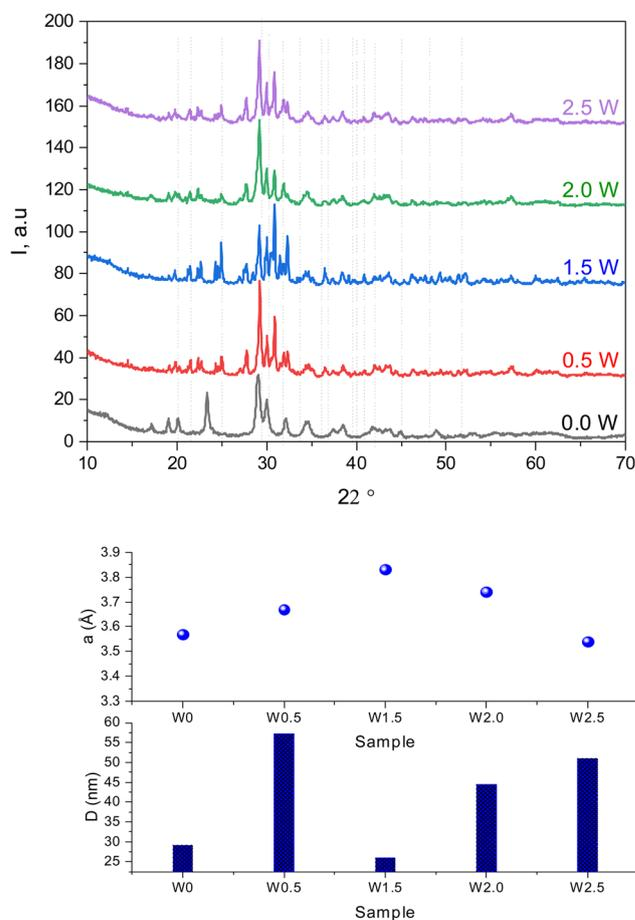
Fig. 3 The XRD of CdO-ZnO-W-P<sub>2</sub>O<sub>5</sub> (CZWP) showing different doping wt% of W in the structure (up), and the lattice parameter dimensions with the crystallite size depiction (down).
