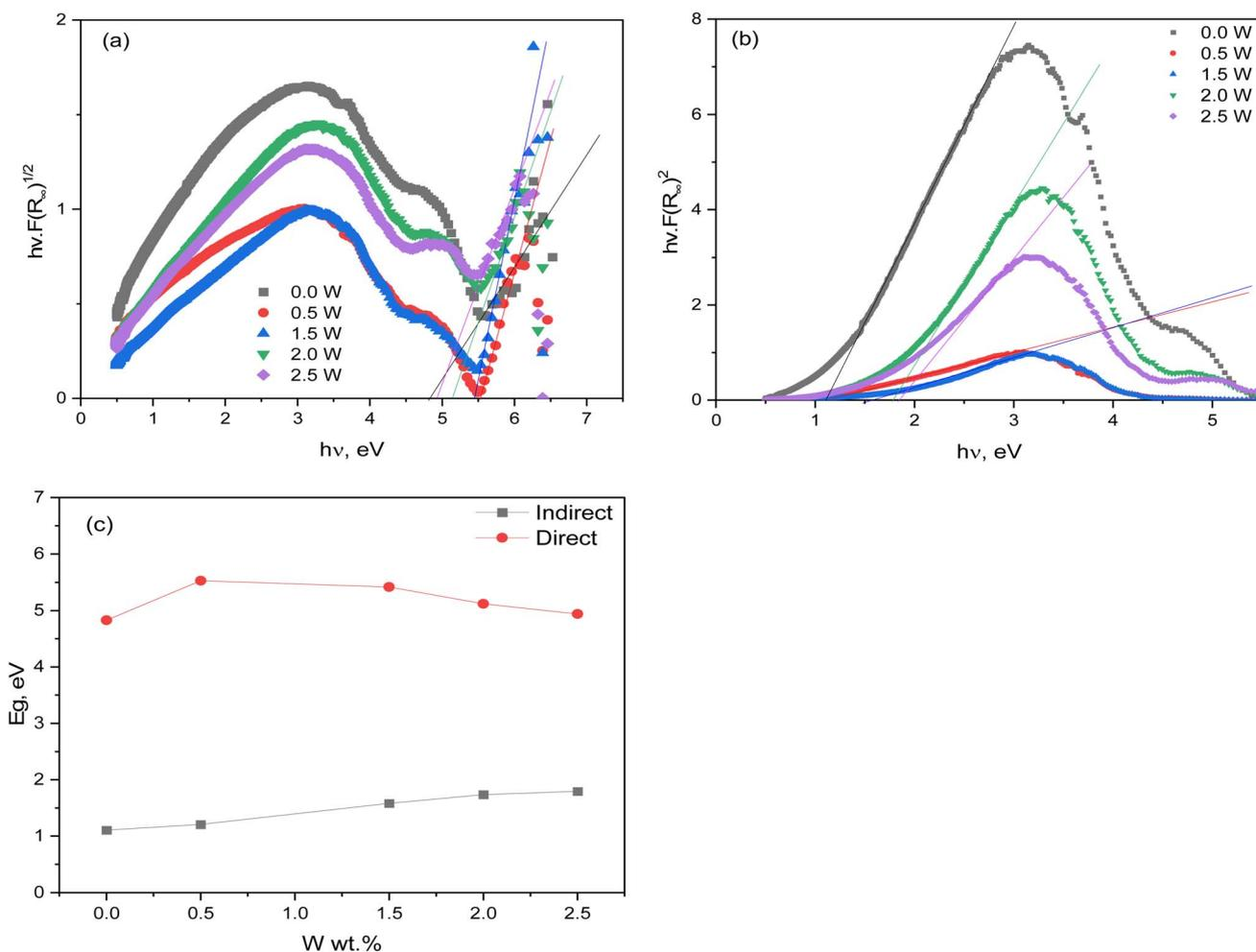
Fig. 11 The Kubelka–Munk function versus incident photon energy for (a) direct and (b) indirect cases. (c) the dependence of band gap on tungsten addition.
