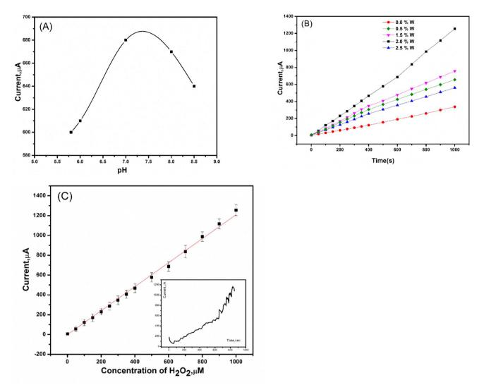
Fig. 17 (A) The pH effect study on 2 W/SPE performance towards the peroxide sensitivity. (B) The corresponding calibration curve of 0 W, 0.5 W, 1.5 W, 2 W and 2.5 W modified SPE toward  $H_2O_2$  response. (C). The corresponding calibration curve of 2 W modified SPE toward  $H_2O_2$  response.
