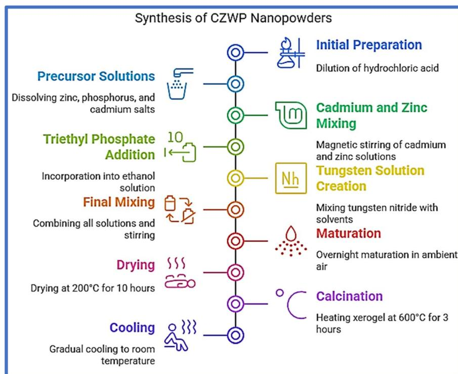
Fig. 1 Schematic diagram of materials synthesis process.
