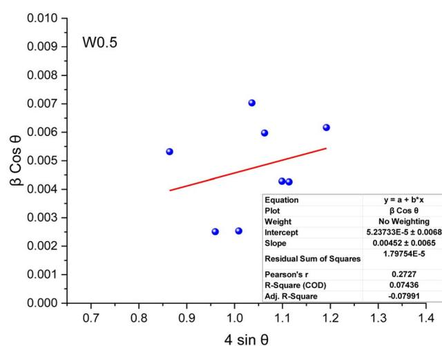
Fig. 4 The relation between  $\beta \cos \theta$  and  $4 \sin \theta$ , at where the crystallite size and microstrain are seized from the slope and intercept, familiarly denoted as Williamson–Hall plot.
