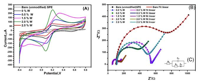
Fig. 13 The (A) CV and (B) EIS measurements of (0, 0.5, 1.5, 2 and 2.5 W) SPEs were measured by using standard redox solution (ferro/ferri cyanide/KCI) with 50 mV s<sup>-1</sup> scan rate. (C) Circuit which used to fit the Nyquist plot of EIS data.
