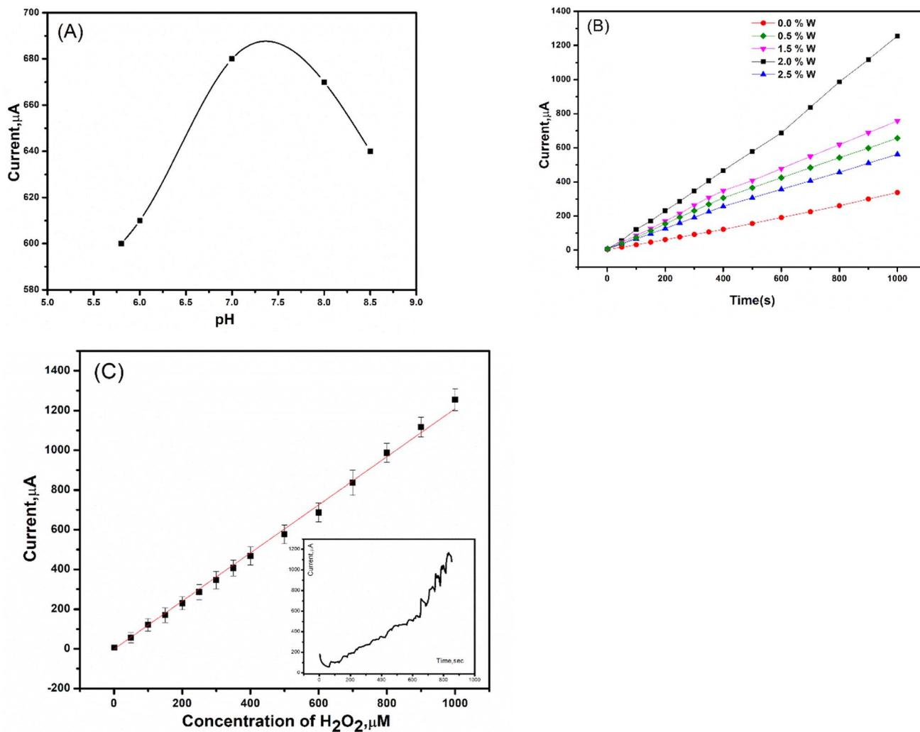
Fig. 17 (A) The pH effect study on 2 W/SPE performance towards the peroxide sensitivity. (B) The corresponding calibration curve of 0 W, 0.5 W, 1.5 W, 2 W and 2.5 W modified SPE toward  $\text{H}_2\text{O}_2$  response. (C). The corresponding calibration curve of 2 W modified SPE toward  $\text{H}_2\text{O}_2$  response.
