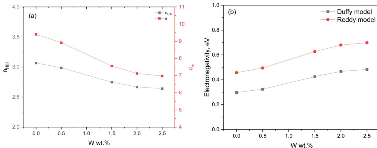
Fig. 12 (a) The refractive index ( $n$ ) and the dielectric constant in the case of an indirect transition gap, and (b) the calculated optical electronegativity of nanocomposites doped by different W content.
