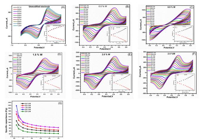
Fig. 14 (A–F) CVs for synthesized CdO-ZnO-W-P<sub>2</sub>O<sub>5</sub> (CZWP) with different % of tungsten (W) modified SPEs at different scan rates and the inset figures are  $I_{\rm pa}$  and  $I_{\rm pc}$  curves of all modified SPEs at different scan rates. (G) Specific capacitance of CZWP with 0.0% W, 0.5% W, 1.5% W, 2.0% W and 2.5% W modified SPE at different scan rates.
