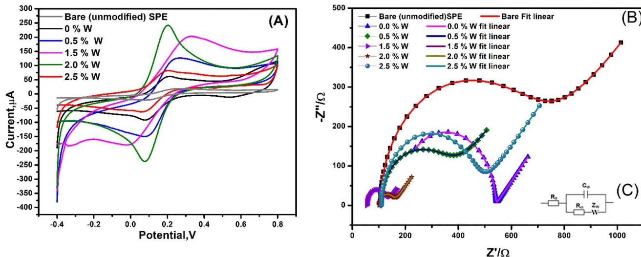
Fig. 13 The (A) CV and (B) EIS measurements of (0, 0.5, 1.5, 2 and 2.5 W) SPEs were measured by using standard redox solution (ferro/ferricyanide/KCl) with  $50 \text{ mV s}^{-1}$  scan rate. (C) Circuit which used to fit the Nyquist plot of EIS data.
