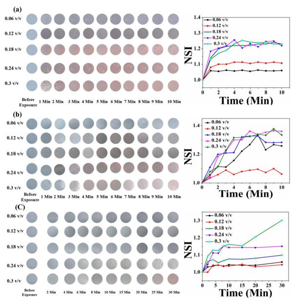
Fig. 12 Time- and concentration-dependent colorimetric response to the HCDA/AgNP (5%)-based paper sensor upon exposure to (a) pesticide  $P_1$ , (b) pesticide  $P_2$  and (c) pesticide  $P_3$ . The respective NSI values are presented alongside each set of colorimetric transitions, demonstrating the sensor's response across different concentrations and time intervals.
