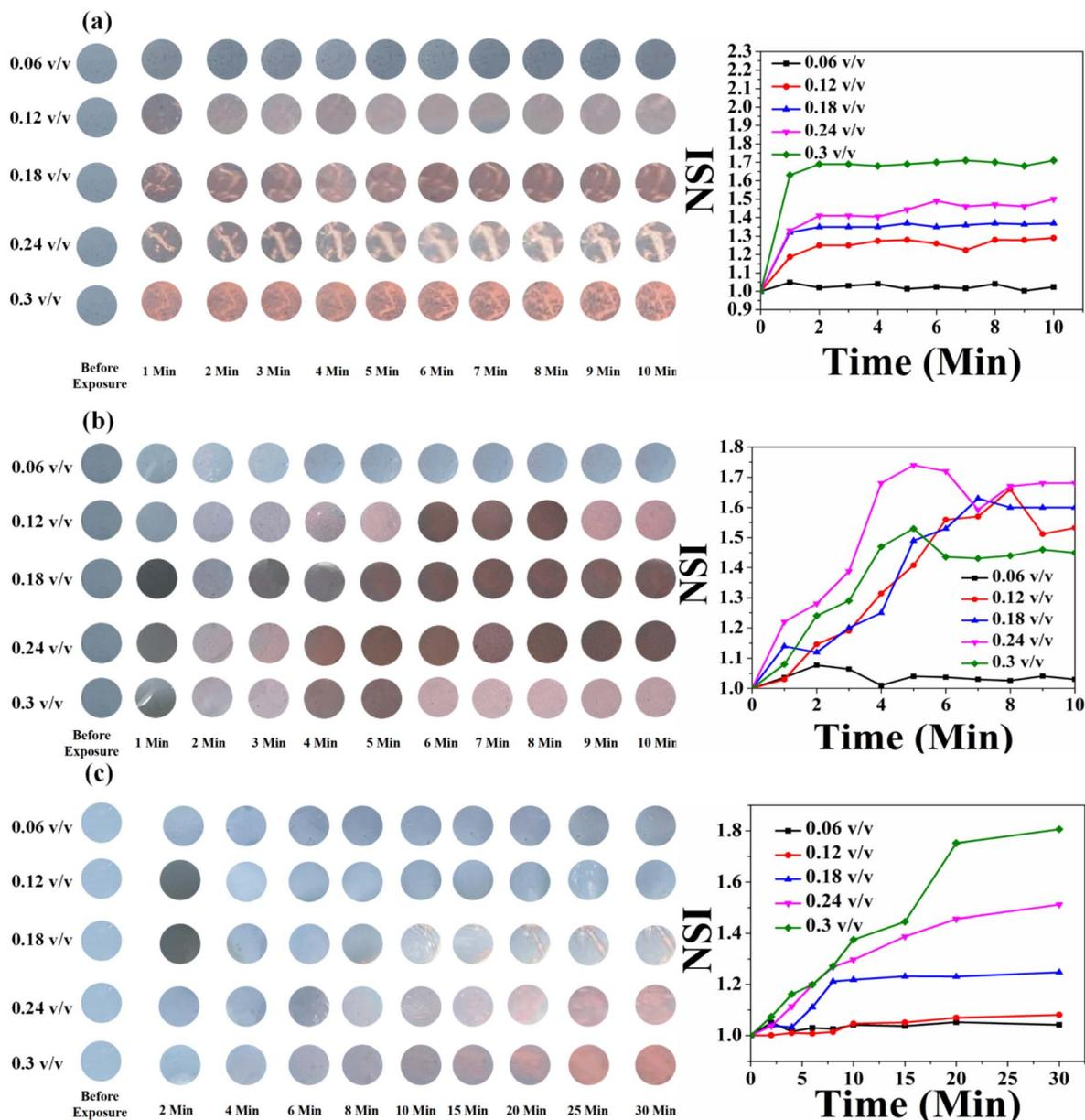
Fig. 14 Time- and concentration-dependent colorimetric response of the HCDA/AgNP (15%)-based paper sensor upon exposure to (a) pesticide P<sub>1</sub>, (b) pesticide P<sub>2</sub> and (c) pesticide P<sub>3</sub>. The respective NSI values are presented alongside each set of colorimetric transitions, demonstrating the sensor's response across different concentrations and time intervals.
