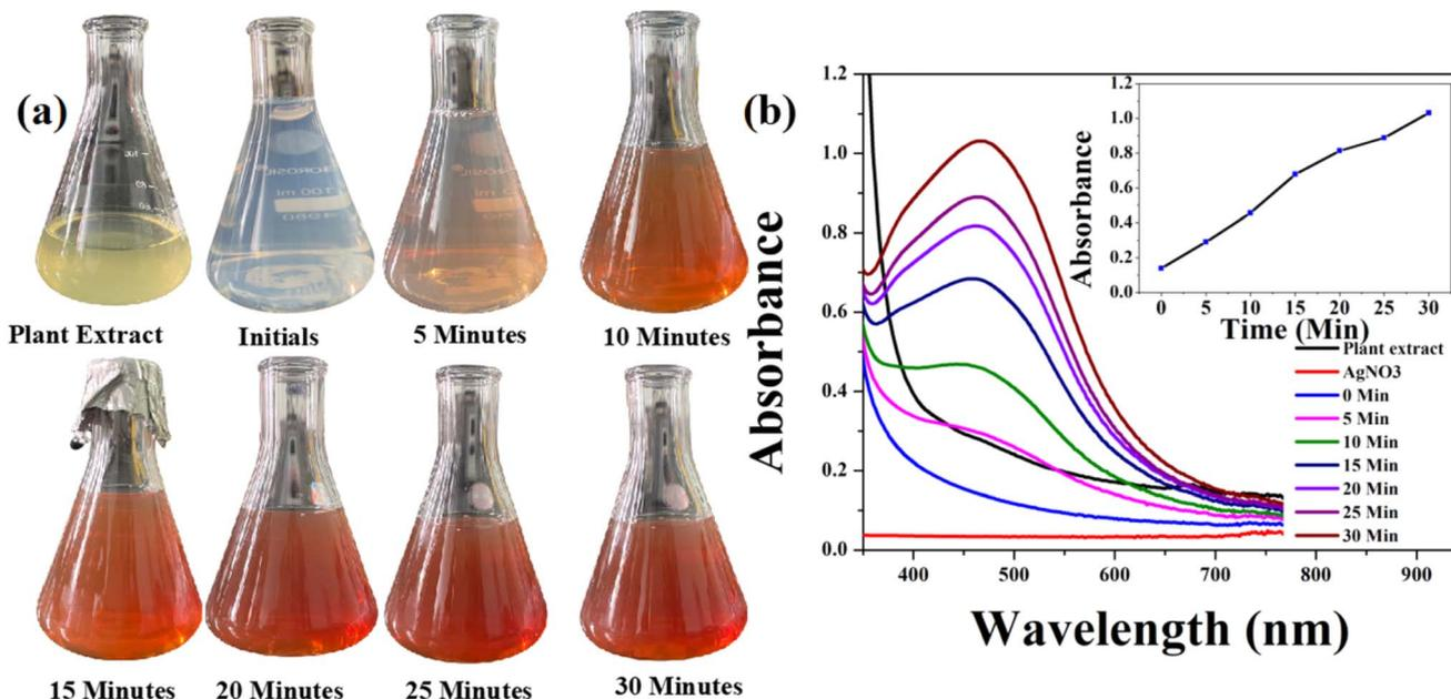
Fig. 1 Formation of biosynthesized AgNPs: (a) colour change profile during the formation of AgNPs and (b) time-dependent UV-Vis absorption spectra of the synthesized AgNPs. Inset: plot of the absorbance (466 nm) of AgNPs versus incubation time.
