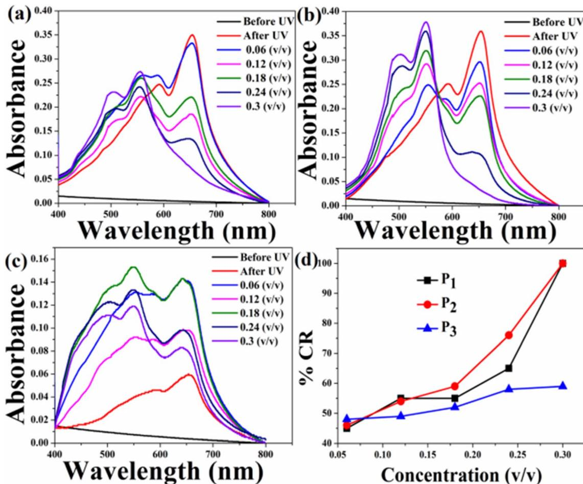
Fig. 9 CR and respective absorption spectra of the HCDA/AgNP (10%) sensing system upon exposure to (a) pesticide P<sub>1</sub>, (b) pesticide P<sub>2</sub> and (c) pesticide P<sub>3</sub> at different concentrations, and (d) % CR of pesticides P<sub>1</sub>, P<sub>2</sub> and P<sub>3</sub> as calculated from (a)–(c).
