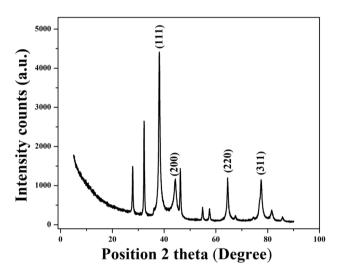
Fig. 5 X-ray diffraction pattern of the synthesized AgNPs
