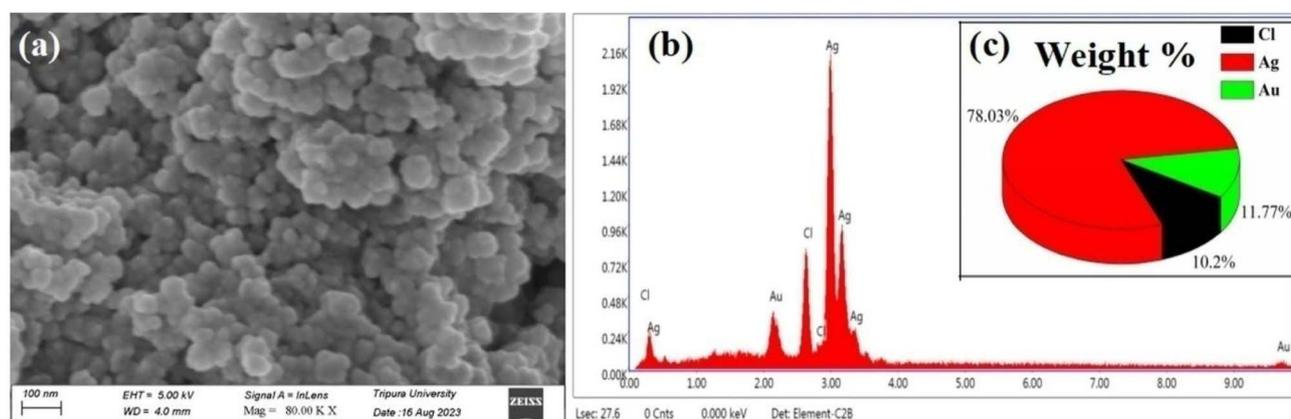
Fig. 2 (a) FESEM images of the biosynthesized AgNPs using *A. heterophylla* leaf extract. (b) EDAX spectrum of the synthesized AgNPs. (c) Weight percentage of the elemental composition of the biosynthesized AgNPs obtained from EDX analysis.
