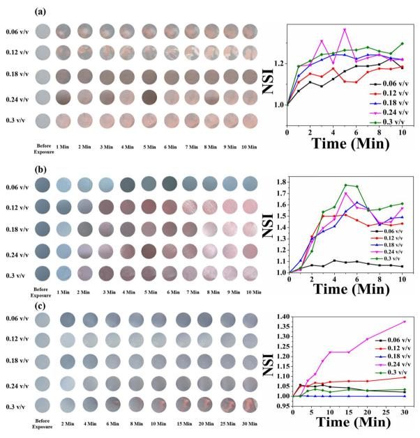
Fig. 13 Time- and concentration-dependent colorimetric response of the HCDA/AgNP (10%)-based paper sensor upon exposure to (a) pesticide P<sub>1</sub>, (b) pesticide P<sub>2</sub> and (c) pesticide P<sub>3</sub>. The respective NSI values are presented alongside each set of colorimetric transitions, demonstrating the sensor's response across different concentrations and time intervals.
