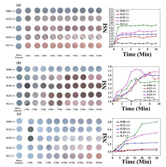
Fig. 14 Time- and concentration-dependent colorimetric response of the HCDA/AgNP (15%)-based paper sensor upon exposure to (a) pesticide  $P_1$ , (b) pesticide  $P_2$  and (c) pesticide  $P_3$ . The respective NSI values are presented alongside each set of colorimetric transitions, demonstrating the sensor's response across different concentrations and time intervals.
