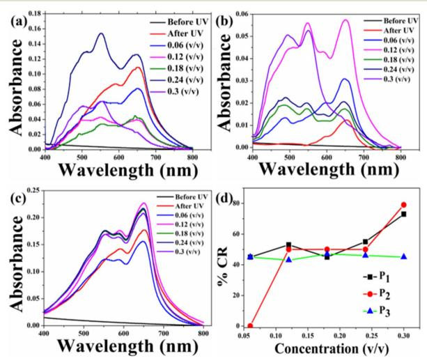
Fig. 8 Absorption spectra of the HCDA/AgNP (5%) sensing system upon exposure to (a) pesticide  $P_1$ , (b) pesticide  $P_2$ , and (c) pesticide  $P_3$  with different concentrations, and (d) % CR of pesticides  $P_1$ ,  $P_2$  and  $P_3$  as calculated from (a–c).
