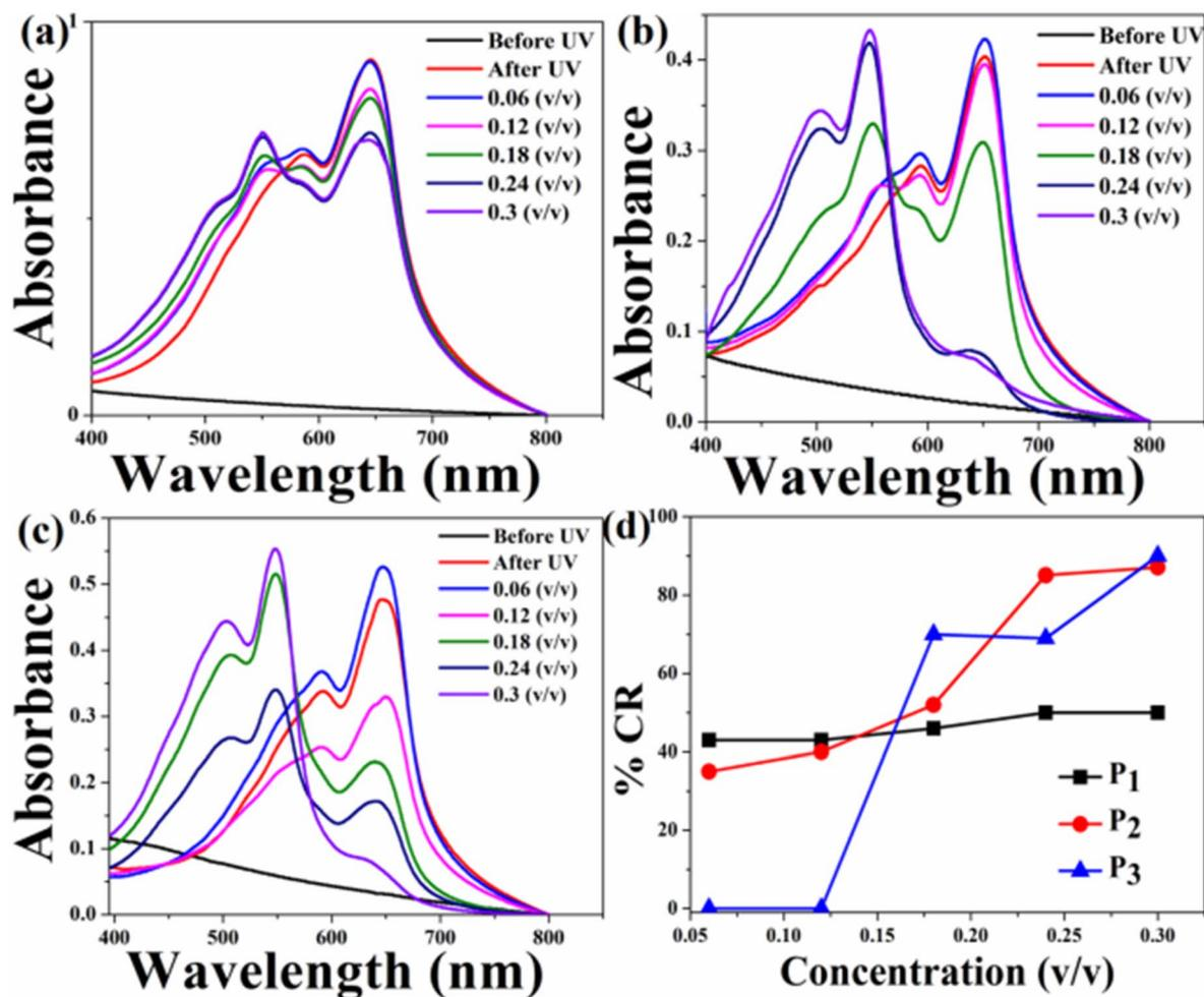
Fig. 10 Absorption spectra of the HCDA/AgNP (15%) sensing system upon exposure to (a) pesticide  $P_1$ , (b) pesticide  $P_2$  and (c) pesticide  $P_3$  at different concentrations, and (d) %CR of pesticides  $P_1$ ,  $P_2$  and  $P_3$  as calculated from (a)–(c).
