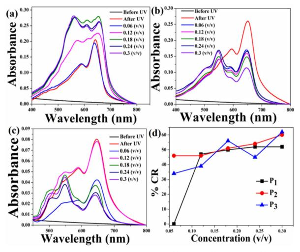
Fig. 7 Absorption spectra of the pure HCDA sensing system upon exposure to (a) pesticide  $P_1$ , (b) pesticide  $P_2$ , and (c) pesticide  $P_3$  at varied concentrations, and (d) % CR of pesticides  $P_1$ ,  $P_2$  and  $P_3$ , as calculated from (a)–(c).
