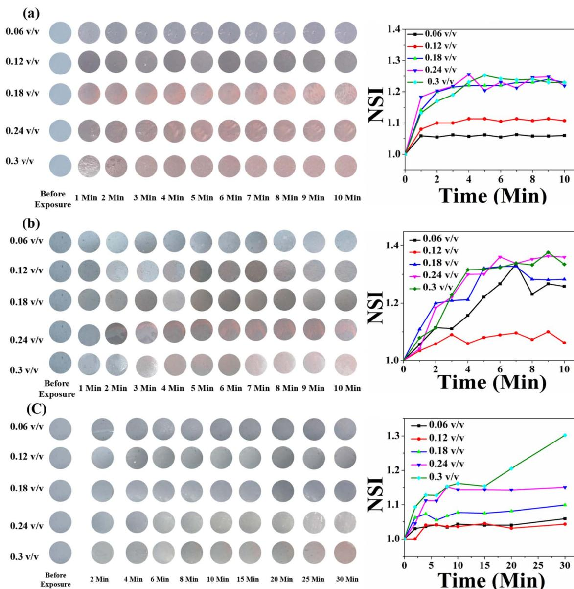
Fig. 12 Time- and concentration-dependent colorimetric response to the HCDA/AgNP (5%)-based paper sensor upon exposure to (a) pesticide P<sub>1</sub>, (b) pesticide P<sub>2</sub> and (c) pesticide P<sub>3</sub>. The respective NSI values are presented alongside each set of colorimetric transitions, demonstrating the sensor's response across different concentrations and time intervals.
