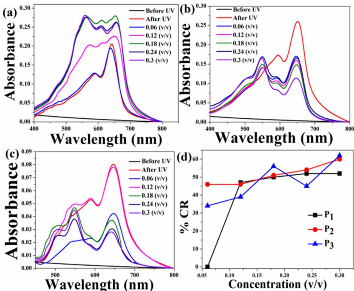
Fig. 7 Absorption spectra of the pure HCDA sensing system upon exposure to (a) pesticide P<sub>1</sub>, (b) pesticide P<sub>2</sub>, and (c) pesticide P<sub>3</sub> at varied concentrations, and (d) % CR of pesticides P<sub>1</sub>, P<sub>2</sub> and P<sub>3</sub>, as calculated from (a)–(c).
