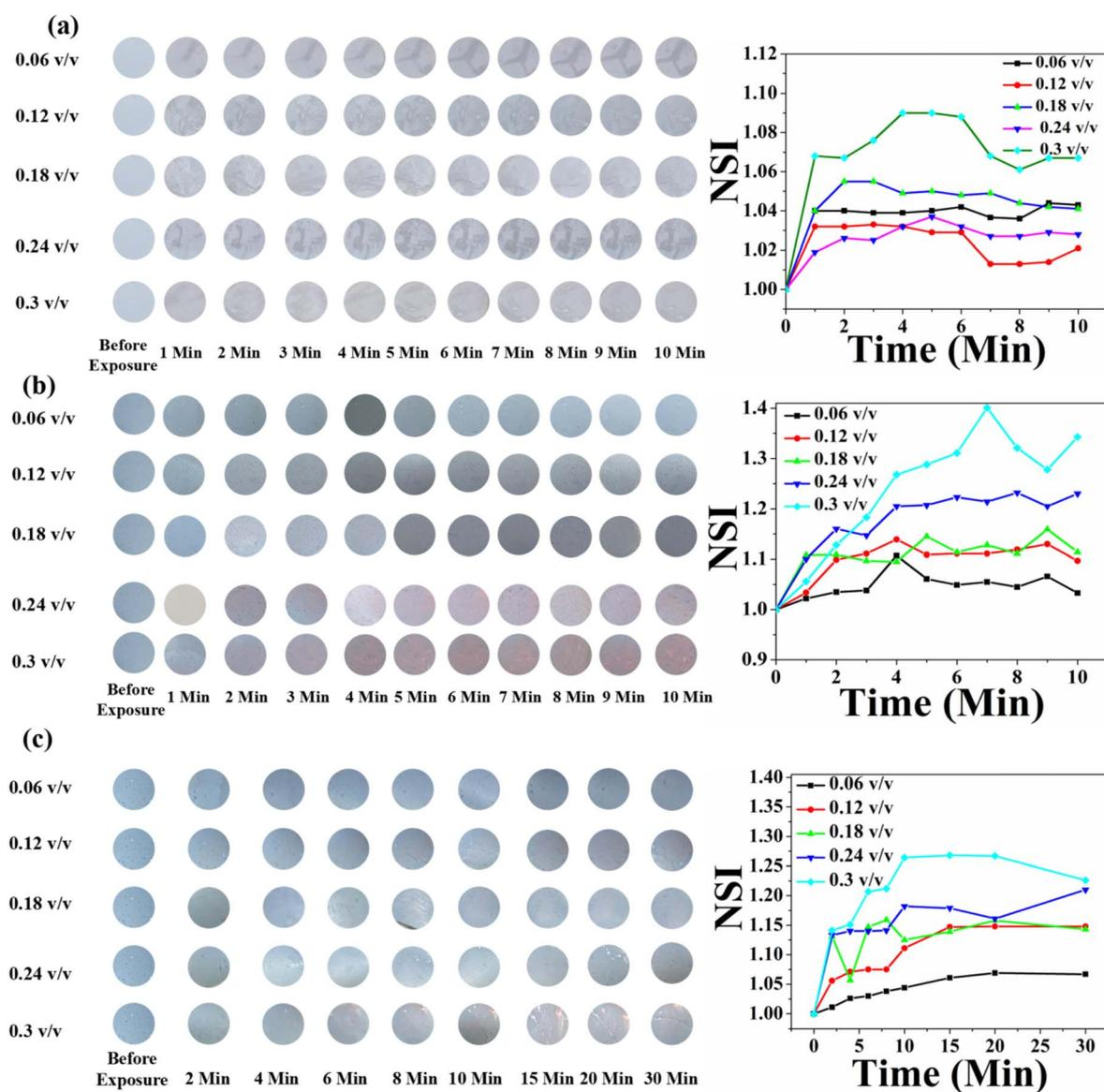
Fig. 11 Time- and concentration-dependent colorimetric response of pure HCDA-based paper sensors upon exposure to (a) pesticide P<sub>1</sub>, (b) pesticide P<sub>2</sub> and (c) pesticide P<sub>3</sub>. The respective NSI values are presented alongside each set of colorimetric transitions, demonstrating the sensor's response across different concentrations and time intervals.
