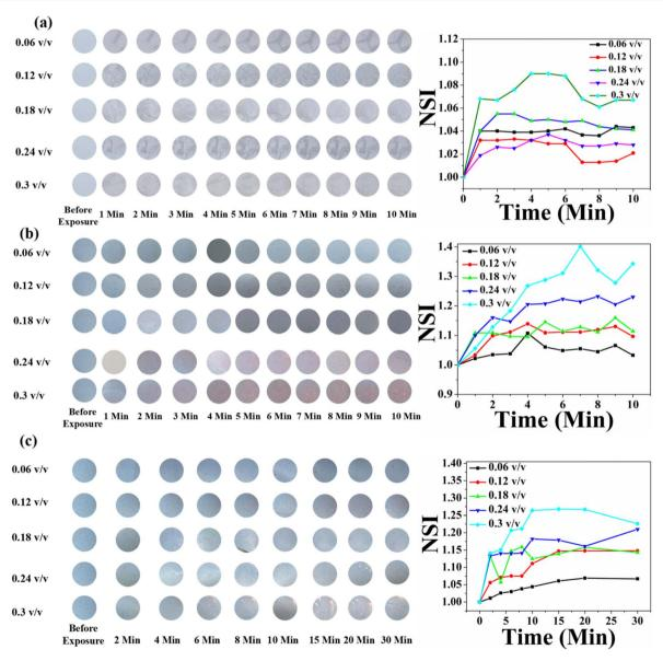
Fig. 11 Time- and concentration-dependent colorimetric response of pure HCDA-based paper sensors upon exposure to (a) pesticide P<sub>1</sub>, (b) pesticide P2 and (c) pesticide P3. The respective NSI values are presented alongside each set of colorimetric transitions, demonstrating the sensor's response across different concentrations and time intervals.
