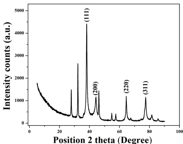
Fig. 5 X-ray diffraction pattern of the synthesized AgNPs.
