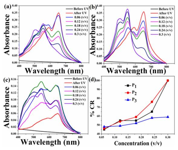
Fig. 9 CR and respective absorption spectra of the HCDA/AgNP (10%) sensing system upon exposure to (a) pesticide  $P_1$ , (b) pesticide  $P_2$  and (c) pesticide  $P_3$  at different concentrations, and (d) % CR of pesticides  $P_1$ ,  $P_2$  and  $P_3$  as calculated from (a)–(c).
