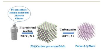
Fig. 1 Schematic of the preparation process of porous C@MoS<sub>2</sub>.
