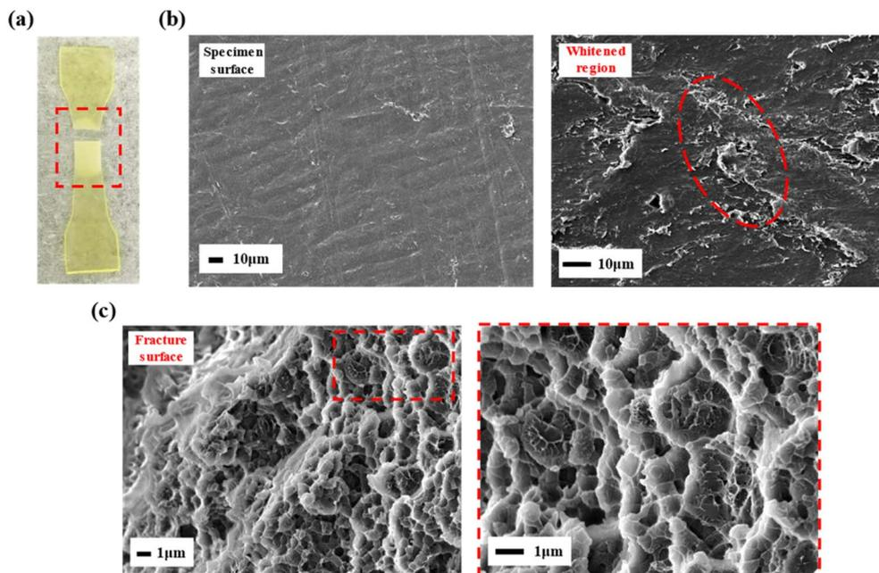
Fig. 2 (a) Fractured specimen of poly(urethane-MMA) (run 3 in Table 2). (b) SEM images of the transparent region and whitened region (0.1 mm from the edge) of the fracture piece. (c) SEM images of the fracture surface of the fracture piece.
