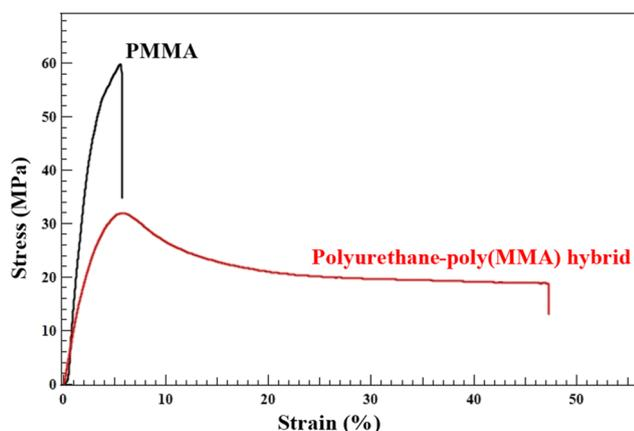
Fig. 1 Stress–strain curves of polyurethane–poly(MMA) hybrid (run 3 in Table 2) and MMA homopolymer (room temperature, 10 mm min<sup>-1</sup>).
