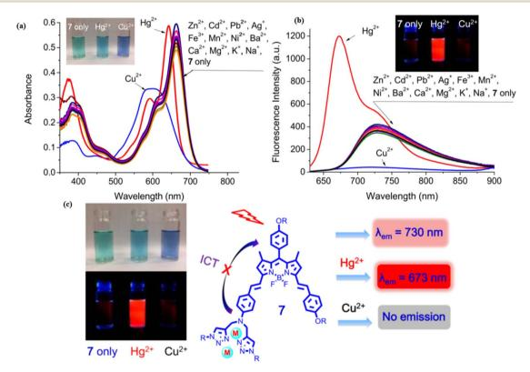
Fig. 18 (a) Change in absorption spectra of probe 47 (6  $\mu$ M) in CH<sub>3</sub>CN/H<sub>2</sub>O (5:1  $\nu$ /v) upon addition of different metal ions (20 equiv.); (b) change in fluorescence spectra of probe 47 (6  $\mu$ M) in CH<sub>3</sub>CN/H<sub>2</sub>O (5:1  $\nu$ /v) upon addition of different metal ions (20 equiv.); (c) the ratiometric and discriminative detection of Hg<sup>2+</sup> and Cu<sup>2+</sup> ions; Reproduced with permission from ref. 92. Copyright 2018, Elsevier.
