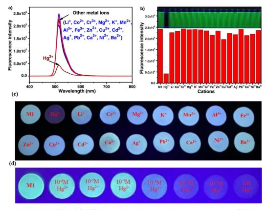
Fig. 16 (a) Emission spectra of probe 37 in H<sub>2</sub>O/DMF (8:2) upon the addition of 4 equivalents of various metal ions; (b) fluorescence intensity at 517 nm of probe 37 in  $H_2O/DMF$  (8:2) with various metal ions (5 equivalents). (c) Test strips exposed to various metal ions when illuminated at 365 nm. (d) Images of the test strips treated with different concentrations of mercury ions. Reproduced with permission from ref. 44. Copyright 2022, Elsevier.
