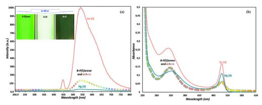
Fig. 13 (a) Emission spectra of probe 14 in  $H_2O/CH_3CN$  (1:1) (1  $\mu$ M) in presence of various metal ions. (b) The absorption spectra of probe 14 in  $H_2O/CH_3CN$  (1:1) (1  $\mu$ M) in presence of various metal ions. Reproduced with permission from ref. 62. Copyright 2022, Elsevier.
