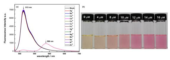
Fig. 15 (a) Fluorescence emission of probe 27 (10  $\mu$ M) with and without various metal ions (100  $\mu$ M); (b) color change of probe 27 (10  $\mu$ M) with different concentrations of Hg<sup>2+</sup> (0–16  $\mu$ M) in MeOH/20 mM HEPES buffer (V/V = 7:3, pH = 6.0) under the daylight. Reproduced with permission from ref. 82. Copyright 2021, Elsevier.
