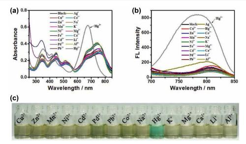
Fig. 21 (a) UV-vis spectra of probe 58 in presence of different ions. (b) Emission spectra of probe 58 in presence of different ions. (c) Color change of probe 58 in daylight upon addition of 100  $\mu$ M of different ions in DMF-H<sub>2</sub>O (v/v = 3:7). Reproduced with permission from ref. 100. Copyright 2022, Elsevier.
