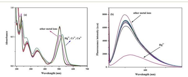
Fig. 24 (a) Absorption and (b) emission spectra of probe 97 in acetonitrile/water (7:3, v/v) solution with 10 equivalents of various metal ions. Reproduced with permission from ref. 104. Copyright 2024, Elsevier.
