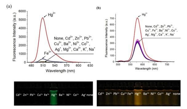
Fig. 14 (a) Emission spectra of 19 (2  $\mu$ m) in CH<sub>3</sub>CN/H<sub>2</sub>O (9 : 1, v/v) upon interaction with different metal ions and the color shifts when exposed to a UV lamp at 365 nm. (b) Emission spectra of 20 (2  $\mu$ m) in CH<sub>3</sub>CN/H<sub>2</sub>O (9 : 1, v/v) upon interaction with different metal ions and the color shifts when exposed to a UV lamp at 365 nm. Reproduced with permission from ref. 81. Copyright 2019, Wiley-VCH.
