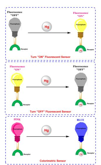
Fig. 3 Schematic overview of various types of colorimetric and/or fluorogenic receptors for the detection of mercury ions; (top) turn "ON" fluorescent sensor; (middle) turn "OFF" fluorescent sensor; (bottom) colorimetric sensor.
