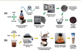
Fig. 1 Summary of the process of synthesis (a) and impregnation (b) of Fe $_{7}$ O $_{4}$  particles.
