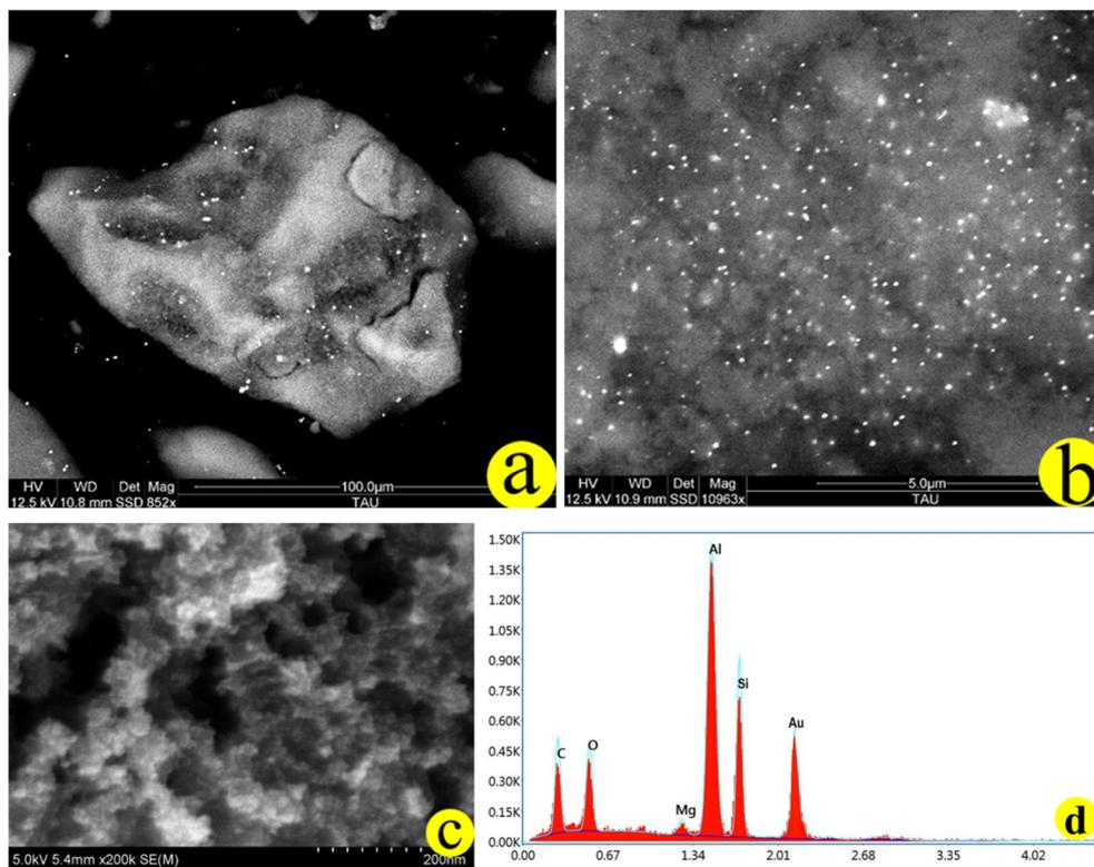
Fig. 2 SEM images of (a) the Au-AG composite showing preserved porous structure at low magnification, (b) higher magnification of the Au-AG composite revealing uniformly distributed Au nanoparticles, and (c) pristine (undoped) silica aerogel showing the mesoporous network structure in the absence of Au nanoparticles. (d) SEM-EDS spectrum of the Au-AG, showing elemental composition and peak intensities.
