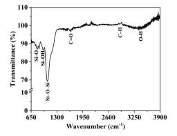
Fig. 4 FTIR spectrum of Au-AG composite from Supercritical Fluid Deposition (SFD). Peaks at  $\sim\!1050~\text{cm}^{-1}$  and  $\sim\!800~\text{cm}^{-1}$  confirm silical structure, while  $\sim\!3400~\text{cm}^{-1}$  and  $\sim\!1640~\text{cm}^{-1}$  indicate hydroxyls and adsorbed water. No Au–O–Si peaks confirm physical incorporation of gold nanoparticles without chemical bonding.
