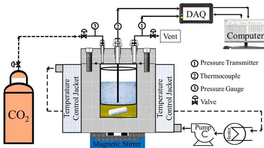
Fig. 1 Schematic diagram of the experimental setup used for the supercritical deposition of gold nanoparticles into the aerogel matrix.
