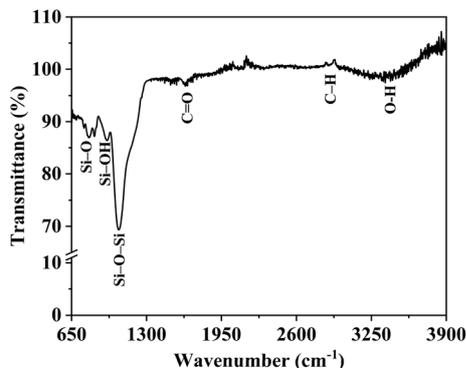
Fig. 4 FTIR spectrum of Au-AG composite from Supercritical Fluid Deposition (SFD). Peaks at  $\sim 1050\text{ cm}^{-1}$  and  $\sim 800\text{ cm}^{-1}$  confirm silica structure, while  $\sim 3400\text{ cm}^{-1}$  and  $\sim 1640\text{ cm}^{-1}$  indicate hydroxyls and adsorbed water. No Au–O–Si peaks confirm physical incorporation of gold nanoparticles without chemical bonding.
