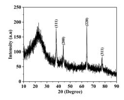
Fig. 3 XRD pattern of gold-doped silica aerogel synthesized by SFD, showing a broad peak at  $2\theta=20-30^\circ$  for amorphous silica and sharp peaks at 38.2°, 44.4°, 64.6°, and 77.5° indicating crystalline gold (fcc structure).
