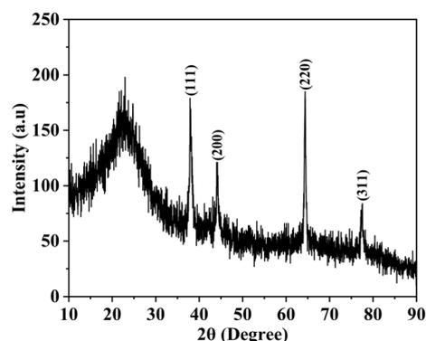
Fig. 3 XRD pattern of gold-doped silica aerogel synthesized by SFD, showing a broad peak at  $2\theta = 20\text{--}30^\circ$  for amorphous silica and sharp peaks at  $38.2^\circ$ ,  $44.4^\circ$ ,  $64.6^\circ$ , and  $77.5^\circ$  indicating crystalline gold (fcc structure).
