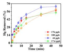
Fig. 6 Percentage removal of mercury (Hg) spiked in deionized water (ddH<sub>2</sub>O) by the Au-AG composite at varying concentrations, illustrating the composite's effectiveness in Hg adsorption over time.
