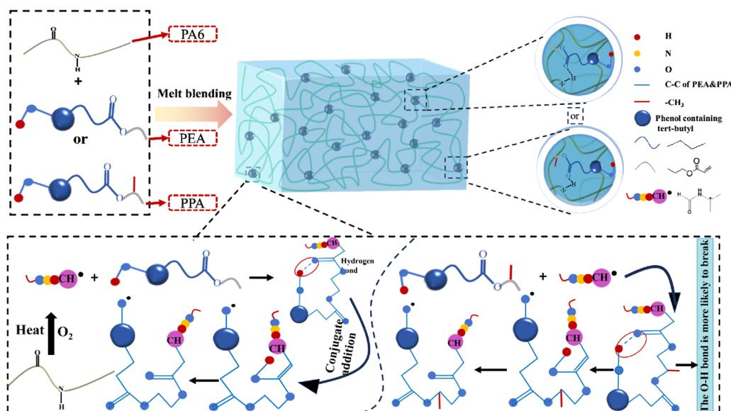
Fig. 6 Mechanism of resistance to thermal and oxygen aging of PEA and PPA.
