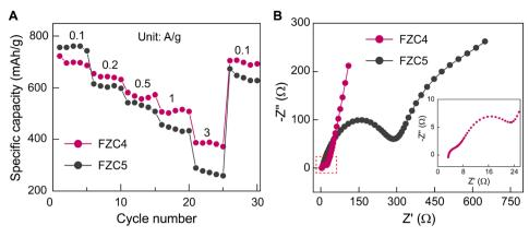
Fig. 7 (A) Rate capability tests across varying current densities ranging from 0.1–3 A g<sup>-1</sup> and (B) Nyquist plots of the FZC4 and FZC5 electrodes.
