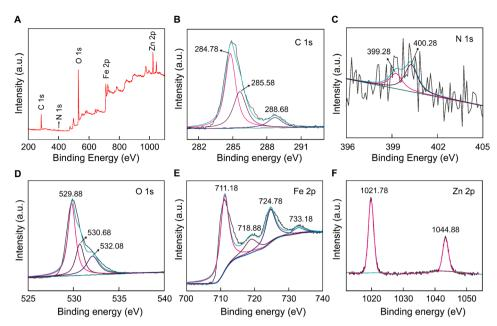
Fig. 5 XPS spectra: (A) survey, (B) C 1s, (C) N 1s, (D) O 1s, (E) Fe 2p and (F) Zn 2p of FZC4 nanocomposite.
