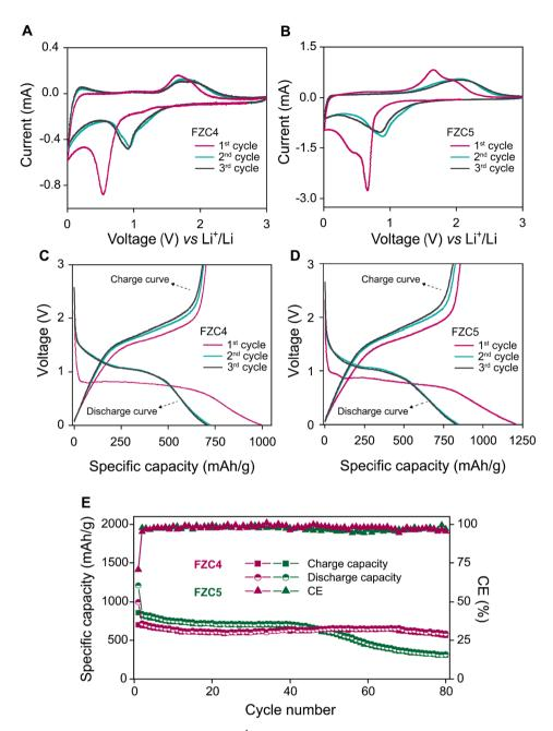
Fig. 6 (A and B) CV curves measured at a scan rate of 0.3 mV s $^{-1}$ . (C and D) GCD tests conducted at a current density of 0.1 A g $^{-1}$ . (E) Cycling performance evaluation at a current rate of 0.1 A g $^{-1}$  for FZC4 and FZC5.
