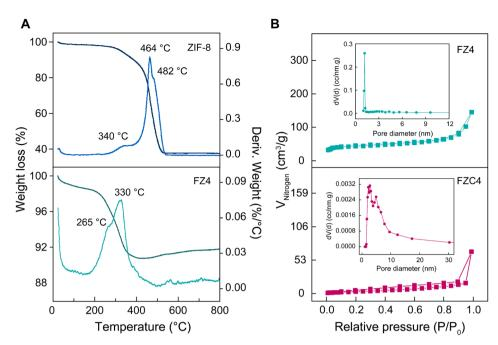
Fig. 2 (A) TGA-DTG curve of FZ4 and ZIF-8 in an air atmosphere. (B) Nitrogen adsorption—desorption isotherms and BJH (Barrett–Joyner–Halenda theory) adsorption dV/d log(D) pore size (insert) of FZ4 and FZC4 nanocomposites.
