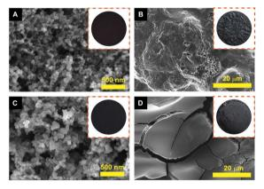
Fig. 8 SEM images and anode electrode photographs (insets) of the FZC4 electrode (A and B) and FZC5 electrode (C and D) before and after 100 cycles at 1 A  $\rm g^{-1}$ , respectively.
