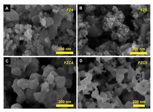
Fig. 3 FESEM images of (A) FZ4, (B) FZ5 and (C) FZC4 and (D) FZC5 nanocomposites
