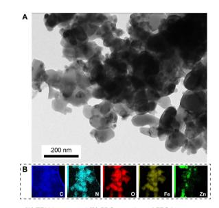
Fig. 4 (A) TEM image and (B) EDS mapping of FZC4 nanocomposite.
