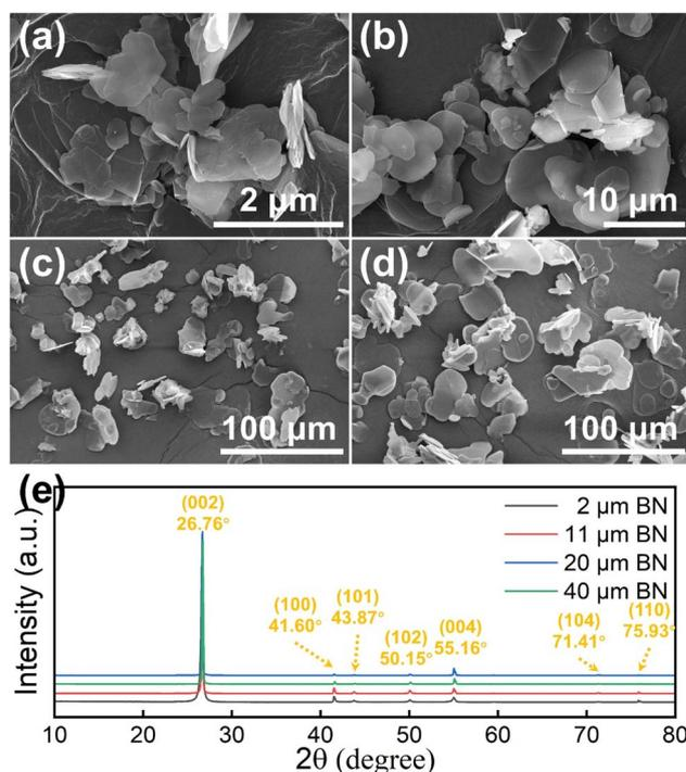
Fig. 2 SEM images of (a) 2 μm BN, (b) 11 μm BN, (c) 20 μm BN and (d) 40 μm BN. (e) XRD patterns of BN with different sizes.
