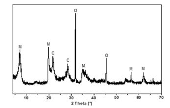
Fig. 15 XRD of catalyst before to reuse. M: montmorillonite, C: cristobalite, and O: iron oxide.
