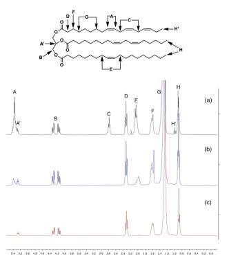
Fig. 9  $^{1}$ H NMR of (a) soybean oil, (b) hydrogenated soybean oil after 60 min at 70  $^{\circ}$ C, and (c) hydrogenated soybean oil after 120 min at 70  $^{\circ}$ C.
