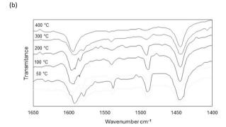
Fig. 6 FT-IR spectra of (a) Nat-Bent and (b) Bent-Pd-2 after pyridine desorption at different temperatures: 50 °C, 100 °C, 200 °C, 300 °C, and 400 °C.
