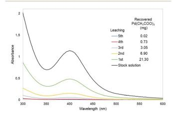
Fig. 1 UV-vis spectra of  $Pd(CH_3COO)_2$  solution after washing of **Bent-Pd-2**.
