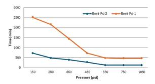
Fig. 11 Evolution of the hydrogenation reaction as the H<sub>2</sub> pressure is varied
