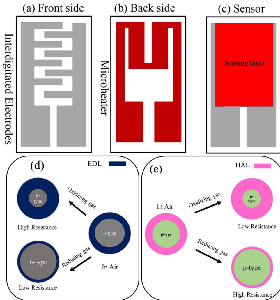
Fig. 1 Schematic of (a) the front side, (b) back side and (c) fabricated resistive gas sensor. General gas sensing mechanism of (d) n-type and (e) p-type gas sensors.
