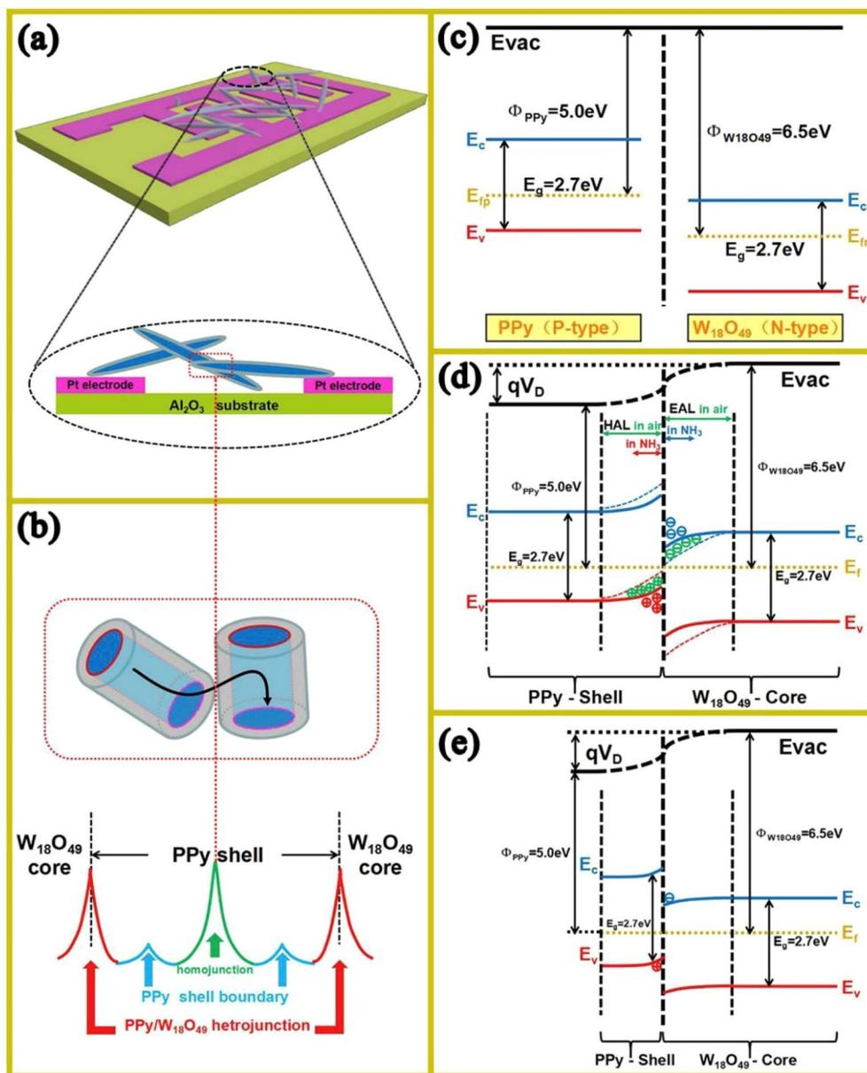
Fig. 17 (a) Schematic of the C-S NR sensor. (b) Various potential barriers in the PPy- $\text{W}_{18}\text{O}_{49}$  C-S NR sensor. (c) Energy band levels of the PPy- $\text{W}_{18}\text{O}_{49}$  C-S NRs before contact, (d) change in energy band upon exposure to  $\text{NH}_3$  and (e) influence of thinner PPy shell on the energy levels.<sup>99</sup> Reproduced with permission from ref. 99. Copyright 2017, Elsevier.
