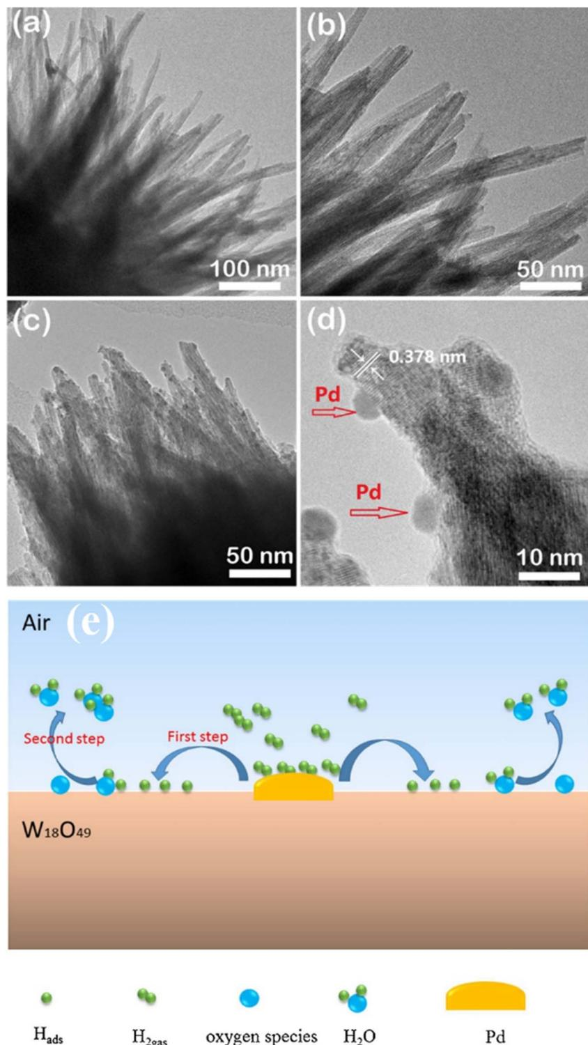
Fig. 8 TEM micrographs of (a) and (b)  $W_{18}O_{49}$  and (c) Pd- $W_{18}O_{49}$ . (d) HRTEM image of Pd- $W_{18}O_{49}$ . (e) Schematic of the spillover effect.<sup>63</sup> Reproduced with permission from ref. 63. Copyright 2018, Elsevier.
