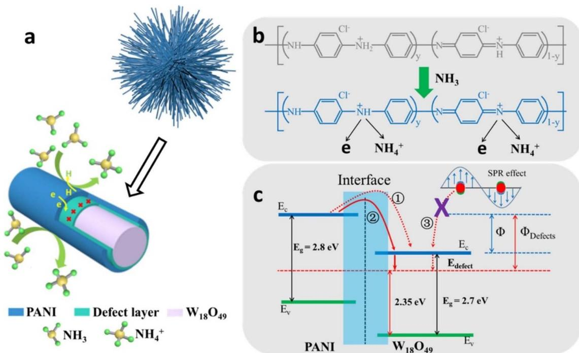
Fig. 22 (a) Schematic of  $W_{18}O_{49}$ -PANI C-S, (b) interaction of  $NH_3$  molecules with PANI and (c) heterojunction band structure and electron flow paths.<sup>110</sup> Reproduced with permission from ref. 110. Copyright 2020, Elsevier.
