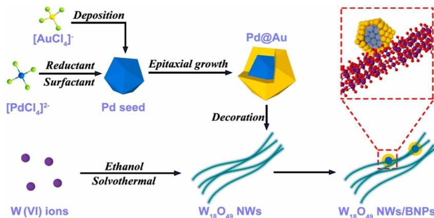
Fig. 10 Schematic representation of the synthesis of  $W_{18}O_{49}$  NWs and  $W_{18}O_{49}$  NWs/BNPs.<sup>68</sup> Reproduced with permission from ref. 68. Copyright 2022, Elsevier.
