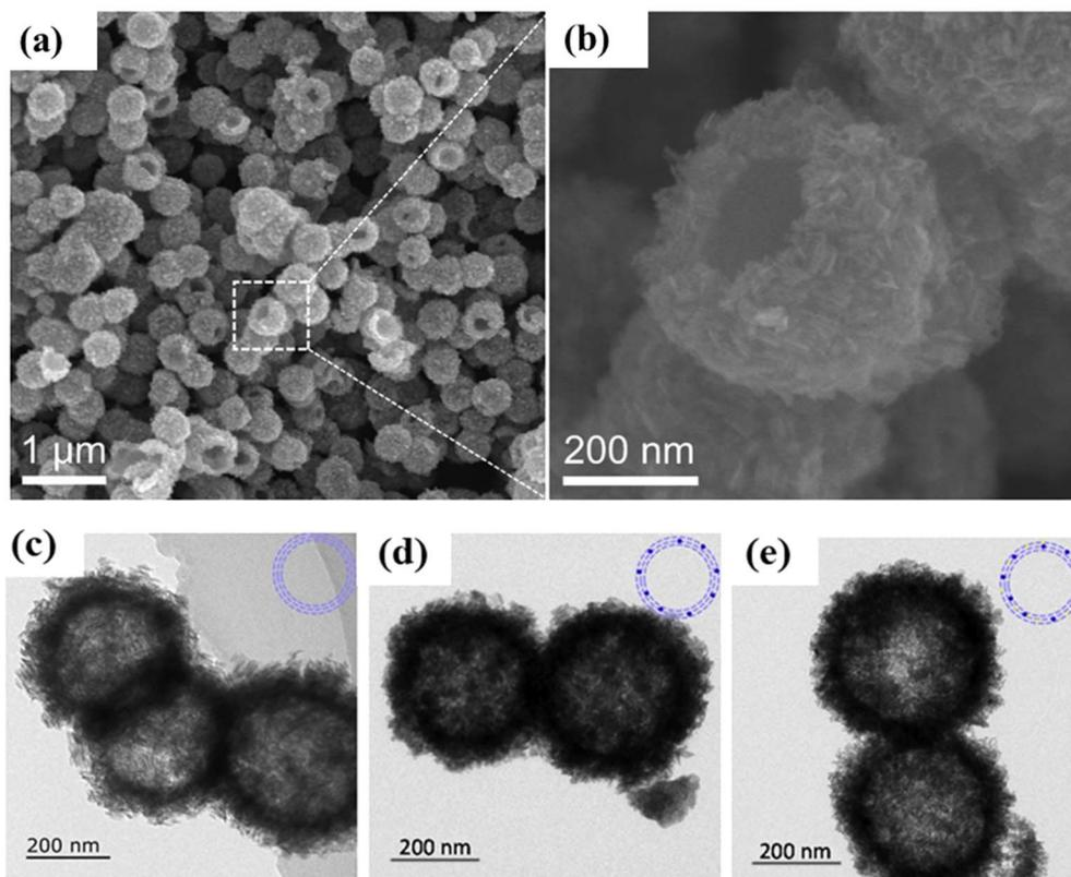
Fig. 12 (a) and (b) SEM micrographs of  $W_{18}O_{49}$  hollow spheres. TEM images of (c)  $W_{18}O_{49}$ , (d)  $Co_3O_4/W_{18}O_{49}$ , and (e) Au-decorated  $Co_3O_4/W_{18}O_{49}$  hollow spheres.<sup>69</sup> Reproduced with permission from ref. 69. Copyright 2019, Elsevier.
