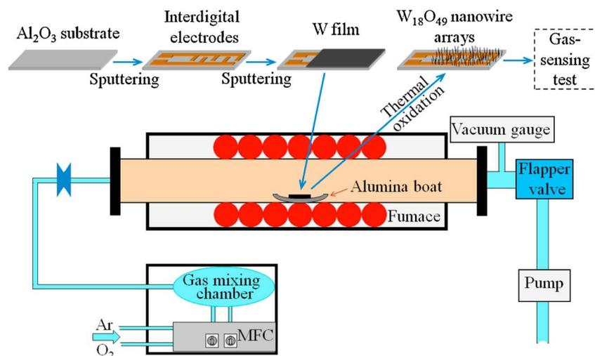
Fig. 5 Schematic of the synthesis of  $W_{18}O_{49}$  NW arrays.<sup>59</sup> Reproduced with permission from ref. 59. Copyright 2016, Elsevier.
