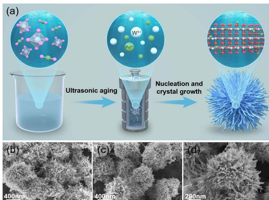
Fig. 7 (a) Synthesis procedure and SEM images of (a)  $W_{18}O_{49}$  nanoflowers and (b–d) Pd (20 mg)-decorated  $W_{18}O_{49}$  nanoflowers.<sup>61</sup> Reproduced with permission from ref. 61. Copyright 2023, Elsevier.
