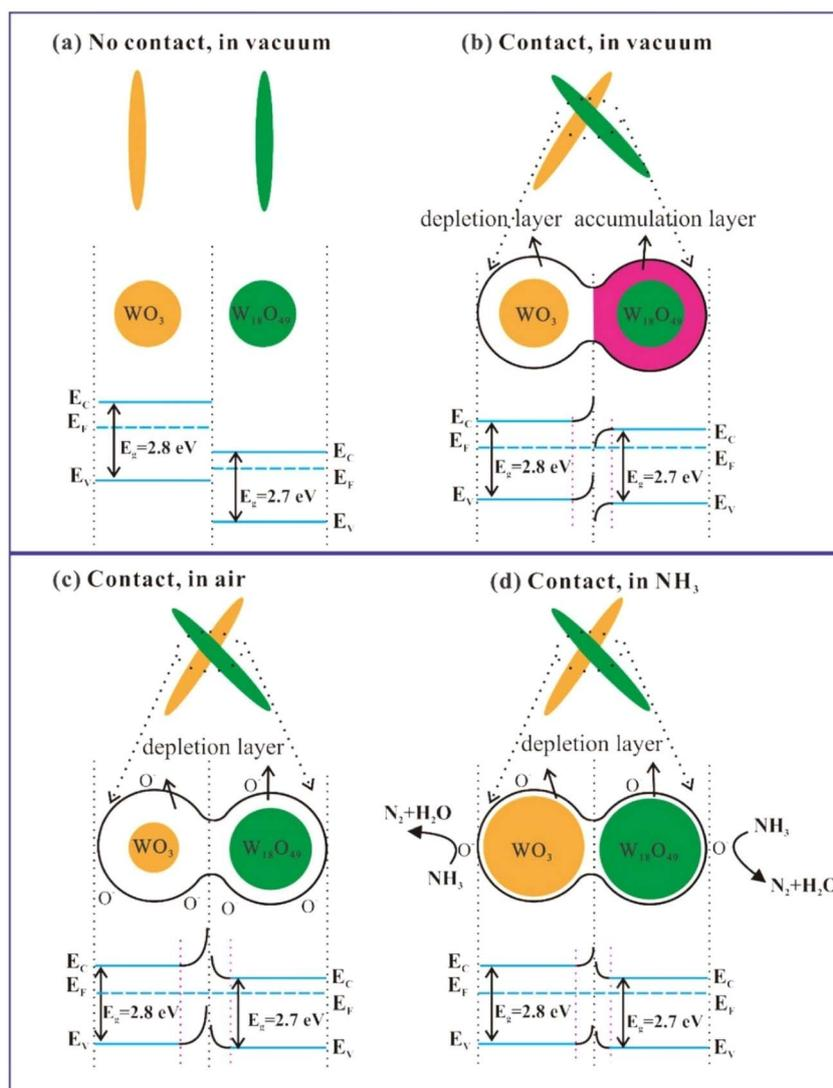
Fig. 20 Schematic of the energy band levels of  $\text{WO}_3$  and  $\text{W}_{18}\text{O}_{49}$  (a) before contact and after junction formation in (b) vacuum, (c) air and (d)  $\text{NH}_3$  gas.<sup>105</sup> Reproduced with permission from ref. 105. Copyright 2018, Elsevier.
