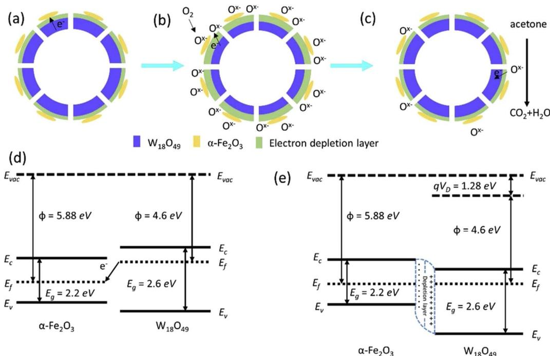
Fig. 21 Schematic of the  $W_{18}O_{49}/\alpha\text{-Fe}_2O_3$  hollow sphere (a) in vacuum, (b) in air and (c) in acetone. (d and e) Energy band diagram of the  $W_{18}O_{49}/\alpha\text{-Fe}_2O_3$  heterojunction before and after contact.<sup>108</sup> Reproduced with permission from ref. 108. Copyright 2019, Elsevier.
