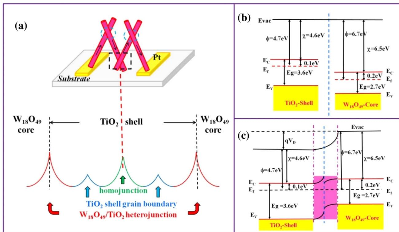
Fig. 18 (a) Schematic of the  $\text{W}_{18}\text{O}_{49}/\text{TiO}_2$  C-S NW gas sensor mechanism. Energy band levels of the  $\text{W}_{18}\text{O}_{49}/\text{TiO}_2$  C-S NW before (b) and after (c) contact.<sup>101</sup> Reproduced with permission from ref. 101. Copyright 2017, Elsevier.
