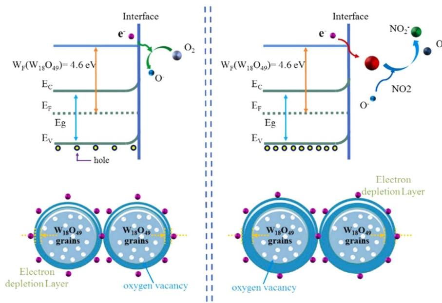
Fig. 3 Schematic of the  $NO_2$  gas sensing mechanism of  $W_{18}O_{49}$  nanoneedles.<sup>48</sup> Reproduced with permission from ref. 48. Copyright 2023, Elsevier.
