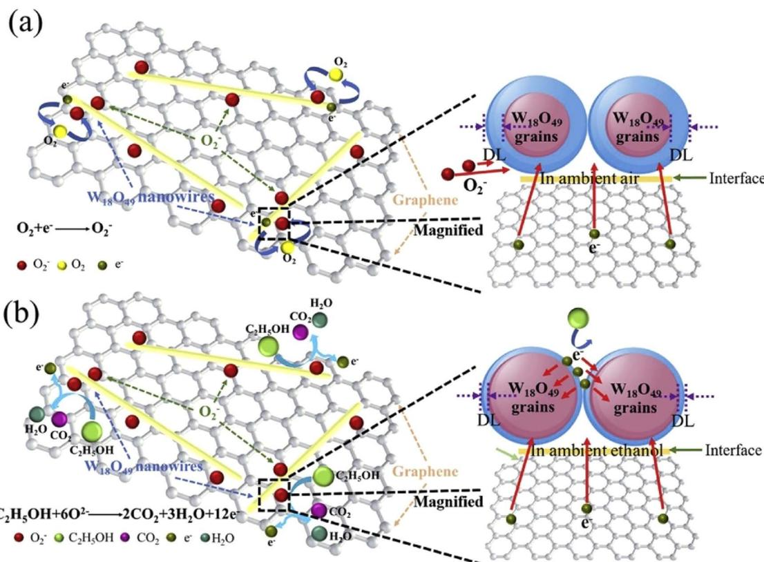
Fig. 16 (a) Schematic of the sensing mechanism of  $W_{18}O_{49}$ /graphene in air (b) and (c) ethanol.<sup>90</sup> Reproduced with permission from ref. 90. Copyright 2021, Elsevier.
