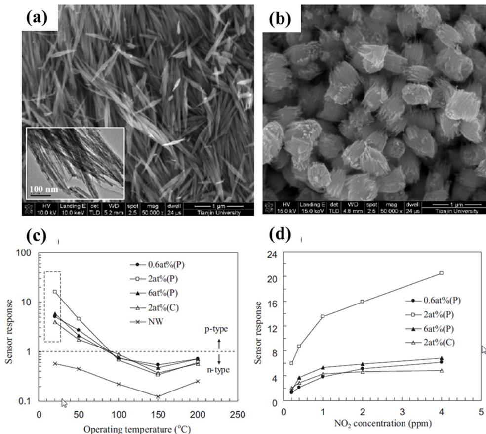
Fig. 15 SEM images of (a) pristine  $W_{18}O_{49}$  NWs and (b) Ti-added  $W_{18}O_{49}$  NWs prepared using a chemical synthesis method. (c) Sensor responses vs. temperature for pristine and Ti-added  $W_{18}O_{49}$  NWs to 2 ppm  $NO_2$  and (d) corresponding calibration curves.<sup>88</sup> P stands for physical impregnation and C stands for chemical addition of Ti. Reproduced with permission from ref. 88. Copyright 2012, Elsevier.
