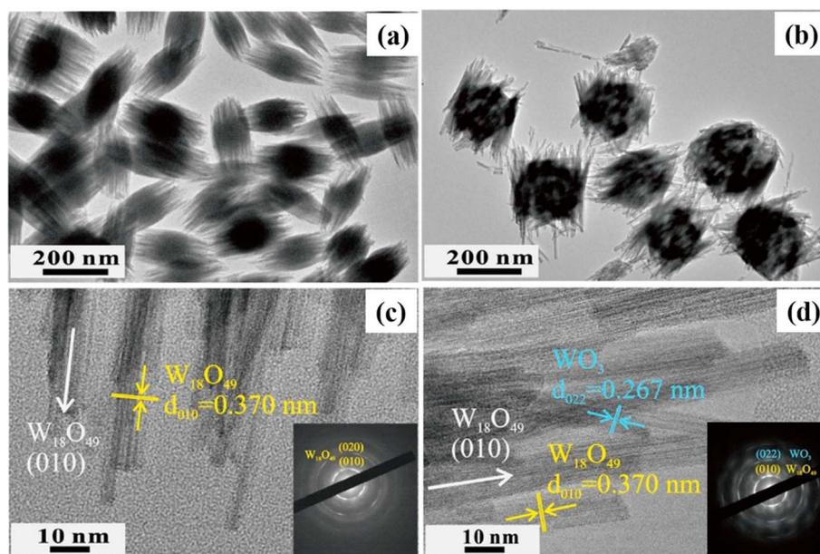
Fig. 19 TEM images of (a) the  $W_{18}O_{49}$  and (b)  $WO_3$ - $W_{18}O_{49}$  composites and HRTEM images of (c)  $W_{18}O_{49}$  and (d)  $WO_3$ - $W_{18}O_{49}$  composites (insets reveal the corresponding SAED patterns).<sup>105</sup> Reproduced with permission from ref. 105. Copyright 2018, Elsevier.
