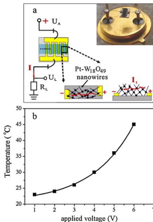
Fig. 9 (a) Schematic of the electrical set up for gas sensing measurement together with digital photo of the sensor. (b) Induced temperature of networked Pt–W<sub>18</sub>O<sub>49</sub> NW versus the applied voltage.<sup>65</sup> Reproduced with permission from ref. 65. Copyright 2011, Elsevier.
