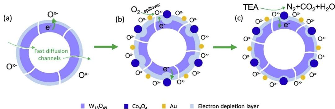
Fig. 13 Schematic of (a) pristine  $W_{18}O_{49}$  in air, (b) and (c) Au-decorated  $Co_3O_4/W_{18}O_{49}$  in air and TEA gas.<sup>70</sup> Reproduced with permission from ref. 70. Copyright 2019, Elsevier.
