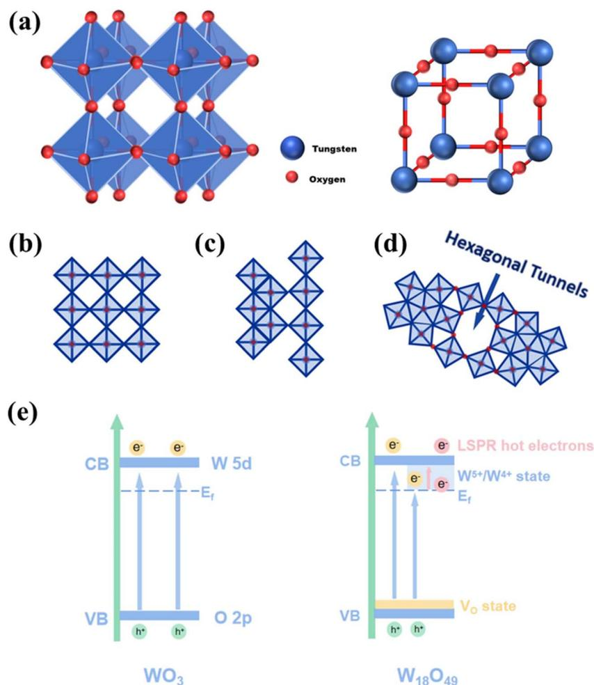
Fig. 2 (a) Structure of  $WO_3$ . (b) Corner- and (c) edge-sharing modes. (d) Pentagonal column mode. (e) Electronic band structure of  $WO_3$  and  $W_{18}O_{49}$ .<sup>44</sup> Reproduced with permission from ref. 34. Copyright 2023, Elsevier.
