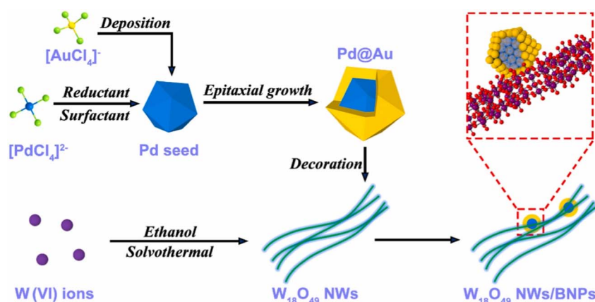
Fig. 10 Schematic representation of the synthesis of W_{18}O_{49} NWs and W_{18}O_{49} NWs/BNPs. 68 Reproduced with permission from ref. 68. Copyright 2022, Elsevier.
