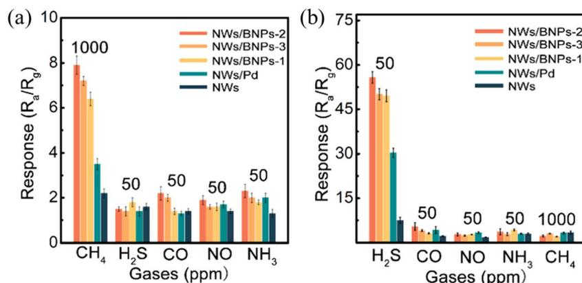
Fig. 11 Selectivity of  $W_{18}O_{49}$  NWs/BNPs-2 at (a)  $320$  °C and (b)  $100$  °C to various gases.<sup>68</sup> Reproduced with permission from ref. 68. Copyright 2022, Elsevier.
