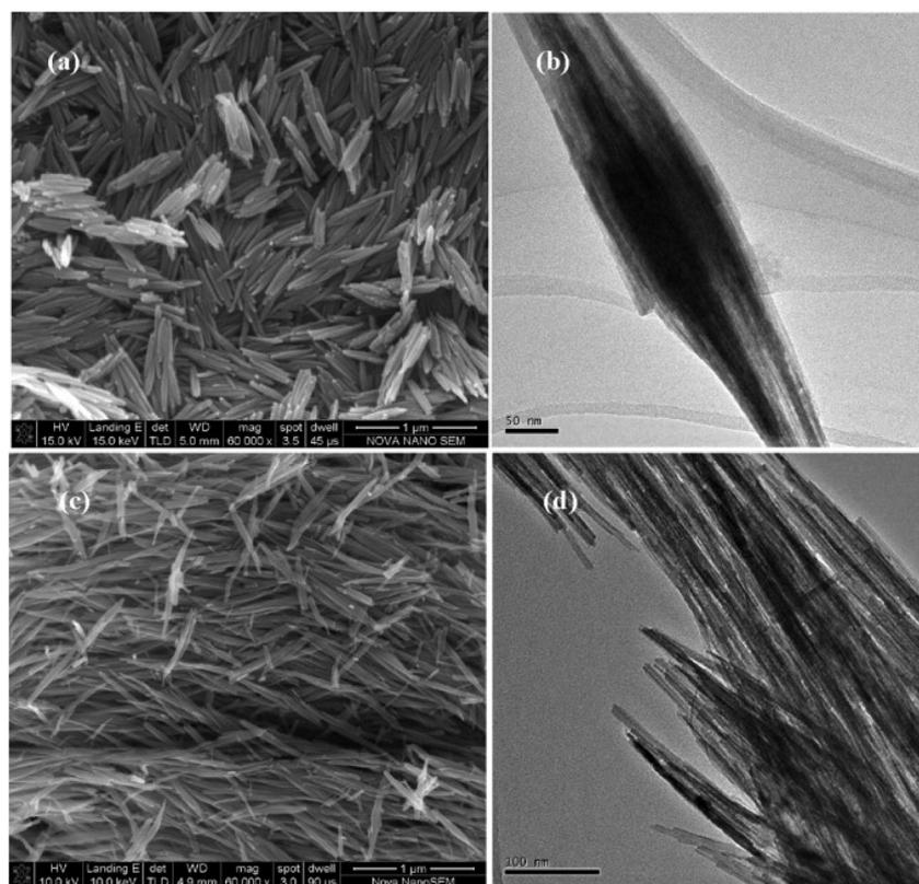
Fig. 4 SEM and TEM micrographs of the  $\text{W}_{18}\text{O}_{49}$  (a) and (b) NRs and (c) and (d) NWs.<sup>57</sup> Reproduced with permission from ref. 57. Copyright 2011, Elsevier.
