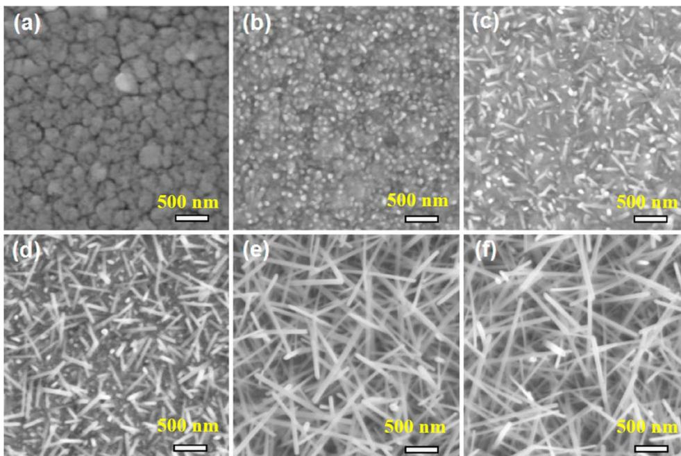
Fig. 6 SEM micrographs of  $W_{18}O_{49}$  grown at  $650\text{ }^{\circ}\text{C}$  for various oxidation times under (a) no oxygen and oxygen flow time for (b) 10, (c) 20, (d) 40 and (e) 60 min and (f) in  $Ar/O_2$  flow during growth.<sup>59</sup> Reproduced with permission from ref. 59. Copyright 2016, Elsevier.
