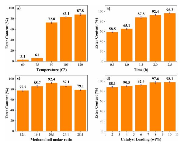
Fig. 7 Influence of (a) reaction temperature, (b) reaction time, (c) MeOH: oil molar ratio and (d) catalyst concentration on ester content
