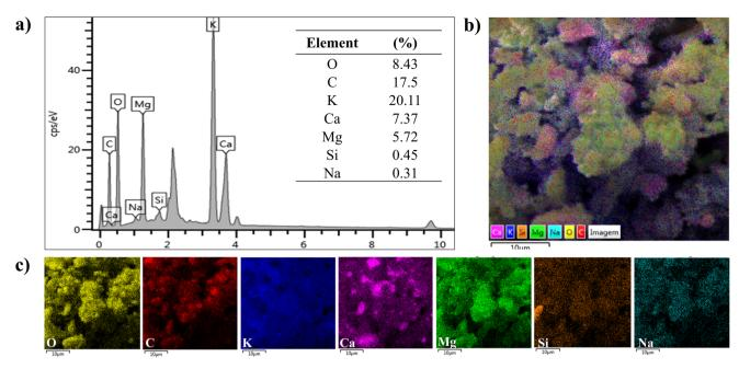
Fig. 12 (a) EDS spectrum, (b) and (c) surface elemental mapping of BHA400/3-R catalyst
