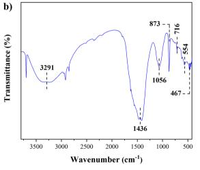
Fig. 11 (a) XRD pattern and (b) FT-IR spectrum of BHA400/3-R catalyst.
