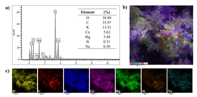
Fig. 5 (a) EDS spectrum, (b) and (c) surface elemental mapping of BHA400/3 catalyst
