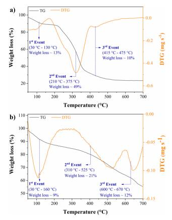
Fig. 6 TG/DTG curves of (a) RBBH and the (b) BHA400/3 catalyst.
