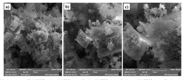
SEM micrographs of BHA400/3 catalyst (a) 1000× magnification, (b) 2500× magnification and (c) 5000× magnification.
