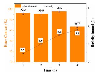
Fig. 2 Evaluation of the influence of calcination time on catalytic activity for biodiesel production and the basicity of synthesized catalysts.
