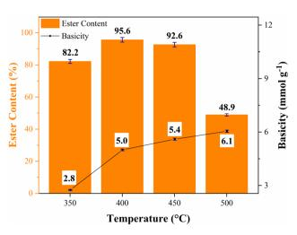
Fig. 1 Evaluation of the influence of calcination temperature on catalytic activity for biodiesel production and the basicity of synthesized catalysts.
