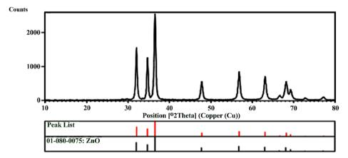
Fig. 5 XRD pattern of the ZnO NPs.
