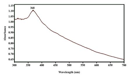
Fig. 3 UV-vis analysis of the ZnO NPs.
