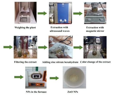
Fig. 1 The preparation steps of ZnO NPs.
