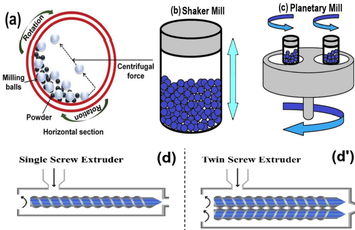
Fig. 1 Schematic representation of (a) ball milling process, (b) Shaker Mill, (c) Planetary Mill, (d) and (d') Single and Twin-Screw Extruder. Reproduced from ref. 68–70 with permission from [Wiely], copyright [2024].
