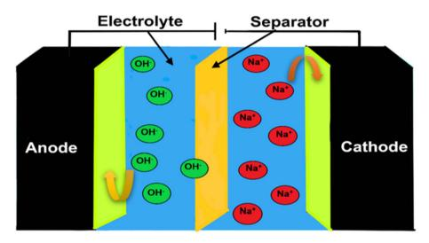
Fig. 8 The mechanism structure of pseudocapacitance. Reproduced from ref. 288 with permission from [Royal Society of Chemistry], copyright [2021].
