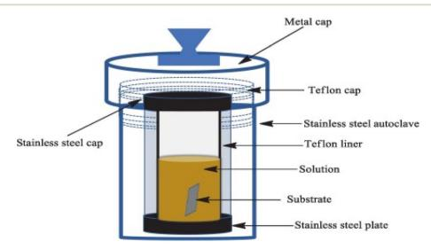
Fig. 3 Schematic of solvothermal technique's equipment. Reproduced from ref. 99 with permission from [Elsevier], copyright [2023].
