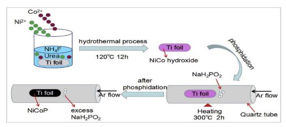
Fig. 5 Phosphorization process for synthesizing NiCoP by NaH<sub>2</sub>PO<sub>2</sub>. Reproduced from ref. 128 with permission from [Elsevier], copyright [2019].
