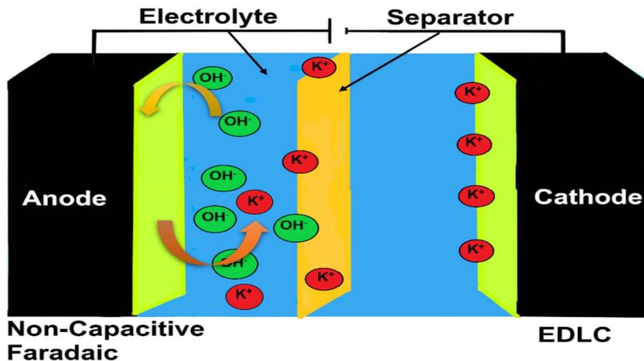
Fig. 9 The structure of hybrid supercapacitors, Reproduced from ref. 288 with permission from [Royal Society of Chemistry], copyright [2021].
