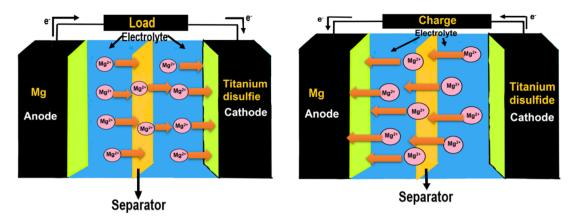
Fig. 11 Ion transport in batteries, Reproduced from ref. 301 with permission from [Nature], copyright [2021].
