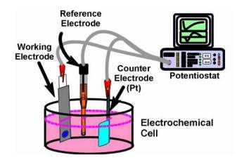
Fig. 2 Schematic of electrodeposition process in three-electrode system. Reproduced from ref. 88 with permission from [IOP Science], copyright [2008].
