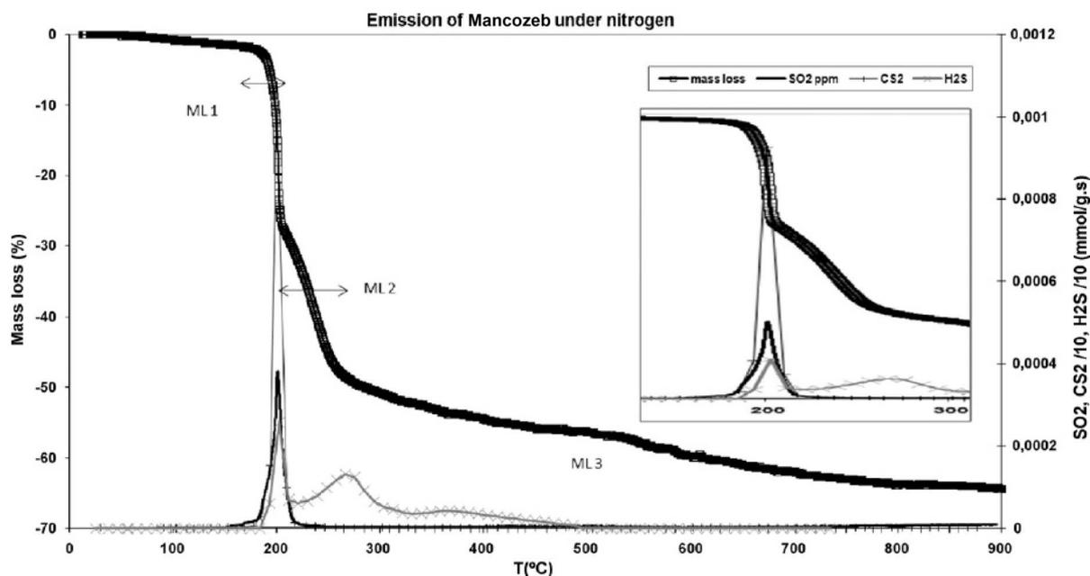
Fig. 2 TG curve and emissions of  $\text{SO}_2$ ,  $\text{H}_2\text{S}$  and  $\text{CS}_2$  per gram of the product during pyrolysis of technical mancozeb ( $5\text{ }^\circ\text{C min}^{-1}$ ).<sup>27</sup>
