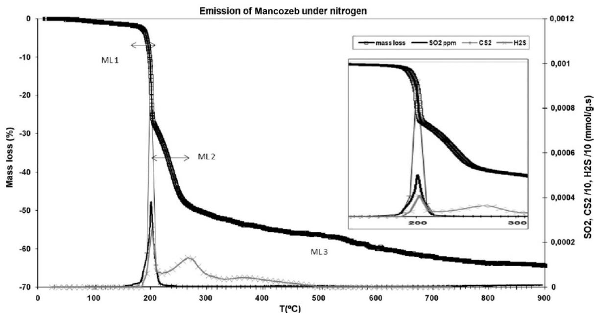
Fig. 2 TG curve and emissions of  $\text{SO}_2$ ,  $\text{H}_2\text{S}$  and  $\text{CS}_2$  per gram of the product during pyrolysis of technical mancozeb ( $5\text{ °C min}^{-1}$ ).<sup>27</sup>
