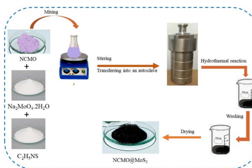
Fig. 2 A graphical illustration of the synthesis of NCMO@ \text{MoS}_2 nanocomposite.
