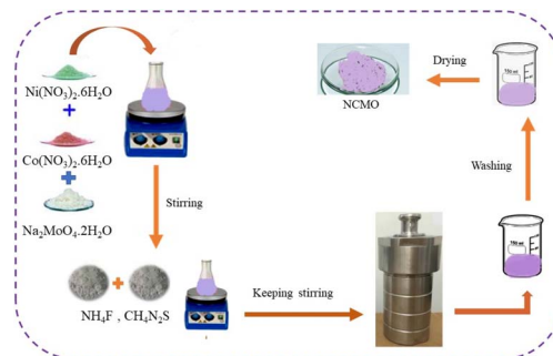
Fig. 1 A graphical illustration of the synthesis of spinel-nanostructured NCMO.
