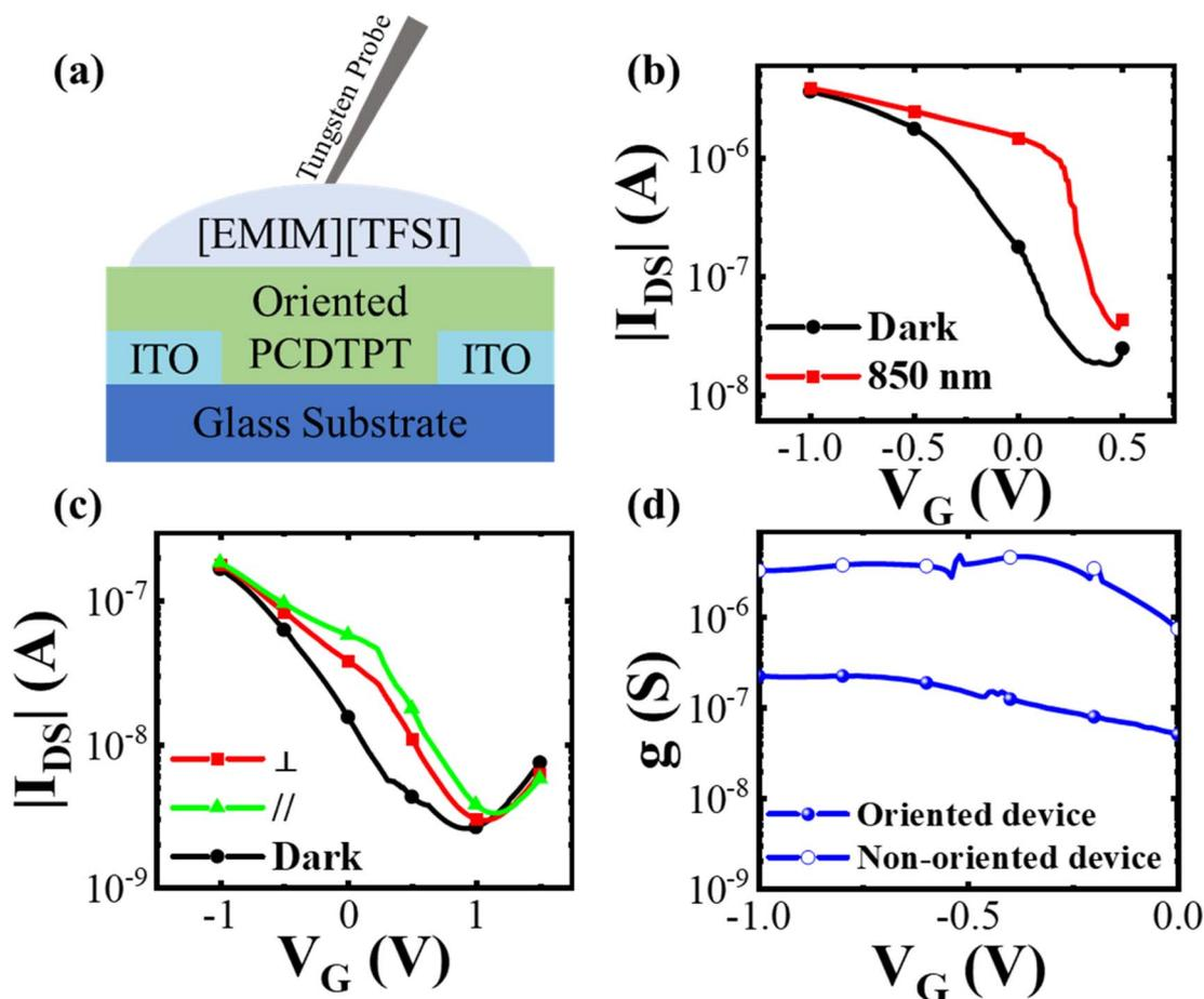
Fig. 3 (a) Schematic of the OECP device structure. Transfer curves of (b) the non-oriented device and (c) the oriented device, with  $V_{DS} = -0.8$  V under a constant  $1 \text{ mW cm}^{-2}$  incident light intensity at 850 nm. (d) Comparison of transconductances values between the two device types.
