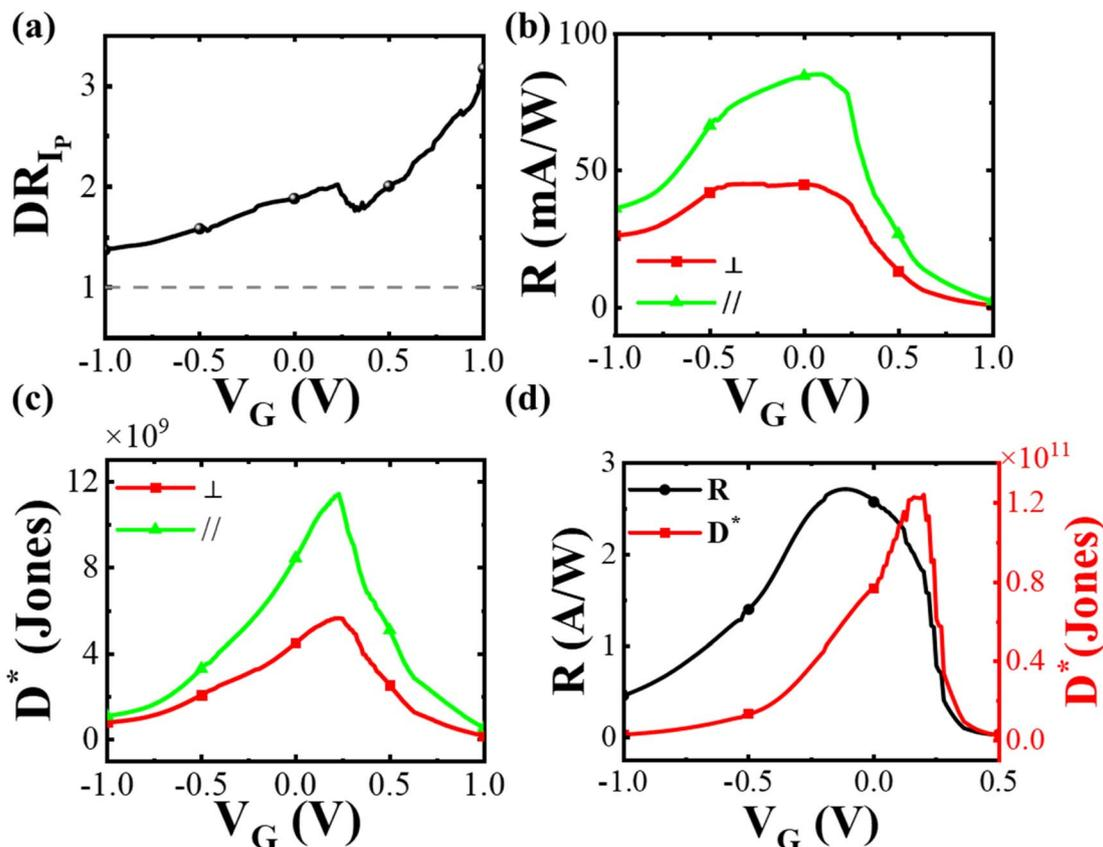
Fig. 4 (a) Photogenerated current dichroic ratio ( $DR_{I_p}$ ), (b) responsivity ( $R$ ), and (c) normalized detectivity ( $D^*$ ) of the oriented device. (d) Corresponding optoelectronic performance parameters for the non-oriented device.
