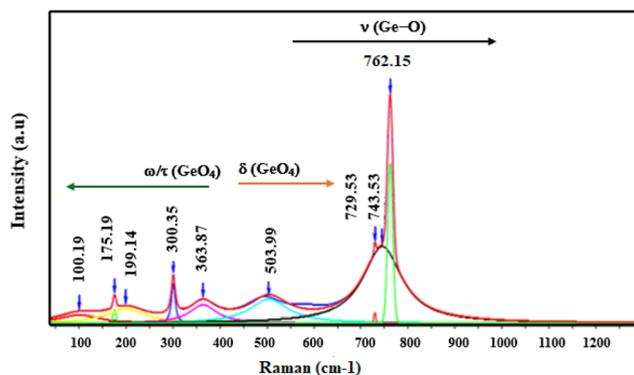
Fig. 4 The Raman spectrum of  $\text{Li}_4\text{GeO}_4$  at room temperature.
