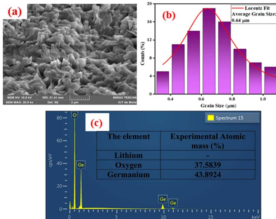
Fig. 3 (a) SEM image of title compound; (b) grain size distribution histogram and (c) the elemental analysis by EDX.
