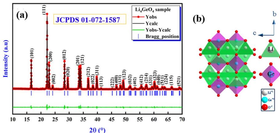
Fig. 2 (a) The Rietveld refinement was performed on the X-ray powder diffraction pattern of  $\text{Li}_4\text{GeO}_4$  that was sintered at  $800^\circ\text{C}$ , and (b) the crystal structural of  $\text{Li}_4\text{GeO}_4$ .
