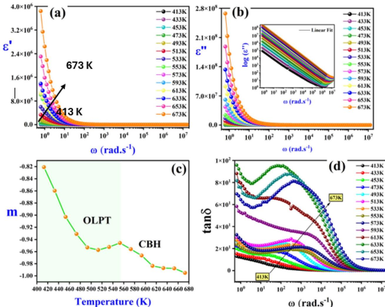
Fig. 7 (a) Frequency dependence of the dielectric constant ( $\epsilon'$ ). (b) Variation of the imaginary part ( $\epsilon''$ ) as a function of frequency, fitted using the universal power law as shown in eqn (7) (inset of figure). (c) Variation of the exponent  $m(T)$  as a function of temperature. (d) Frequency dependence of the loss factor.
