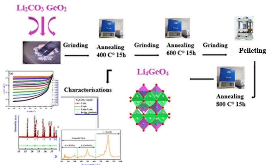
Fig. 1 Schematic representation of the  $\text{Li}_4\text{GeO}_4$  synthesis via the solid-state method.
