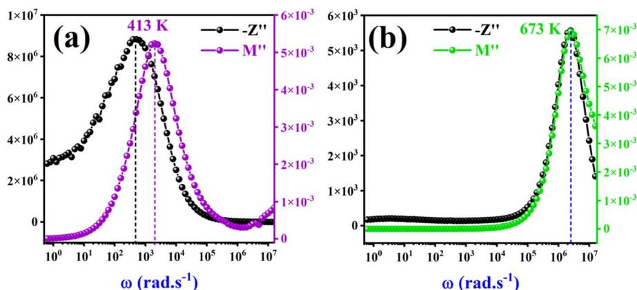
Fig. 9 Variation of  $-Z''$  and  $M''$  as a function of frequency at 413 K (a) and 673 K (b).
