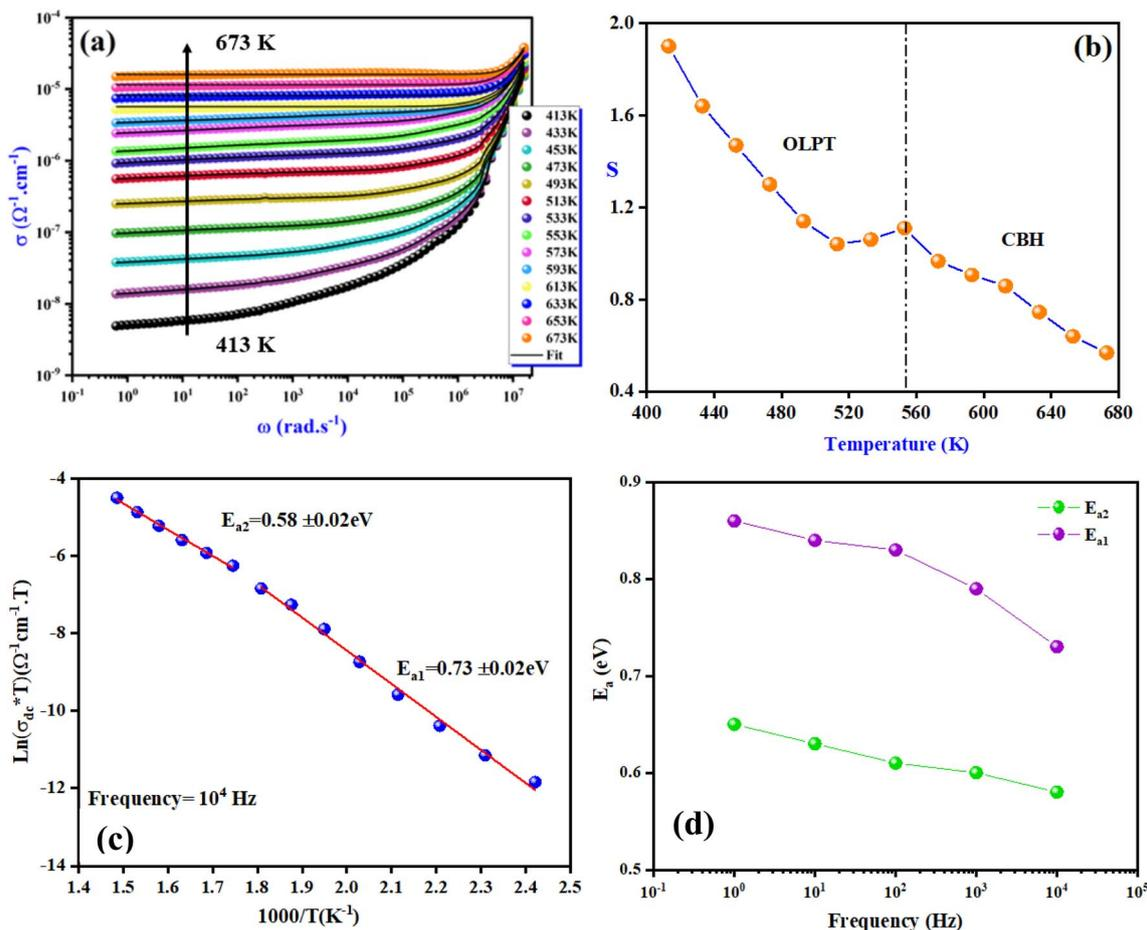
Fig. 6 (a) The variation of the AC conductivity as a function of frequency at various temperatures for  $\text{Li}_4\text{GeO}_4$ . Solid lines connecting the data points illustrate the fitting of the AC conductivity data using Jonscher's power law (eqn (5)). (b) The power exponent ( $S$ ), (c) the variation of  $\ln(\sigma_{\text{dc}} \times T)$  as a function of the inverse temperature at a frequency of  $10^4$  Hz, and (d) the variation of the activation energy as a function of frequency.
