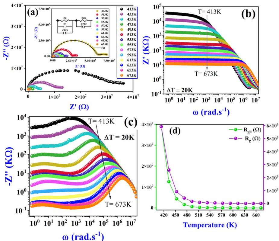
Fig. 5 (a) The  $-Z''$  vs.  $Z'$  curves at various temperatures for  $\text{Li}_4\text{GeO}_4$ , the solid lines associating the data points are adjusted curves employing an equivalent circuit model, as depicted in the respective inset. (b) Real ( $Z'$ ) and (c) imaginary ( $-Z''$ ) parts of the complex impedance of  $\text{Li}_4\text{GeO}_4$  as functions of angular frequency. (d) Variation of  $R_g$  (grain resistance) and  $R_{gb}$  (grain boundary resistance) as a function of temperature.
