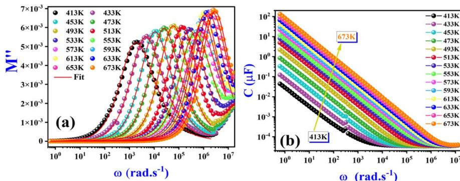
Fig. 8 (a) Variation of the imaginary part of the electric module as a function of frequency. (b) Frequency-dependent capacitance spectra.
