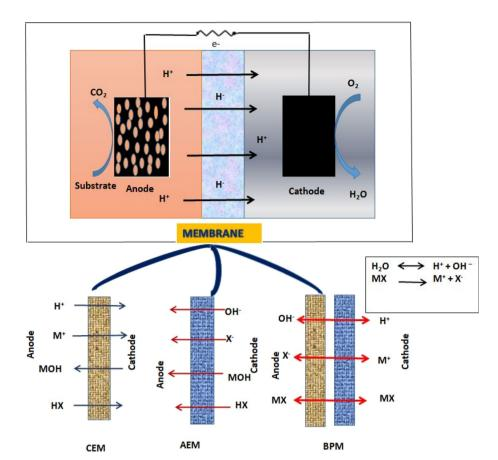
Fig. 2 Dual chambered MFC system with anode, cathode and membrane.
