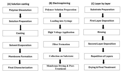
Fig. 4 Schematic diagram of (A) solution casting, (b) electrospinning, (c) layer by layer.
