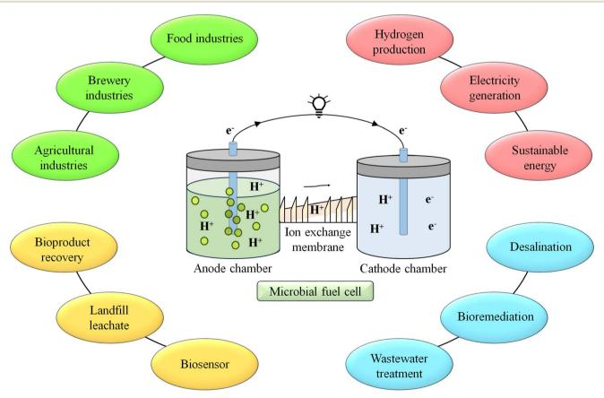
Fig. 1 Application of MFC in various fields.
