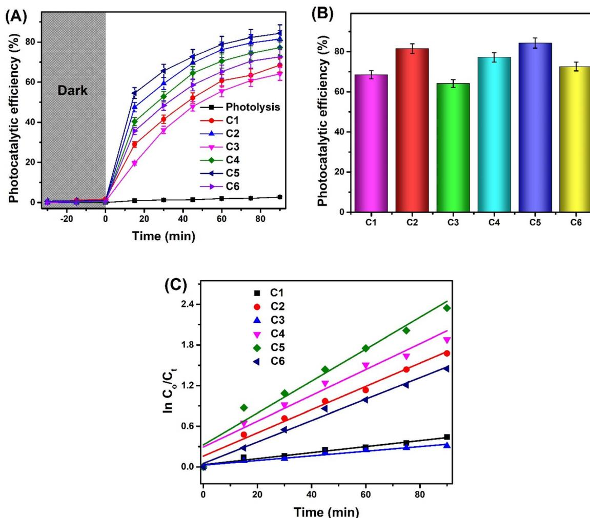
Fig. 2 (A) Photocatalytic efficiency of a synthesized complexes for the removal of DCF as a function of light irradiation time, (B) comparative photocatalytic efficiency, and (C) reaction kinetics of synthesized complexes.
