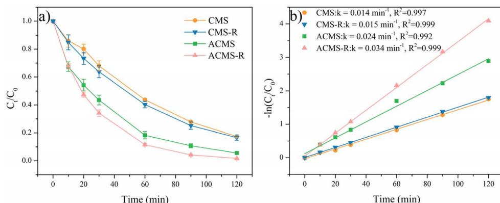
Fig. 5 (a) RhB degradation in PMS activated with the CMS, CMS-R, ACMS, and ACMS-R as catalysts, respectively; (b) corresponding fitted kinetics curves. Experimental conditions:  $[\text{RhB}]_0 = 50 \text{ mg L}^{-1}$ ,  $[\text{catalyst}] = 800 \text{ mg L}^{-1}$ ,  $[\text{PMS}] = 400 \text{ mg L}^{-1}$ ,  $\text{pH}_0 = 7$ ,  $T = 25 \text{ }^\circ\text{C}$ .
