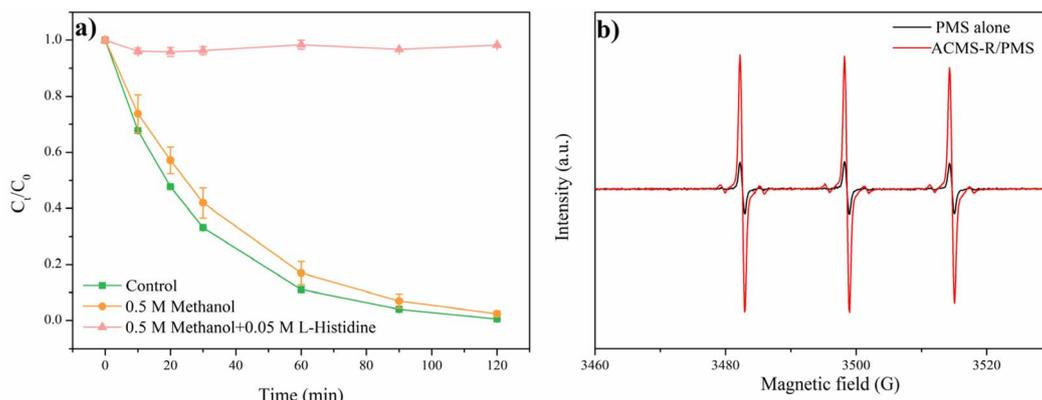
Fig. 7 (a) Quenching experiments with ACMS-R as the catalyst. Experimental conditions: [catalyst] = 800 mg L<sup>-1</sup>, [PMS] = 800 mg L<sup>-1</sup>, [RhB]<sub>0</sub> = 50 mg L<sup>-1</sup>, pH = 7, T = 25 °C, [methanol] = 0.5 M, [L-histidine] = 0.05 M. (b) EPR measurements of the ACMS-R/PMS system with TEMP as the spin-trapping agent.
