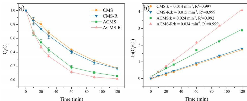
Fig. 5 (a) RhB degradation in PMS activated with the CMS, CMS-R, ACMS, and ACMS-R as catalysts, respectively; (b) corresponding fitted kinetics curves. Experimental conditions: [RhB]<sub>0</sub> = 50 mg L<sup>-1</sup>, [catalyst] = 800 mg L<sup>-1</sup>, [PMS] = 400 mg L<sup>-1</sup>, pH<sub>0</sub> = 7, T = 25 °C.
