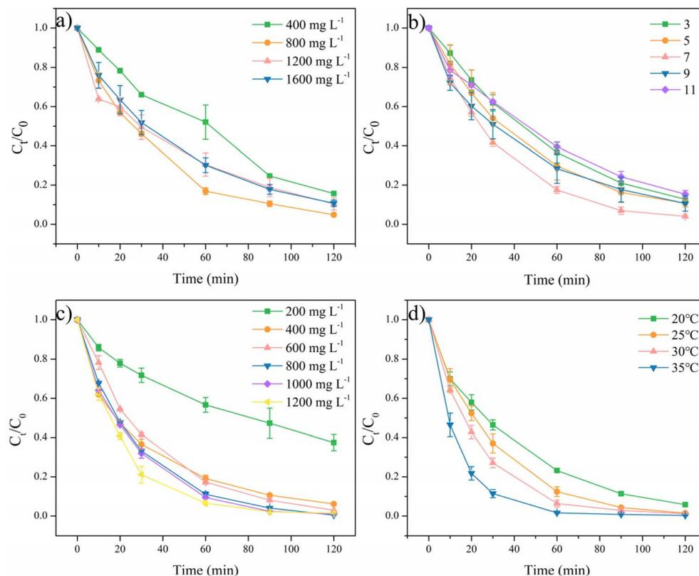
Fig. 6 Effects of the (a) catalyst dosage, (b) pH, (c) PMS concentration, and (d) temperature. Experimental conditions:  $[RhB]_0 = 50 \text{ mg L}^{-1}$ ,  $[catalyst] = 800 \text{ mg L}^{-1}$  (for b, c, and d),  $[PMS] = 400 \text{ mg L}^{-1}$  (for a and c) and  $800 \text{ mg L}^{-1}$  for d,  $pH_0 = 7$  (for a, b, and d),  $T = 25^\circ \text{C}$  (for a, b, and c).
