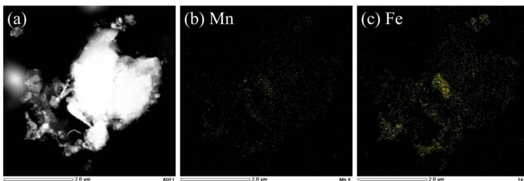
Fig. 2 (a)–(c) EDS elemental mapping images of ACMS-R.
