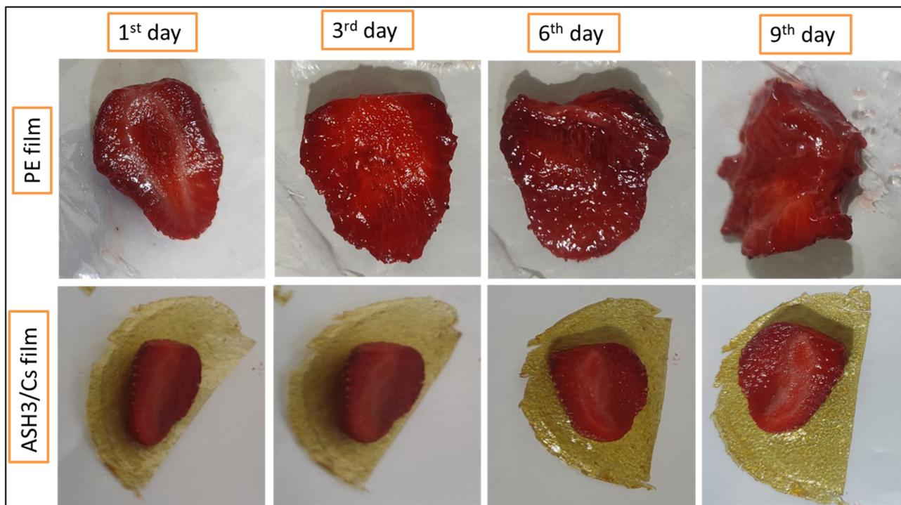
Fig. 14 Visual inspection of fresh-cut strawberries after wrapping with PE film and ASH3/Cs films at 1, 3, 6, and 9 day of storage at 25 °C and 65% of humidity.
