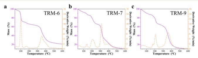
Fig. 7 (a-c) TG and DTG curves of TRM-6. TRM-7 and TRM-9.
