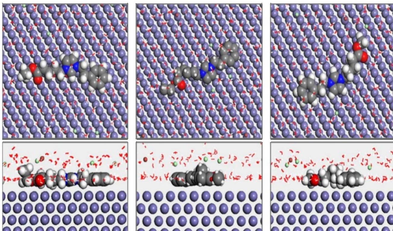
Fig. 4 Top and side views of the equilibrium adsorption geometries of the examined inhibitors on the Fe (110) surface after the MD process.
