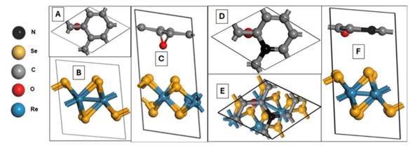
Fig. 11 Optimized geometries of (A) GO sheet, (B) ReSe<sub>2</sub> structure, (C) GO/ReSe<sub>2</sub> heterostructure, (D) N-rGO sheet, (E) top-view of N-rGO/ ReSe<sub>2</sub> heterostructure and (F) side-view of N-rGO/ReSe<sub>2</sub> heterostructure. The red, black, grey, blue and gold represent the following atoms, oxygen, nitrogen, carbon, rhenium and selenium, respectively.
