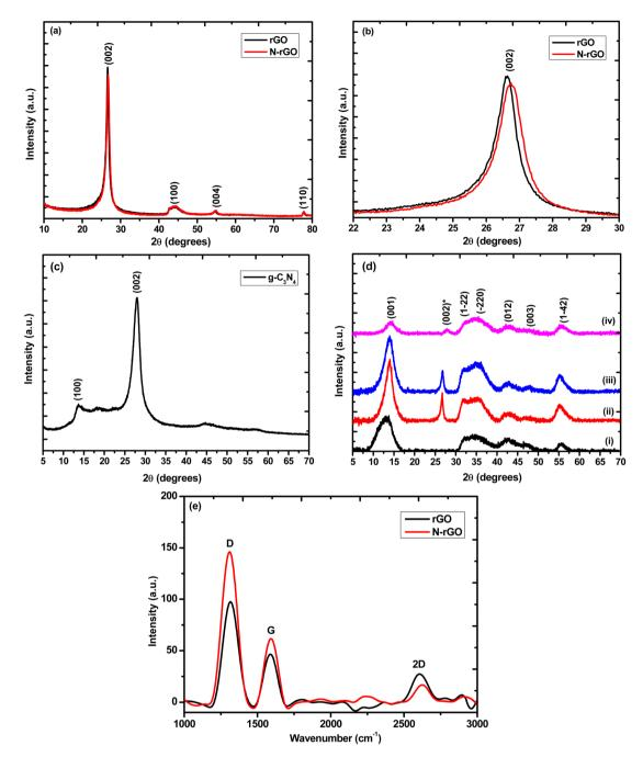
Fig. 1 PXRD patterns of (a) rGO and N-rGO. (b) PXRD shows the shift of the (002) in rGO and N-rGO. (c) The PXRD pattern of  $g-C_3N_4$  (d) PXRD pattern of (i) pristine ReSe<sub>2</sub>, (ii) ReSe<sub>2</sub>-rGO, (iii) ReSe<sub>2</sub>-N-rGO, and (iv) ReSe<sub>2</sub>-g-C<sub>3</sub>N<sub>4</sub>. (e) Raman spectra of rGO and N-rGO.
