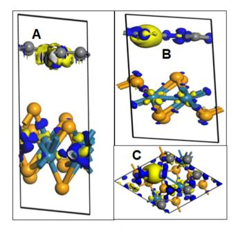
Fig. 12 The three-dimensional (3D) charge density differences of (A) ReSe<sub>2</sub>-rGO heterostructure, (B) side view of ReSe<sub>2</sub>-N-rGO heterostructure and (C) top view of ReSe2-N-rGO heterostructure. The yellow and blue colours represent the accumulation and depletion of electrons, respectively.
