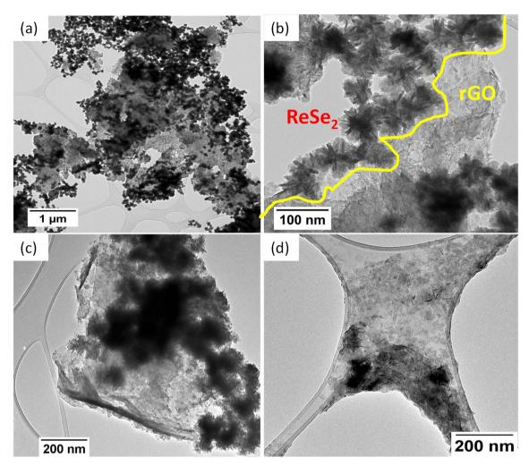
Fig. 6 (a) Formation of the ReSe<sub>2</sub>-rGO after selenization. (b) Interface between the ReSe<sub>2</sub> and the rGO. (c) Formation of ReSe<sub>2</sub>-N-rGO after selenization. (d) Formation of ReSe<sub>2</sub>-q- $C_3N_4$  after selenization.
