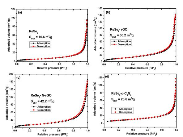
Fig. 9 Adsorption-desorption isotherms of (a) ReSe<sub>2</sub>, (b) ReSe<sub>2</sub>-rGO, (c) ReSe<sub>2</sub>-N-rGO, and (d) ReSe<sub>2</sub>-g-C<sub>3</sub>N<sub>4</sub>.
