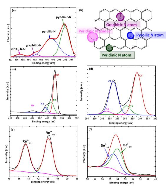
Fig. 2 (a) Deconvoluted XPS spectrum of the N1s peak for N-rGO. (b) Graphical representation of the types of nitrogen defects introduced. (c) Deconvoluted N1s peak of g- $C_3N_4$ . (d) Deconvoluted C1s peak of g- $C_3N_4$ . (e) High-resolution XPS spectrum of Se.
