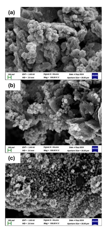
Fig. 7 SEM images of (a) ReSe $_2$ -rGO, (b) ReSe $_2$ -N-rGO, and (c) ReSe $_2$ -g-C $_3$ N $_4$ .
