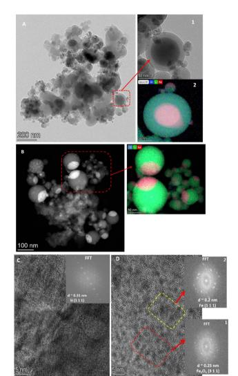
Fig. 6 HR-TEM images of the shocked M3 sample. (A) Spherical grains with dense cores and less dense shells; (B) HAADF image highlighting high Z-value cores and low Z-value shells; (C) nanocrystalline Si; and (D) polycrystalline phases with magnetite (311) in red and Fe (111) in yellow.
