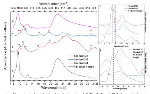
Fig. 1 ATR-FTIR spectra of the unshocked sample (A) and shocked samples of M1 (B), M2 (C), and M3 (D). Inset 1 highlights the red shift observed in the Si-O stretching vibration region for the shocked M1 and M2 samples compared to their unshocked counterparts. Inset 2 illustrates the red shift in the O-Si-O bending vibration region for the shocked M1 and M2 samples relative to their unshocked counterparts.
