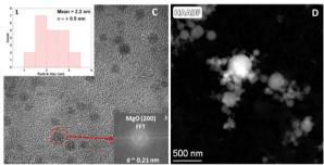
Fig. 4 HR-TEM images of the shocked M1 samples: (A) large spherical grains, (B) polycrystalline forsterite, (C) MgO quantum dots, and (D) HAADF image of the distinctive large grains.
