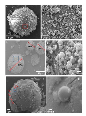
Fig. 3 FE SEM images of the shocked samples of M1 (A and B), M2 (C and D) and M3 (E and F)
