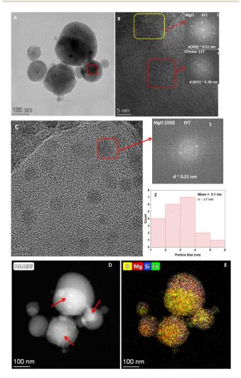
Fig. 5 HR-TEM images of the shocked M2 sample: (A) large spherical grains; (B) presence of MgO and olivine within the area marked by a red square in (A); (C) MgO quantum dots along with their particle size distribution; (D) HAADF image of the spherical grains shown in (A); and (E) elemental mapping of the grains depicted in (A).
