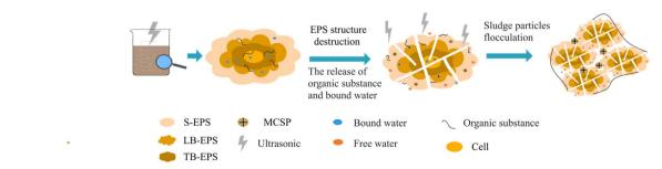
Fig. 8 Sludge dewatering mechanism.
