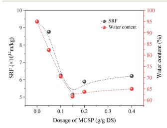
Fig. 3 Effect of MCSP dosage on sludge dewatering performance.
