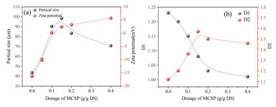
Fig. 6 Effects of MCSP combined with ultrasonic conditioning on sludge particle size, zeta potential, and fractal dimension (a) particle size and zeta potential; (b) fractal dimension.
